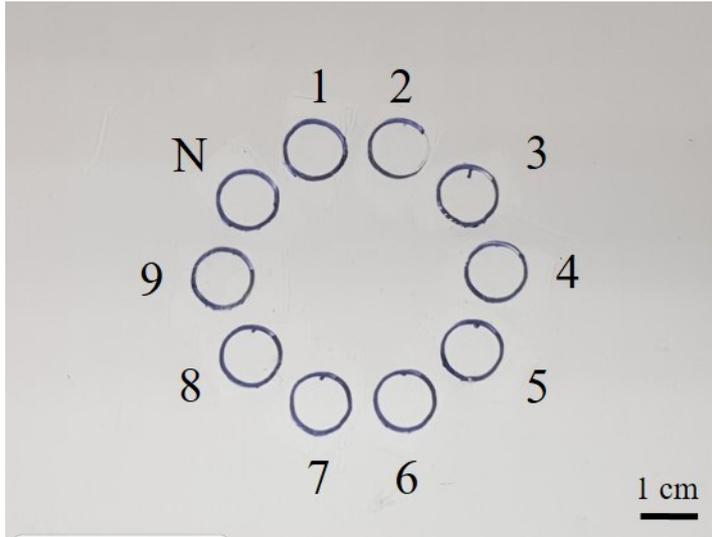
**Figure S3.** A circular glass array for spotting 6-mm tissue samples (either healthy or cancerous tissues could be applied). N=negative control region.
