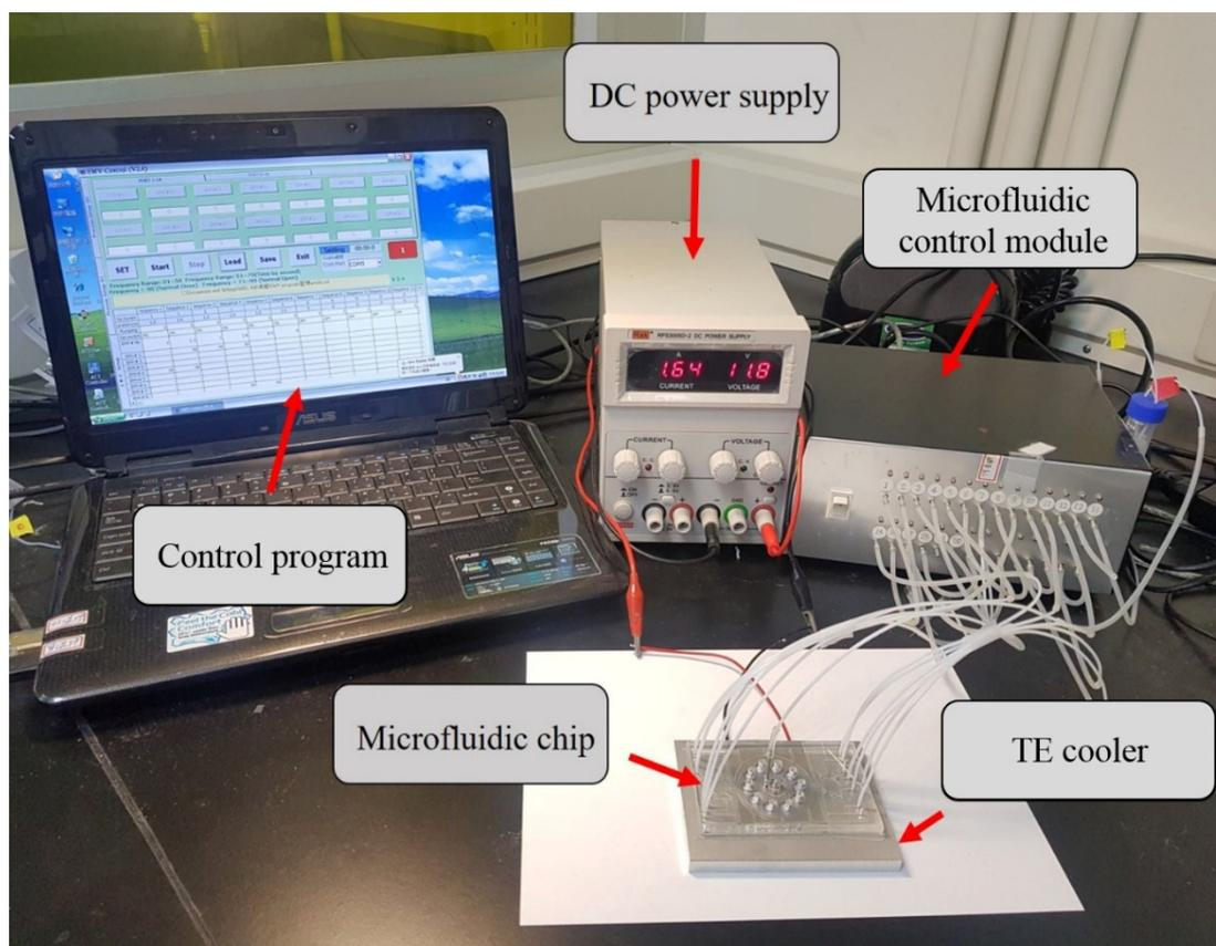
**Figure S2.** Experimental setup for on-chip clinical tissue staining. Upon integrating a thermoelectric (TE) cooler, a microfluidic control module, a DC power supply, and a computer, the entire protocol discussed in the main text could be automated.
