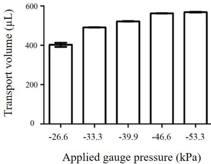
**Figure S4.** The relationship between the liquid transport volume and the applied (air) gauge pressure. Across 16 transport iterations, the variation in liquid volume transported remained low (error bars represent standard deviation).
