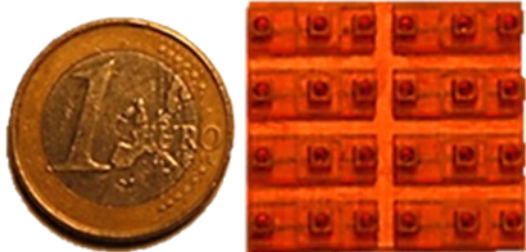
Fig. S4. An array of individual microfluidic droplet generators fabricated in a single stereolithographic printing procedure.
