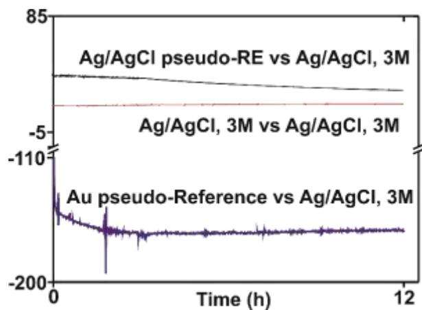
**Figure S6.** Potential profile recorded during the stability tests along 12 hours for the three compared reference electrodes. The top part of the plot has been magnified to show the variation of the Ag/AgCl pseudo-reference when compared with the commercial golden standard. Au pseudo-reference electrode showed higher potential variation than Ag/AgCl pseudo-reference and the golden standard.
