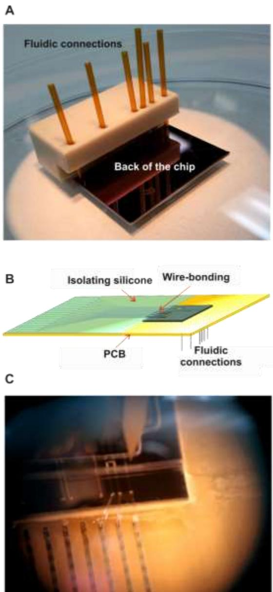
**Figure S2.** (A) Image of the bonding between the fluidic tubes and the rear fluid output of the silicon chip. (B) 3-D schematic view of the chip encapsulated in a PCB. (C) Image detailing the wire-bonding between the electrical pads of the chip and the electrical pads of the PCB.
