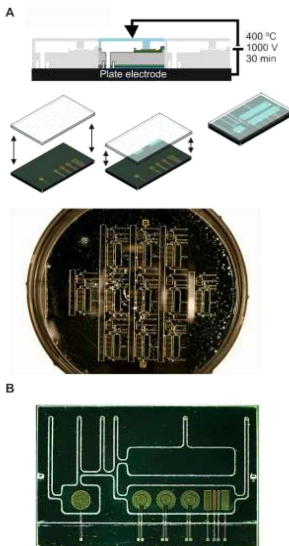
**Figure S1.** (A) Schematic images showing the anodic bonding between the wafer glass (containing the microfluidic cover) and the silicon chip (containing the electrodes) performed by applying temperature and electric field. Etched thickness of 0.35 mm. Bottom thickness of 0.15 mm. (B) Image of the individual chip after the dicing step of the bonded glass cover/silicon chip.
