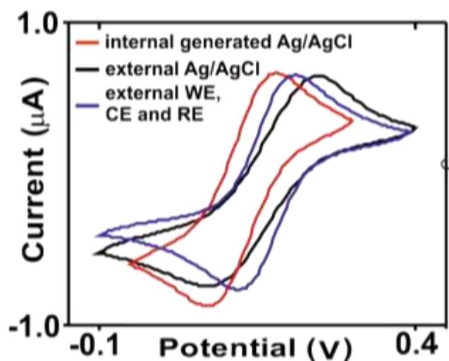
**Figure S7.** Cyclic voltammograms recorded in 0.1 M KCl 1mM potassium ferricyanide after the activation of the gold microelectrode positioned on the ME-LoC versus the Ag/AgCl pseudo-RE (red line) and an external double-junction Ag/AgCl RE (black line). The voltammogram recorded with an external gold microelectrode as WE is plotted using a blue line. The electrochemical cell in this last experiment was completed using a commercial Pt CE and a commercial Ag/AgCl RE.
