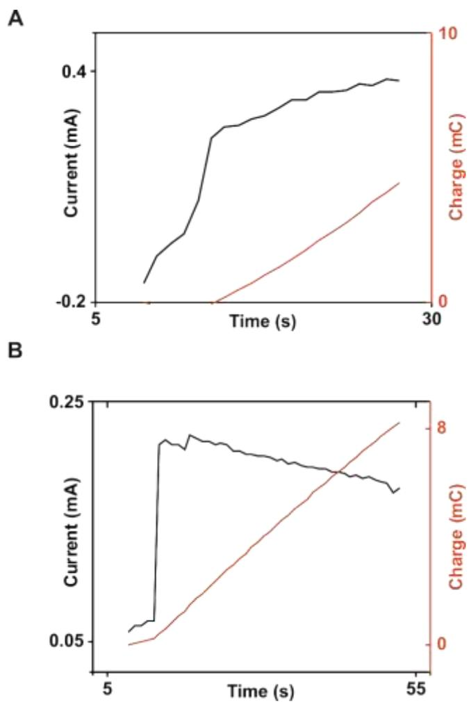
**Figure S5.** Current (black line) and accumulation charge (red line) profile recorded during the amperometric electrogeneration of the (A) PPy/ferrocyanide and (B) PPy/GOX membranes.
