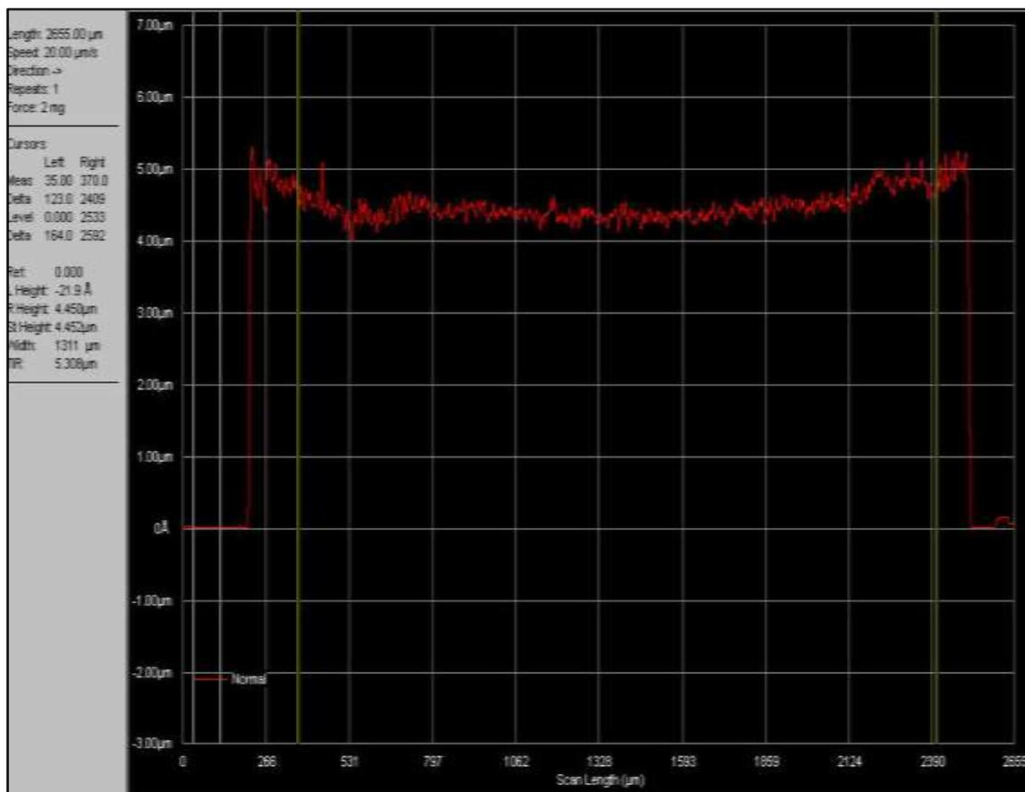
**Figure S3.** Result of the profilometry performed on the pseudo-reference electrode, once Ag and AgCl were deposited. As can be seen, the thickness of both layers is around 4  $\mu\text{m}$ , which fits with the theoretical calculations, since for the formation of the 1.3  $\mu\text{m}$  AgCl layer, part of the 4  $\mu\text{m}$  of Ag has been consumed
