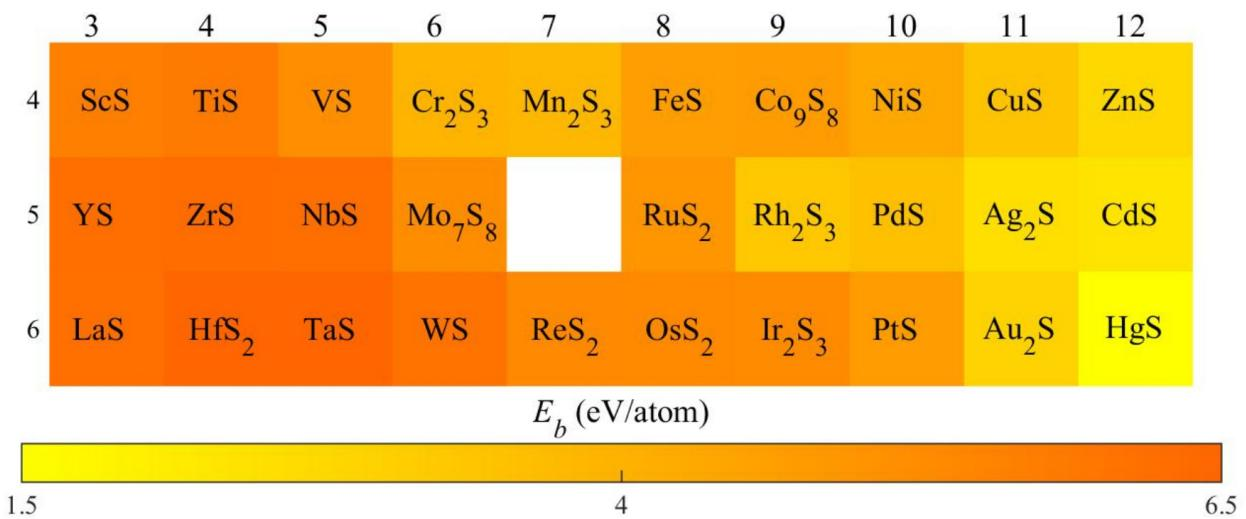
**Fig. S4** Binding energy for the TM-sulfides plotted in rows and columns of the periodic table. Orange means high binding energy, while yellow is for low binding energy.
