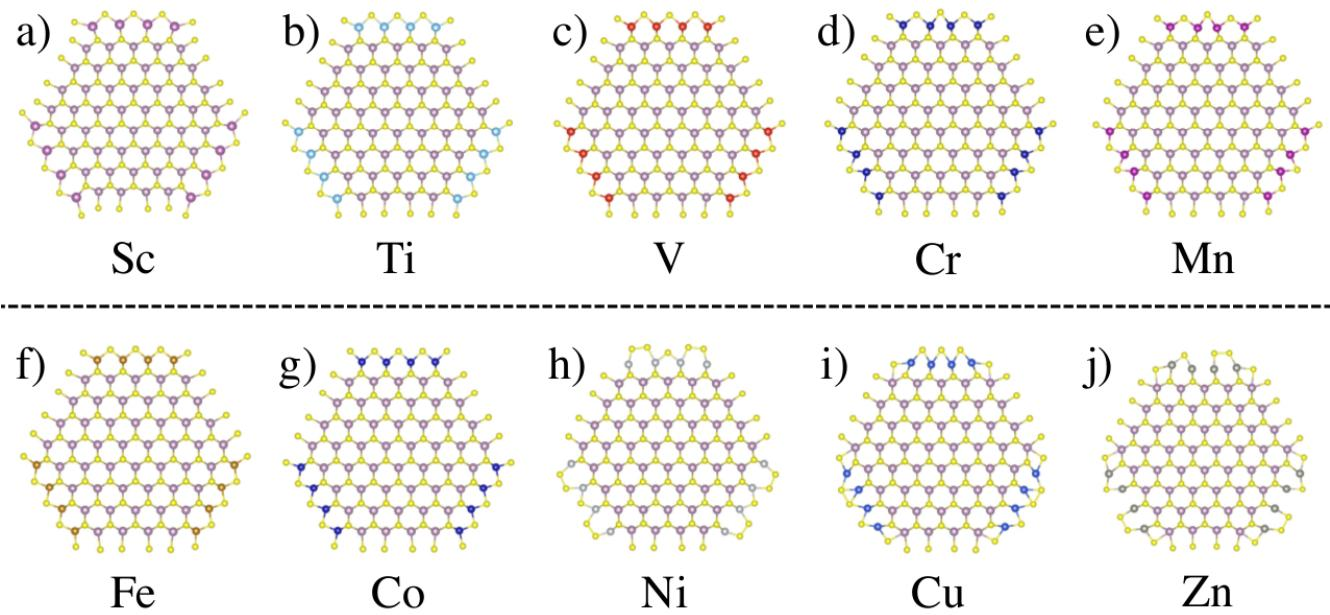
**Fig. S2** Geometrical structures of the relaxed TM-promoted  $\text{MoS}_2$  nanosheets with sulfur saturation, with the  $3d$  TM promoters; a) Sc, b) Ti, c) V, d) Cr, e) Mn, f) Fe, g) Co, h) Ni, i) Cu, and j) Zn.
