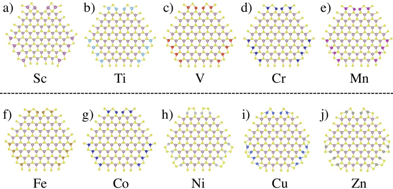
**Fig. S3** Geometrical structures of relaxed TM-promoted MoS<sub>2</sub> nanosheets with sulfur vacancy at the center of the edge (Vs@Cen), with the 3d TM promoters; a) Sc, b) Ti, c) V, d) Cr, e) Mn, f) Fe, g) Co, h) Ni, i) Cu, and j) Zn
