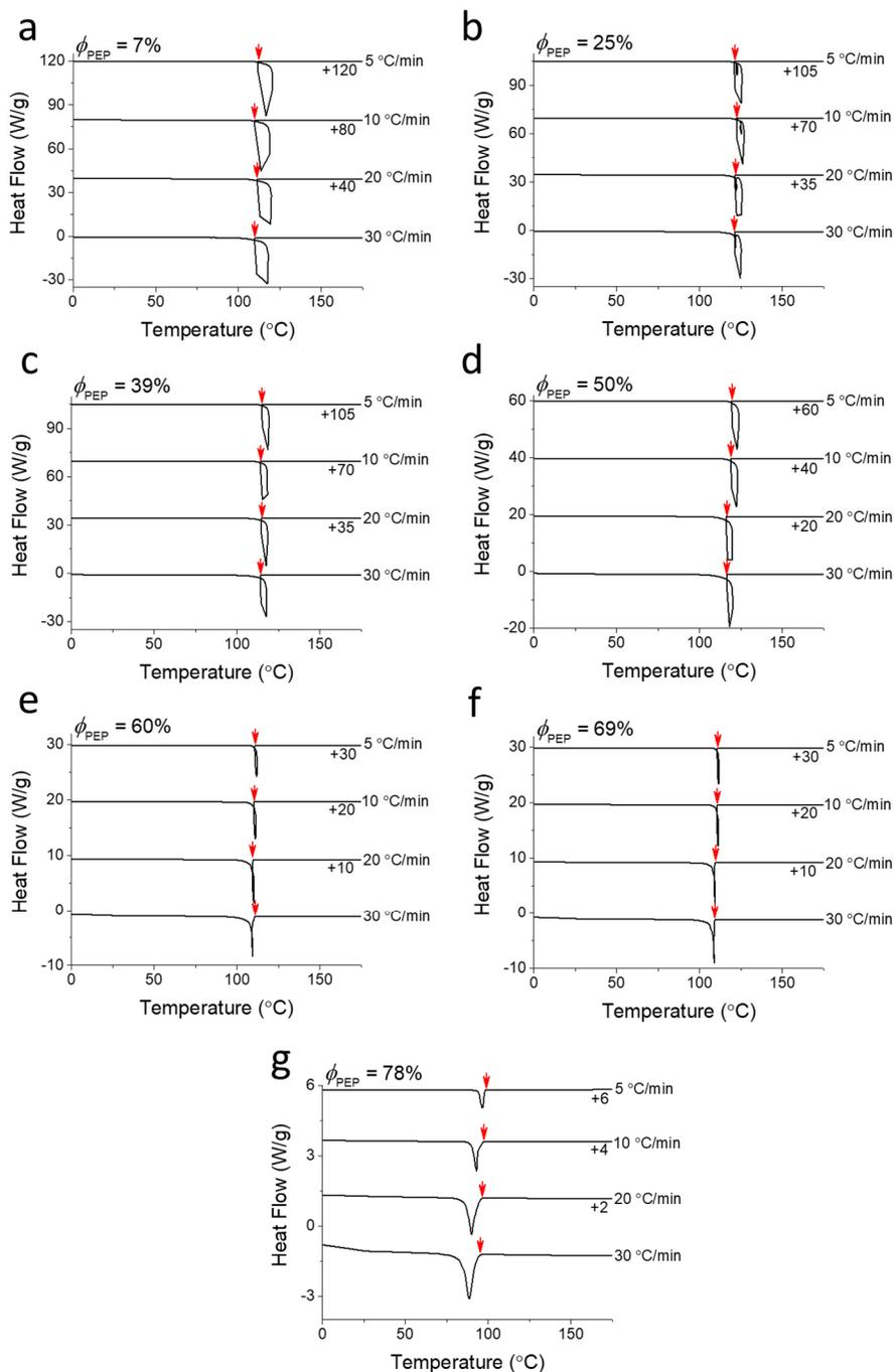
**Figure S3.** Cooling DSC thermograms of poly(ethylene-*alt*-propylene) (PEP,  $M_n = 25.5$  kg/mol) and pyrene mixtures at  $\phi_{\text{PEP}} =$  (a) 7 vol. %, (b) 25 vol. %, (c) 39 vol. %, (d) 50 vol. %, (e) 60 vol. %, (f) 69 vol. %, (g) 78 vol. % in endo-up forms. The commencement temperatures of crystallization are marked with red arrows. Thermograms are shifted for clear representations.
