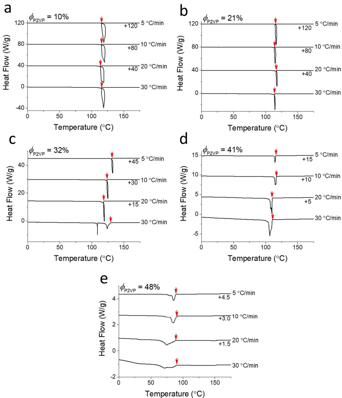
**Figure S4.** Cooling DSC thermograms of poly(2-vinylpyridine) (P2VP,  $M_n = 20.3$  kg/mol) and pyrene mixtures at  $\phi_{P2VP} =$  (a) 12 vol. %, (b) 23 vol. %, (c) 34 vol. %, (d) 45 vol. %, (e) 55 vol. % in endo-up forms. The commencement temperatures of crystallization are marked with red arrows. Thermograms are shifted for clear representations.
