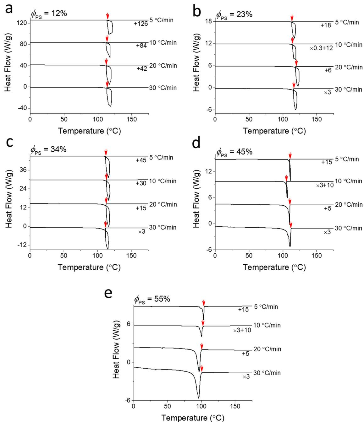
**Figure S2.** Cooling DSC thermograms of polystyrene (PS,  $M_n = 23.4$  kg/mol) and pyrene mixtures at  $\phi_{PS} =$  (a) 12 vol. %, (b) 23 vol. %, (c) 34 vol. %, (d) 45 vol. %, (e) 55 vol. % in endo-up forms. The commencement temperatures of crystallization are marked with red arrows. Thermograms are shifted for clear representations.
