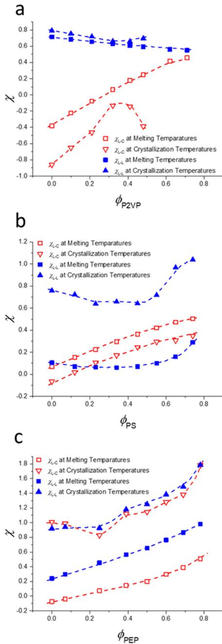
**Figure S5.** Effective interaction parameters of pyrene and (a) Poly(2-vinylpyridine), (b) Polystyrene, or (c) Poly(ethylene-*alt*-propylene) at the binodal and crystallization temperatures and compositions based on the parameters extracted from the melting and crystallization temperatures in Figure 6 of the main text. The effective interaction parameters extracted at different temperatures and by the different experimental methods are inconsistent with each other.
