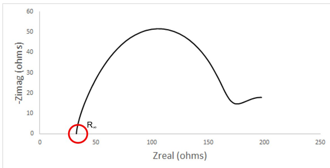
Fig. S4. Example of EIS results form a Li/Li symmetric cell as shown in Fig. S3 and R_\infty
