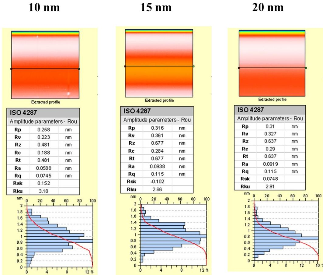
**Figure S4.** Roughness profiles of ALD processed Al<sub>2</sub>O<sub>3</sub> films with thicknesses ranging from 2 nm to 20 nm.
