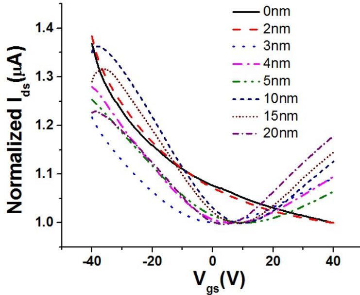
**Figure S5.** Semiconducting property of the FET sensor with an ALD Al<sub>2</sub>O<sub>3</sub> film of various thicknesses.
