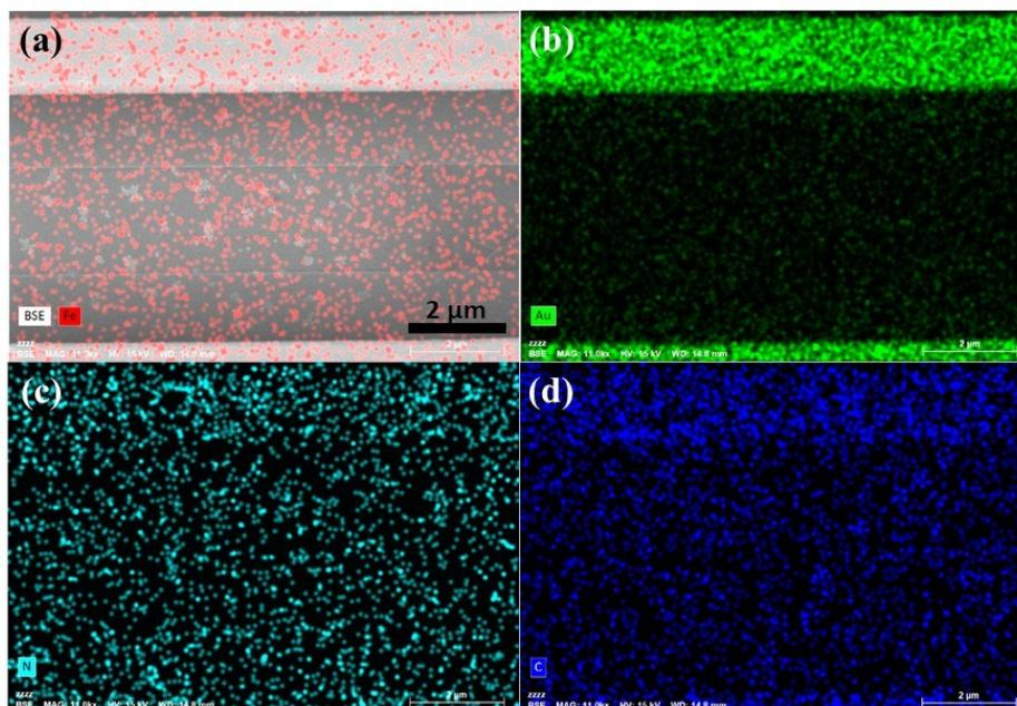
Figure S1. EDS mapping of a) Iron, b) Gold, c) Nitrogen, d) Carbon elements on the sensor surface.
