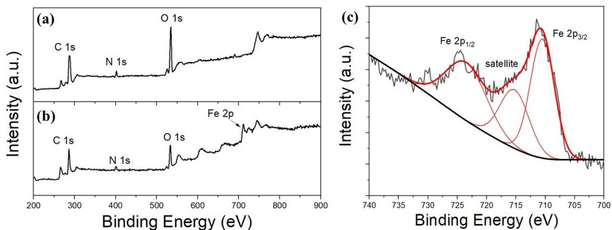
Figure S2. XPS spectra of the (a) as-prepared sample and (b) sample treated in Ar plasma. (c) High resolution XPS spectra of the Fe 2p level. The spectrum acquired before the etching process (a) indicates typical peaks for C 1s, N 1s and O 1s core levels. After plasma treatment (b), the Fe inside the ferritin was exposed. The visible emissions from Fe 2p<sub>3/2</sub> (710.5 eV), Fe 2p<sub>3/2</sub> (715.3 eV), and Fe 2p<sub>1/2</sub> (723.5 eV) are more evident.
