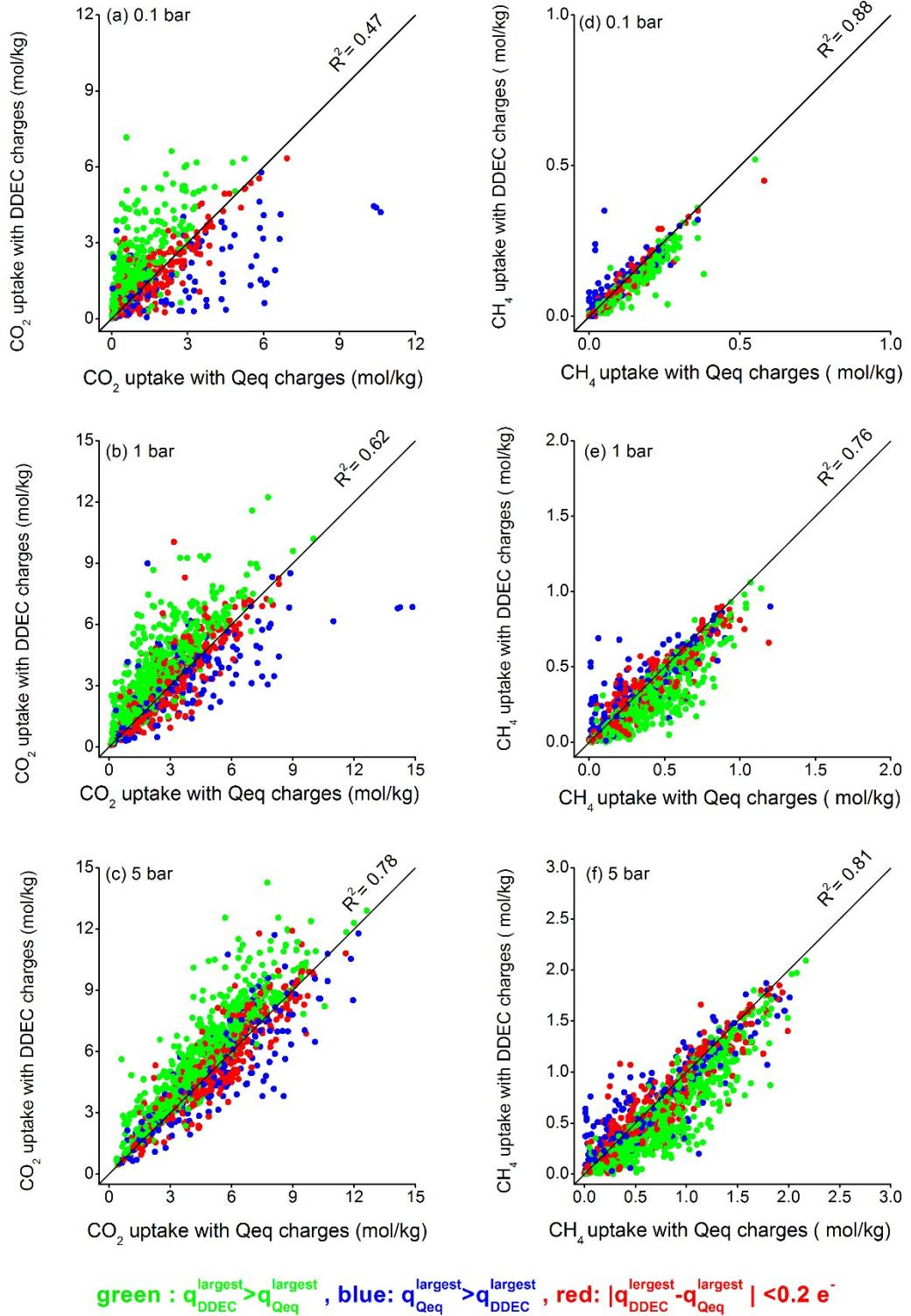
**Figure S3.**  $\text{CO}_2$  uptakes (a-c) and  $\text{CH}_4$  uptakes (d-f) obtained from simulations using Qeq and DDEC charges at 0.1, 1, 5 bar for  $\text{CO}_2/\text{CH}_4$ : 50/50 mixture.
