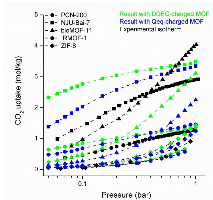
**Figure S2.** Comparison of  $\text{CO}_2$  adsorption isotherms obtained for DDEC-charged and Qeq-charged MOFs at 298 K.
