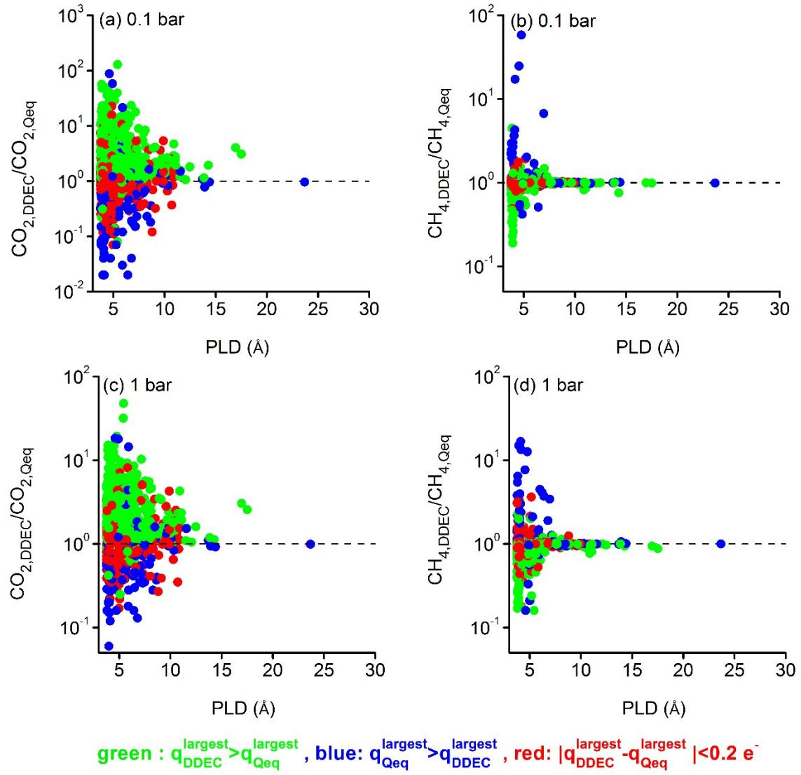
**Figure S8.** The ratio of (a, c)  $\text{CO}_2$  uptakes (b, d)  $\text{CH}_4$  uptakes computed by DDEC-charged to the ones computed by Qeq-charged MOFs as a function of PLD.
