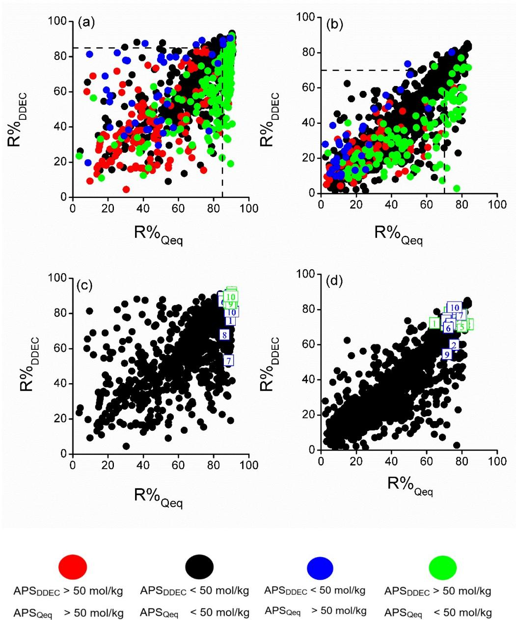
**Figure S7.** Comparison of R% of DDEC and Qeq-charged MOFs at (a, c) VSA (b, d) PSA conditions for  $\text{CO}_2/\text{CH}_4$ : 50/50 mixture. Dashed lines show  $R\% = 85\%$  in (a),  $R\% = 70\%$  in (b). The top 10 MOFs identified by DDEC and Qeq methods are shown with green and blue, respectively.
