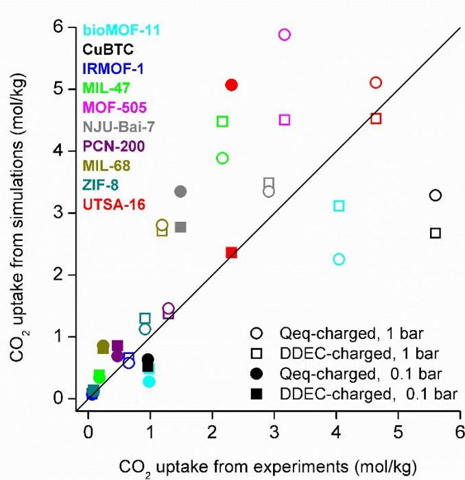
**Figure S1.** Comparison of the experimental  $\text{CO}_2$  uptakes<sup>1-7</sup> with our simulation results obtained using different charge assignment methods. Squares (circles) represent the simulation results of DDEC (Qeq)-charged MOFs while filled (empty) symbols are the results for 0.1 (1) bar.
