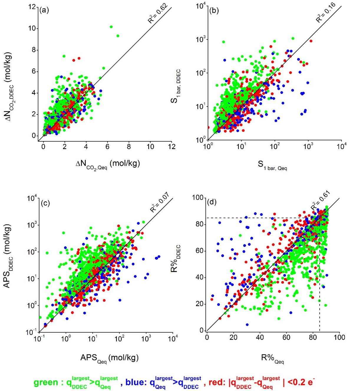
**Figure S5.** Calculated adsorbent performance evaluation metrics using Qeq and DDEC charges at VSA condition, 298 K for CO<sub>2</sub>/CH<sub>4</sub>:50/50 mixture; (a)  $\Delta N_{CO_2}$ , (b)  $S_{ads}$ , (c) APS, (d) R%. Dashed lines in (d) show R% = 85%.
