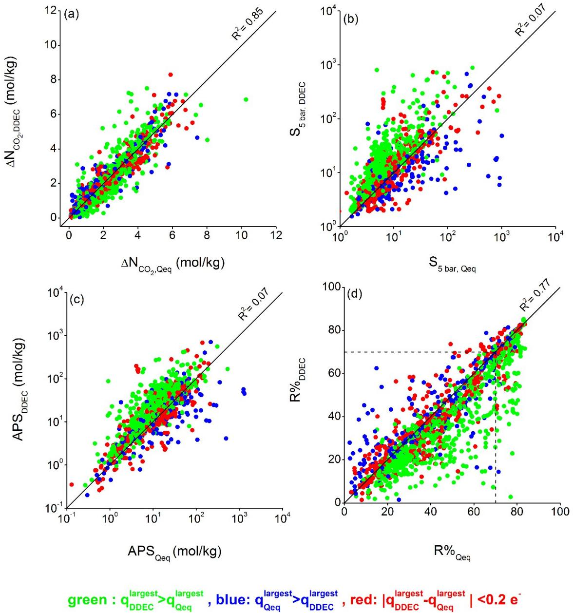
**Figure S6.** Calculated adsorbent performance evaluation metrics using Qeq and DDEC charges at PSA condition, 298 K for CO<sub>2</sub>/CH<sub>4</sub>:50/50 mixture; (a)  $\Delta N_{CO_2}$ , (b)  $S_{ads}$ , (c) APS, (d) R%. Dashed lines in (d) show R% =70%.
