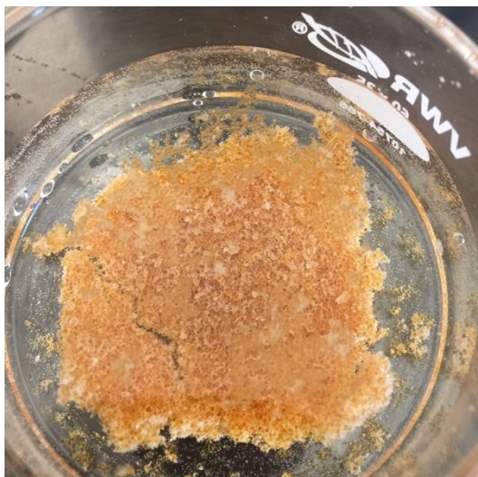
Figure S2. CEI-CER RW synthesized without adding polyethylene to the mixture. This RW shows poor mechanical integrity after immersion in water due to chemical incompatibility between the SPEEK CEI and CER.
