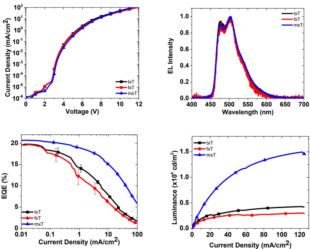
Fig. S18. OLED device characteristics of phenanthro[9,10-*d*]triazoles
