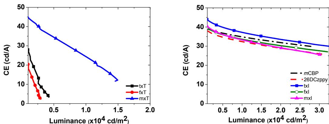
Fig. S19. Current Efficiency plot of phenanthro[9,10-*d*]triazoles and phenanthro[9,10-*d*]imidazoles
