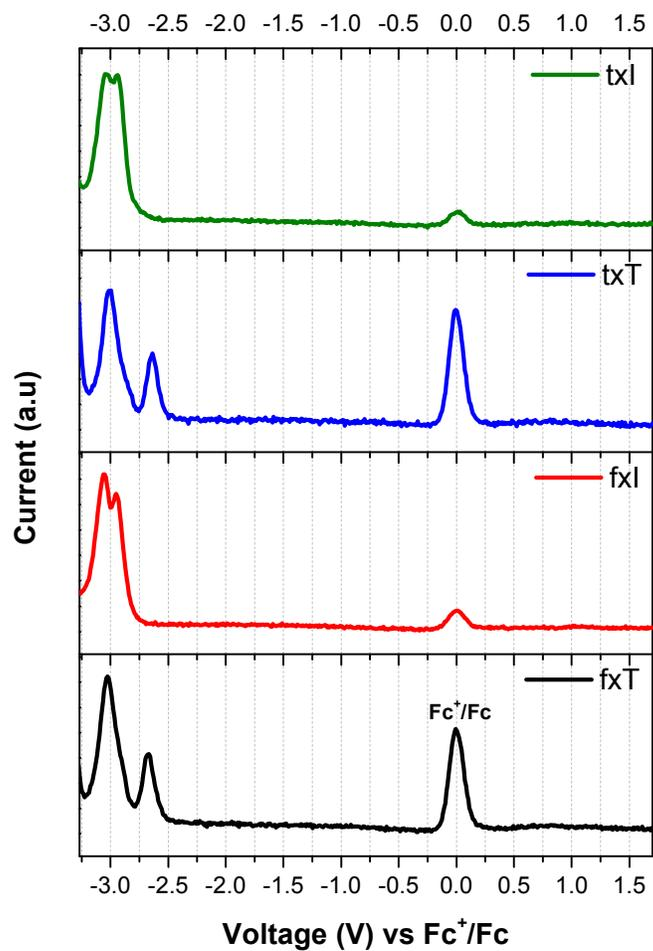
Fig. S13. DPV data of selected phenanthro[9,10-*d*]triazoles/imidazoles
