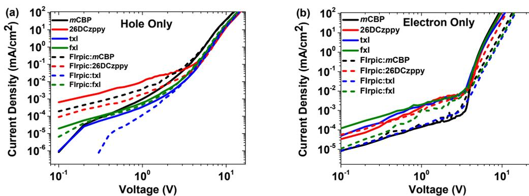
**Fig. S20.** (a) Hole only Structure: 20 min UV Ozone 70 nm ITO / 5 nm HATCN / 20 nm TAPC / 10 nm mCP / 20 nm 8vol% Firpic:host or neat host / 10 nm HATCN / 100 nm Al. (b) Electron only Structure: no UV Ozone 70 nm ITO / 30 nm BP4mPy / 20 nm 8 vol% Firpic:host or neat host / 30 nm BP4mPy / 1.5 nm LiQ / 100 nm Al
