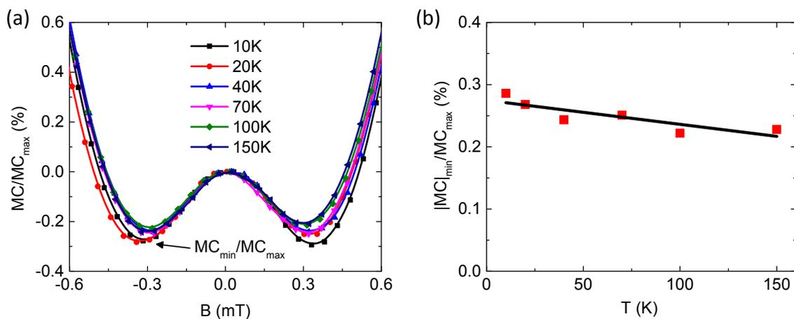
**Figure S7.** MC response of a pristine OLED at the ultra-small magnetic field. (a) Normalized MC response at the ultra-small magnetic field with temperature dependence. (b)  $|MC|_{\min}/MC_{\max}$  at different temperatures, where the data points (red square) is linearly fitted (black line).
