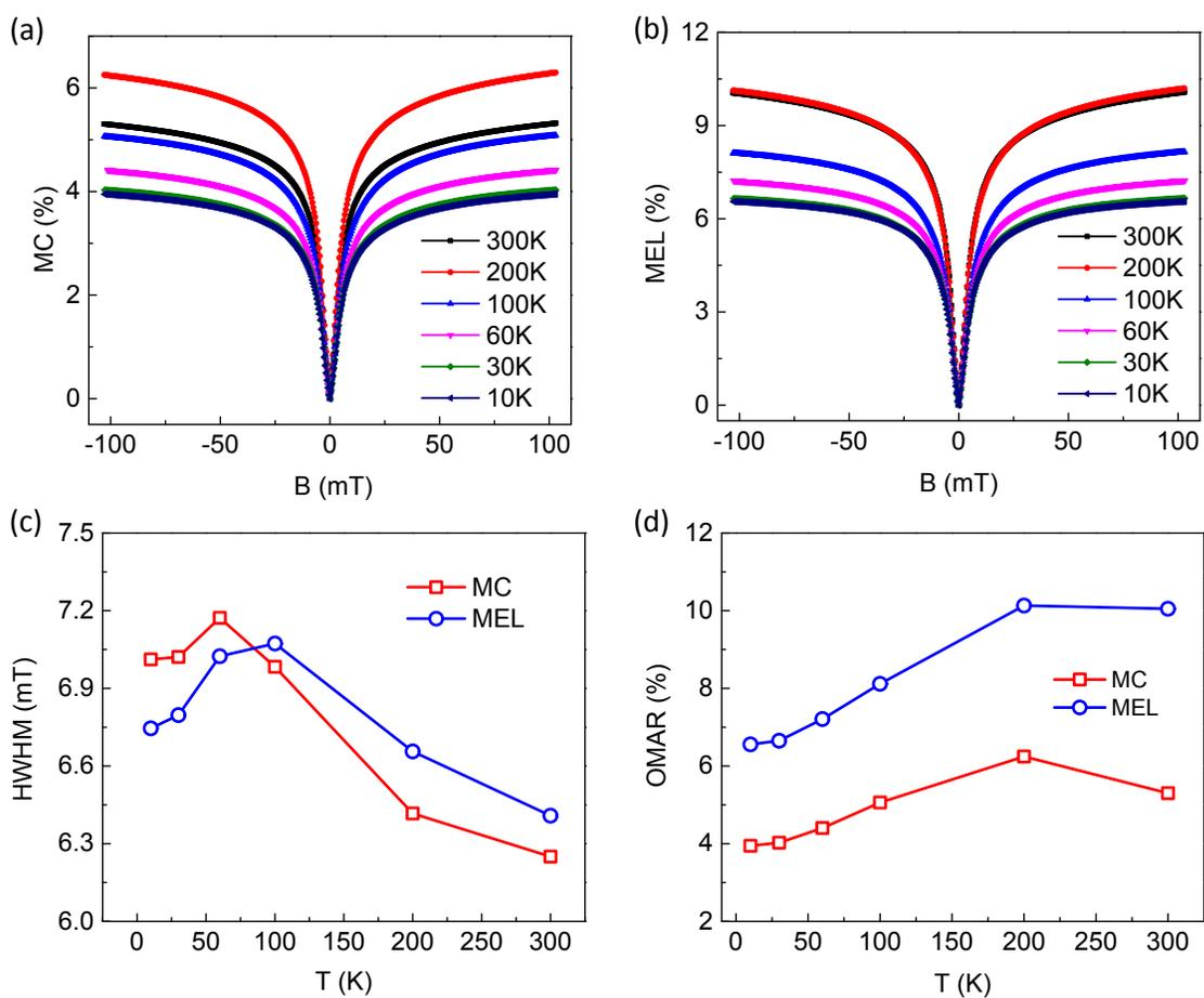
**Figure S5.** Magnetic field effect of the pristine OLED at different temperatures. (a) MC responses and (b) MEL responses with temperature dependence. (c) Half-width of half maximum (HWHM) and (d) the magnitude of MC and MEL responses with temperature dependence.
