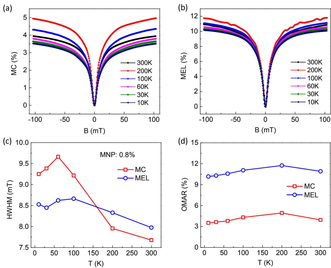
**Figure S4.** Magnetic field effect of the blend OLED with 0.8% MNP at different temperatures. (a) MC responses and (b) MEL responses with temperature dependence. (c) Half-width of half maximum (HWHM) and (d) the magnitude of MC and MEL responses with temperature dependence.
