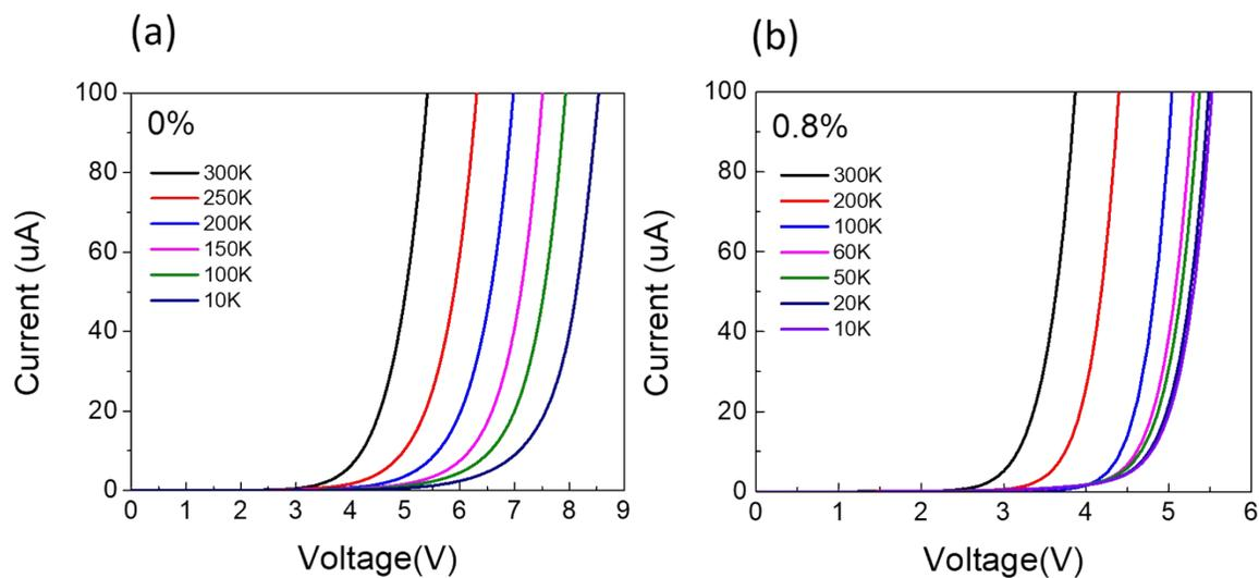
**Figure S6.** Typical temperature dependence of current density in (a) pristine and (b) 0.8% MNP based OLEDs.
