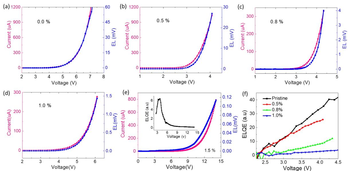
**Figure S1.** The current-voltage (IV) and EL-V characteristics of the devices with (a) 0.0 %, (b) 0.5 %, (c) 0.8 %, (d) 1.0 %, and (e) 1.5% MNP concentration at room temperature, (f) Electroluminescence quantum efficiency (ELQE defined by  $EL/I$ ) versus applied voltage. The data was processed from parts a-d. The ELQE of 1.5% MNP device is plotted in the inset of (e).
