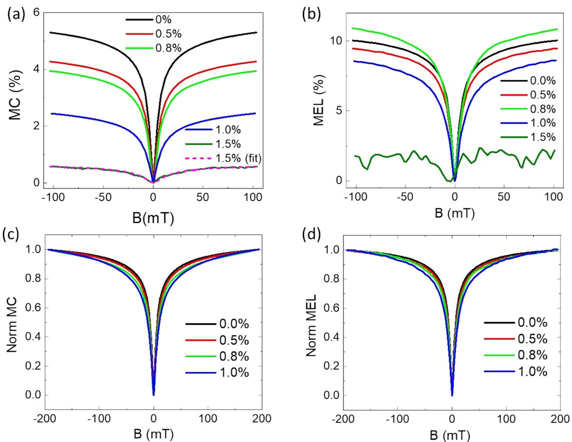
**Figure S2.** Magnetic field effect of the OLEDs with different concentrations of MNPs at 300 K. (a) MC response and (b) MEL response with the concentration dependence with magnetic field range of 100 mT. Normalized (c) MC and (d) MEL with magnetic field range of 200 mT.
