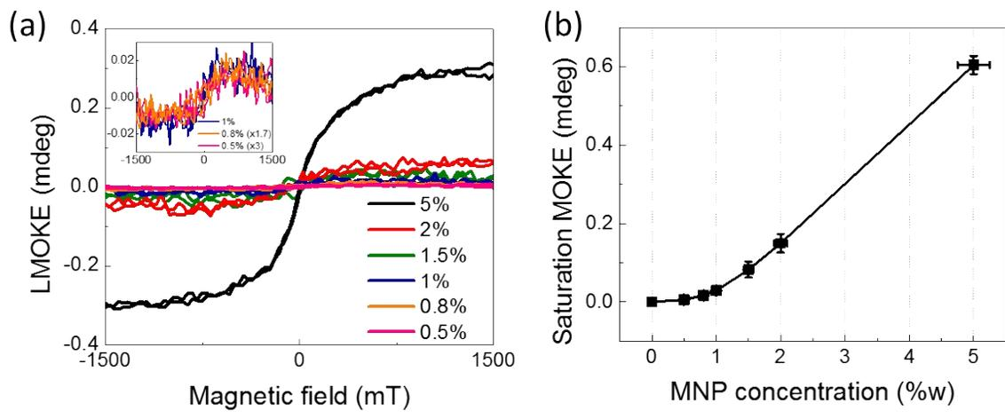
**Figure S3.** (a) MOKE hysteresis curve of SU8/MNP thin film with different concentration of MNPs. Inset: zoom-in of MOKE hysteresis curve with low concentration of MNP of 1% and 0.5%. (b) Saturation MOKE signal versus concentration of MNPs (%w) with error bars.
