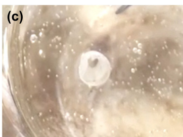
(c) If wax is too hot ( T \gg T_m ) or if incubation time in hot wax > 30s , initial wax shell starts to melt
