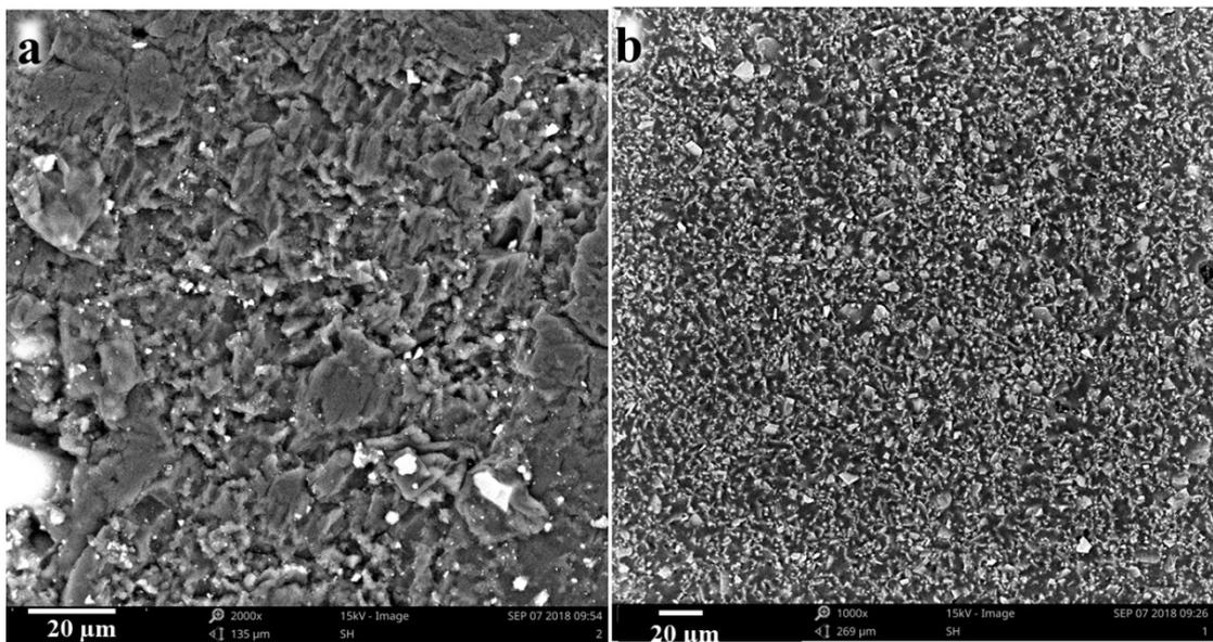
**Figure S10** SEM of epoxy-insulation board (a) and epoxy-heat insulation board (b).
