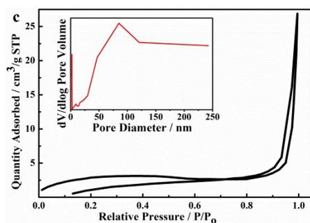
**Figure S3** N<sub>2</sub> adsorption-desorption isotherms and pore distribution (inset) of relevant (a) EP, (b) SEP and (c) PEP.
