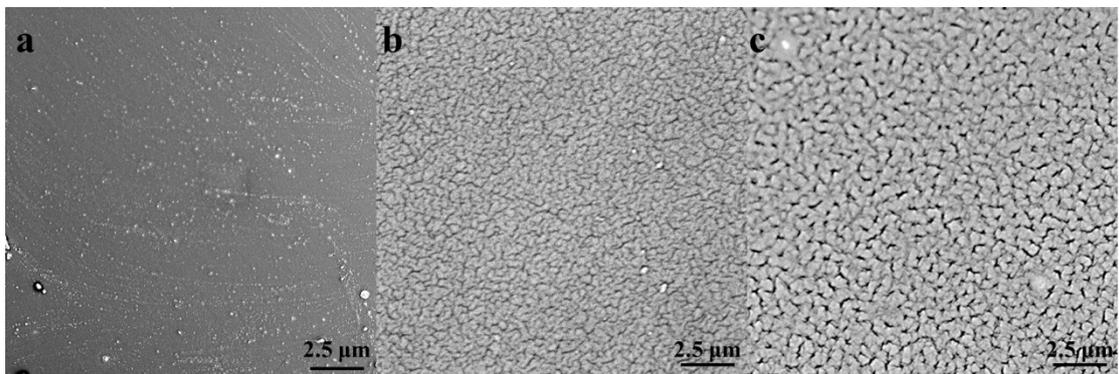
**Figure S2.** The SEM of cross section of EP (a), SEP (b) and PEP (c).
