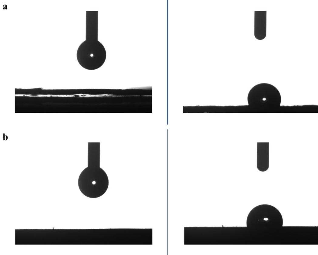
**Figure S9** Water contact angle of epoxy-insulation board (a) and epoxy-heat insulation board (b) were modified by NMP under microwave radiation at 150°C for 30 min. During the water CA measurement, the water droplet was 3  $\mu$ L.
