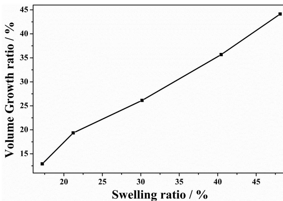
**Figure S7.** The swelling ratio versus volume growth ratio of SEP.
