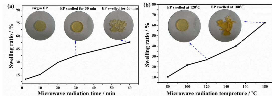
**Figure S1.** The effect of microwave conditions on the swelling of EP: a) microwave time (microwave temperature is 150°C, and microwave power is 400 W); b) microwave temperature (microwave time is 30 min, and microwave power is 400 W). The embedded graph is optical pictures of EP during the swelling. The swelling ratio (r) of EP was calculated as follows:
