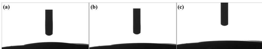
**Figure S4.** Wettability toward oil of the (a) EP, (b) SEP, (c) FEP. During the oil CA measurement, the chloroform droplet was 3  $\mu$ L.
