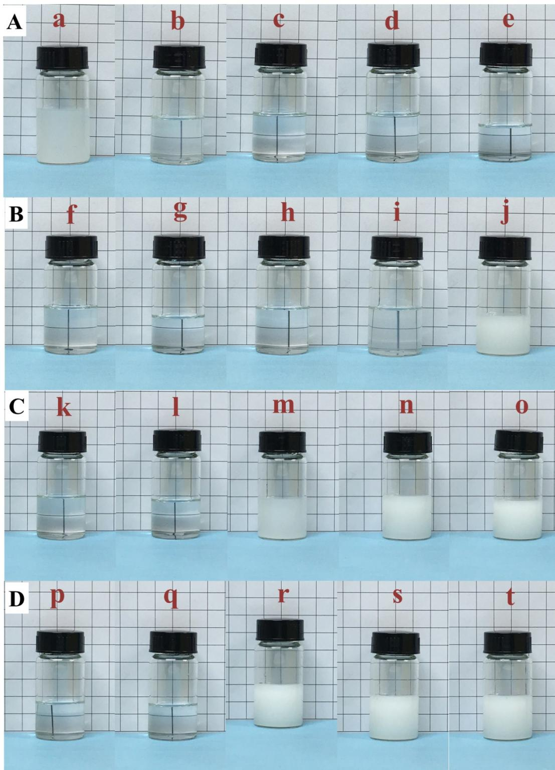
**Figure S8.** The optical images of the effect of PEP with different pore sizes (from A to D, 80 nm, 360 nm, 550 nm and 1.5 μm respectively) on separation of emulsion with different droplet sizes (from left to right, 20 μm, 6 μm, 550 nm, 300 nm, and 150 nm respectively).
