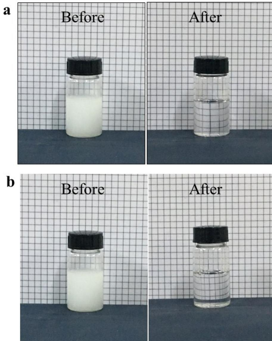
**Figure S11** Photos of oil/water emulsion with an average droplet size of  $3.50\ \mu\text{m}$  before and after separation by modified epoxy-insulation board (a) and epoxy-heat insulation board (b).
