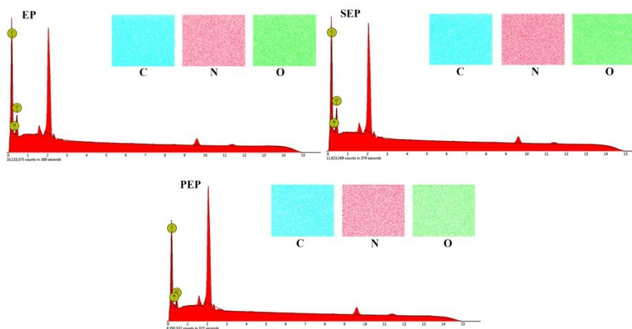
**Figure S6.** The EDX spectra and C, N, O mapping of EP, SEP and PEP.
