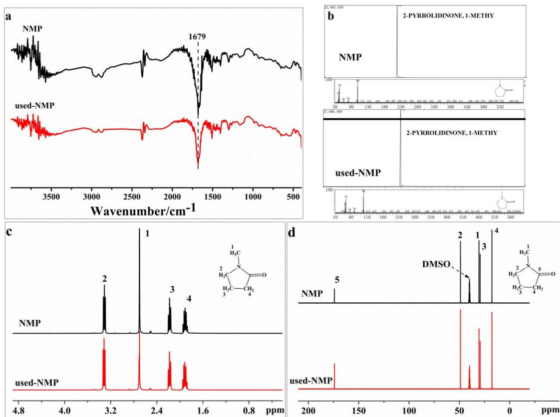
**Figure S5.** FT-IR spectra (a), GC-MS chromatogram (b), <sup>1</sup>H-NMR spectra (c), <sup>13</sup>C-NMR spectra (d) of virgin NMP and used NMP.
