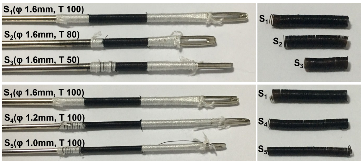
Fig. S2 Photos of hair springs. Hair springs with different turns and different diameters: S1 (φ1.6 mm, T100), S2 (φ1.6 mm, T80), S3 (φ1.6 mm, T50), S4 (φ1.2 mm, T100) and S5 (φ1.0
