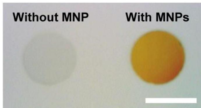
**Figure S1.** Image of free-standing albumin films with and without MNPs. Scale bar: 3 mm.
