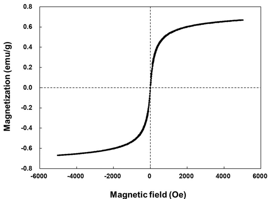
**Figure S2.** Magnetic hysteresis curve of albumin film containing MNPs.
