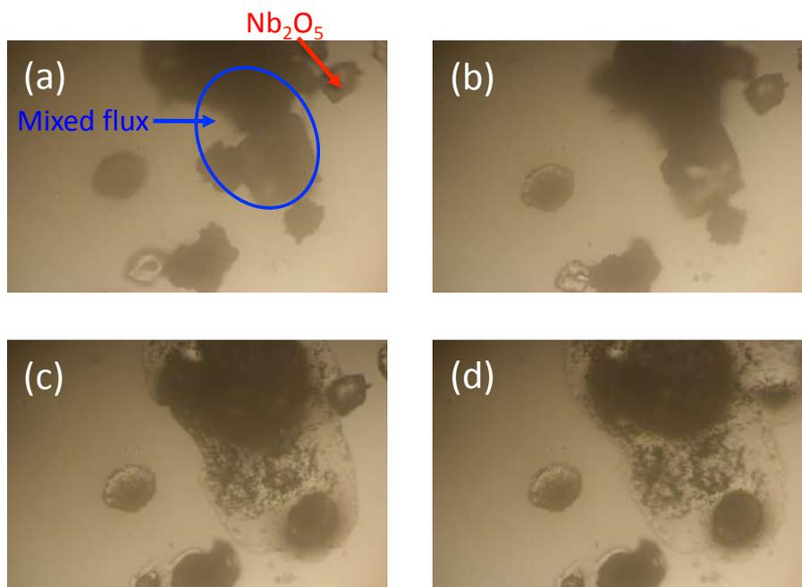
**Fig. S6** Optical micrographs of the mixed chloride flux and the solutes: (a) at 20 °C, (b) at 500 °C for 0 min., (c) at 500 °C for 5 min., and (d) at 500 °C for 10 min.
