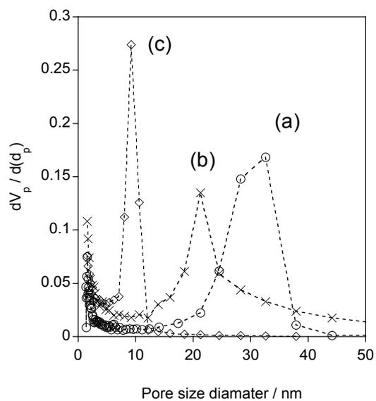
**Fig. S2** Pore size distributions of SBA-15 (33) (a), (21) (b), and (9) (c), evaluated by the BJH method.
