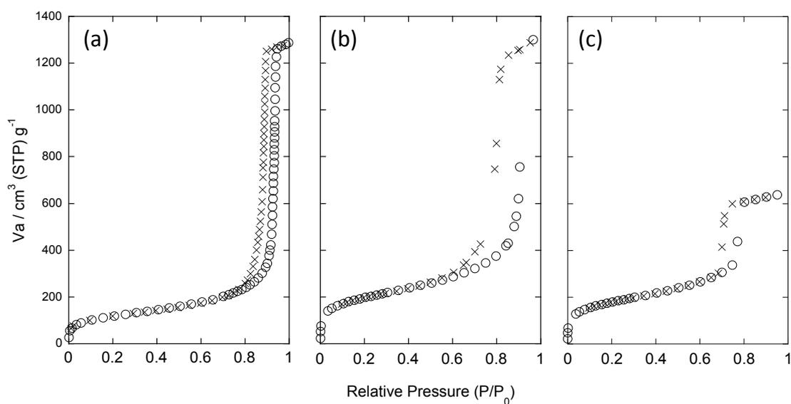
**Fig. S1** Nitrogen adsorption/desorption isotherms of SBA-15 (33) (a), (21) (b), and (9) (c).
