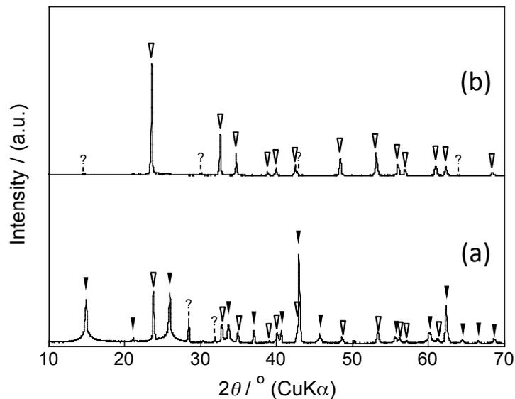
**Fig. S5** XRD patterns of the products synthesized without SBA-15;  $\text{Nb}_2\text{O}_5:\text{Li}_2\text{CO}_3 = 1 : 3$  (a) and  $= 3 : 1$  (b). The marks white and black correspond to  $\text{LiNbO}_3$  and  $\text{Li}_3\text{NbO}_4$ , respectively.
