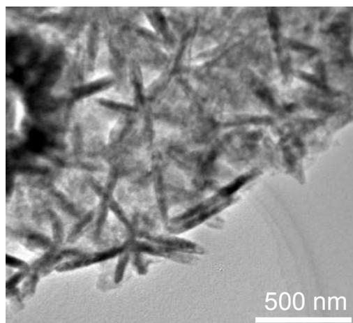
**Fig. S3** FE-TEM image of the product synthesized in the presence of SBA-15(21).
