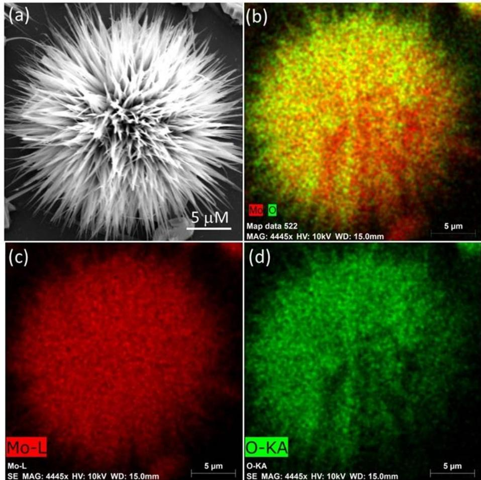
**Figure S3.** (a) FESEM image of MoO<sub>3</sub> sea urchin (b) combined EDS map of Mo L level and O K level (c) Corresponding EDS mapping of Mo L and (d) O K level.
