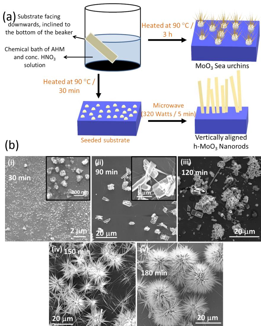
**Figure S1.** (a) Schematic of synthesis of MoO<sub>3</sub> sea urchins and h-MoO<sub>3</sub> nanorods employing chemical bath deposition and microwave methods, respectively. (b) FESEM images of MoO<sub>3</sub> sea urchin growth at various reaction stages from 30 to 180 minutes.
