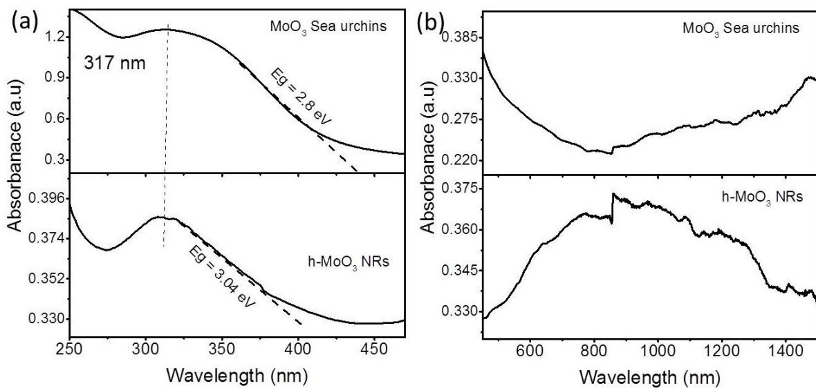
**Figure S6.** (a) UV-visible-NIR absorption spectra of as-synthesized  $\text{MoO}_3$  nanostructures such as  $\text{MoO}_3$  sea urchins and vertically aligned h- $\text{MoO}_3$  nanorods (b) Zoomed view of absorption spectra in (a).
