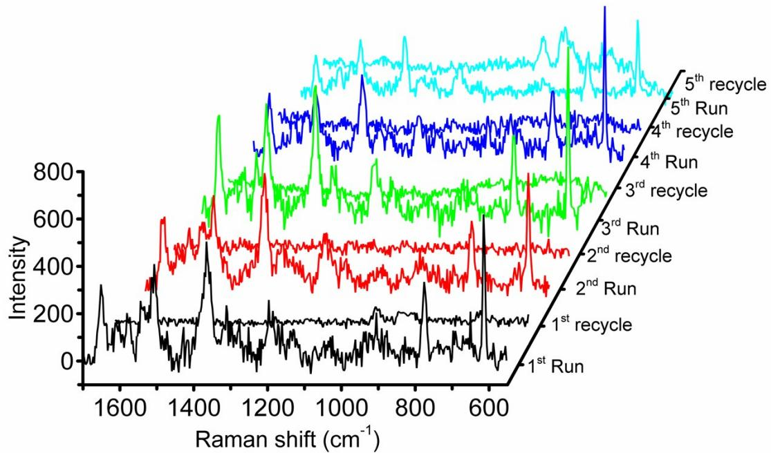
**Figure S13.** Reusable vertically aligned h-MoO<sub>3</sub> nanorods as SERS substrates; SERS of 100  $\mu\text{M}$  R6G before and after UV treatment.
