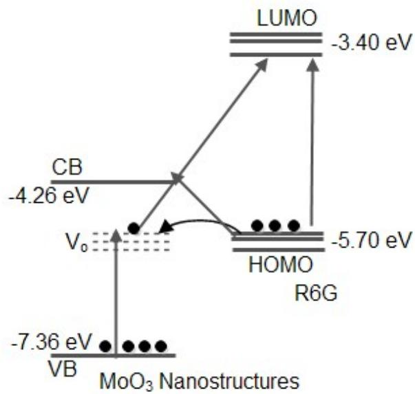
**Figure S11.** Schematic representation of charge transfer between the MoO<sub>3</sub> nanostructures and R6G molecules during the excitation with 532 nm laser light.
