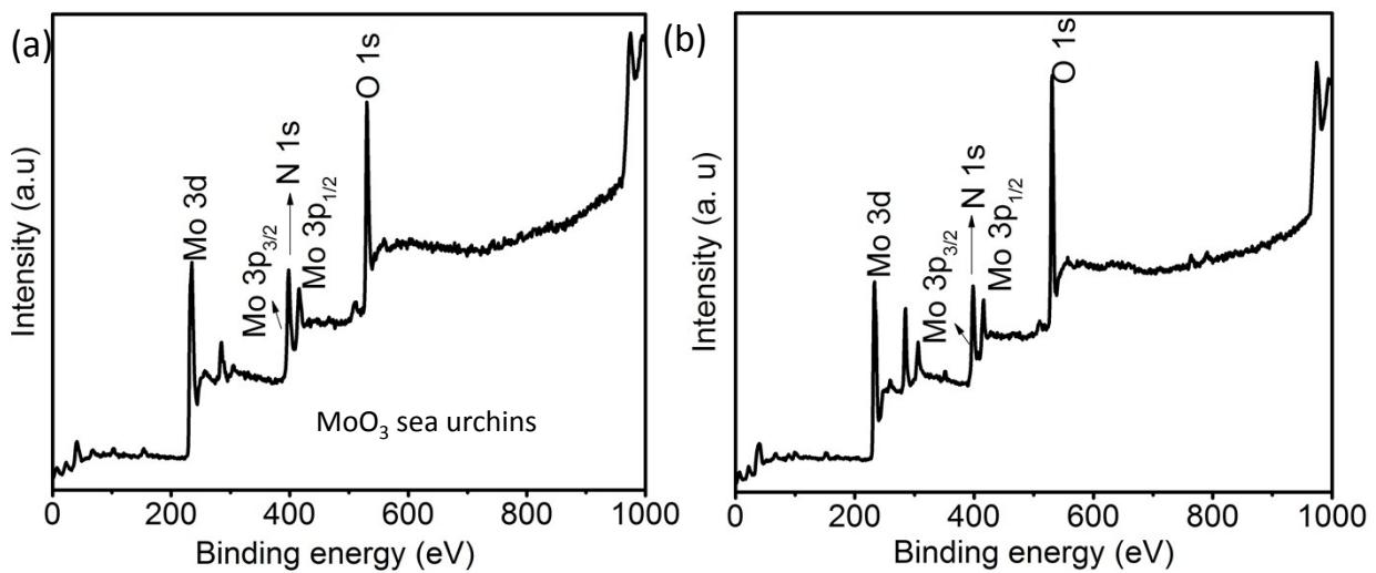
**Figure S7.** XPS Survey spectra of  $\text{MoO}_3$  nanostructures (a)  $\text{MoO}_3$  sea urchins (b) h- $\text{MoO}_3$  nanorods.
