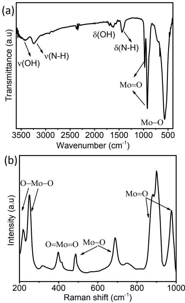
**Figure S5.** (a) FTIR spectra (b) Raman spectra of vertically aligned  $\text{MoO}_3$  nanorods.
