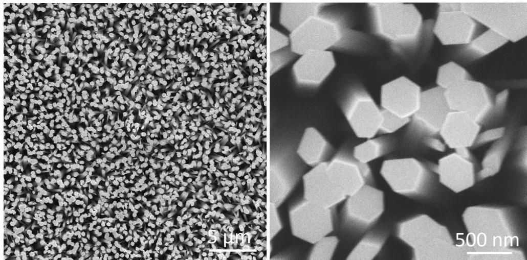
**Figure S4.** FESEM images of vertically aligned h-MoO<sub>3</sub> nanorods grown on Si substrate employing microwave method (a) low magnification image (b) high magnification image
