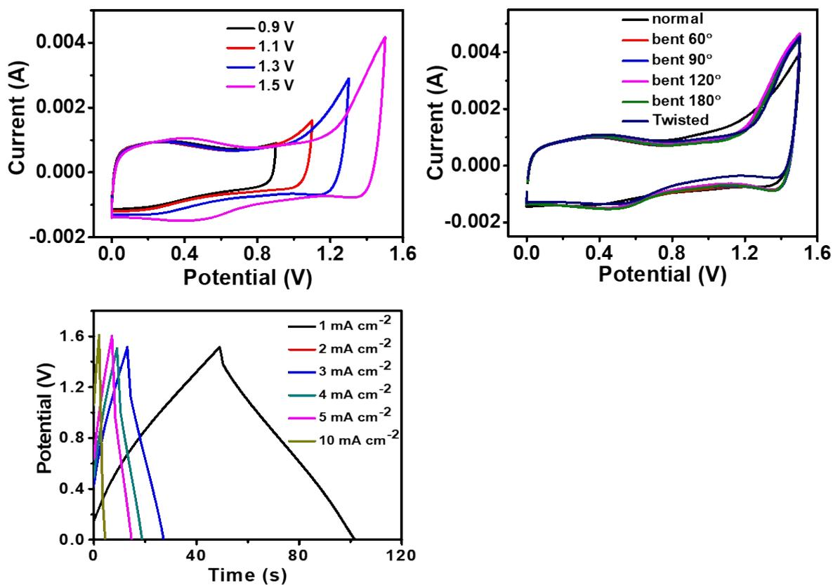
Fig. S2 (a) CV curves for NVL@CC//AC HSC at a scan rate of 10 mV s<sup>-1</sup> at different potential
