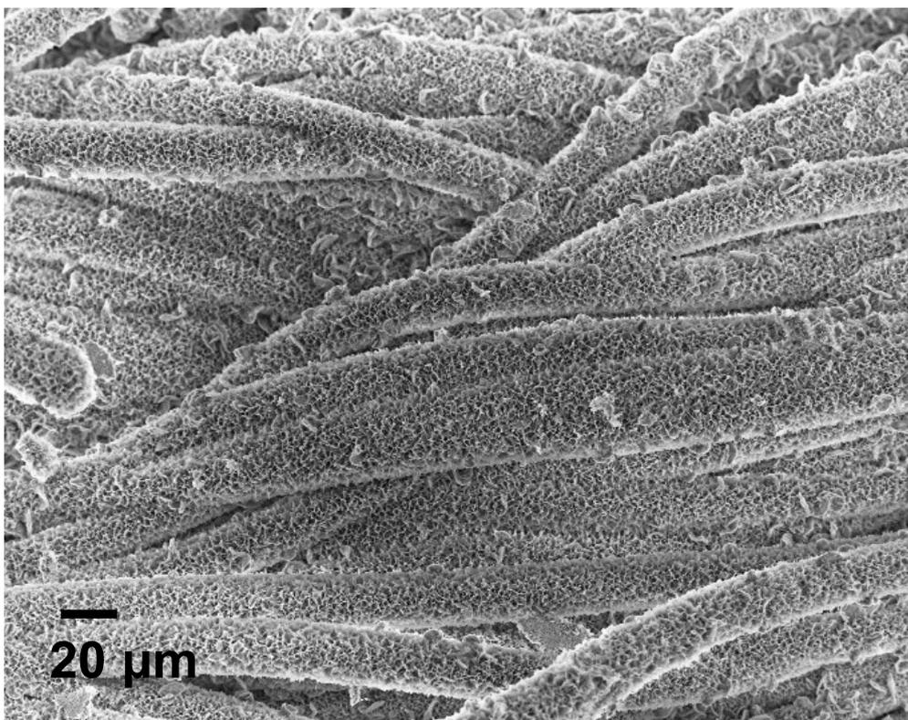
Fig. S1 Low magnification FESEM image for NVL@CC.
