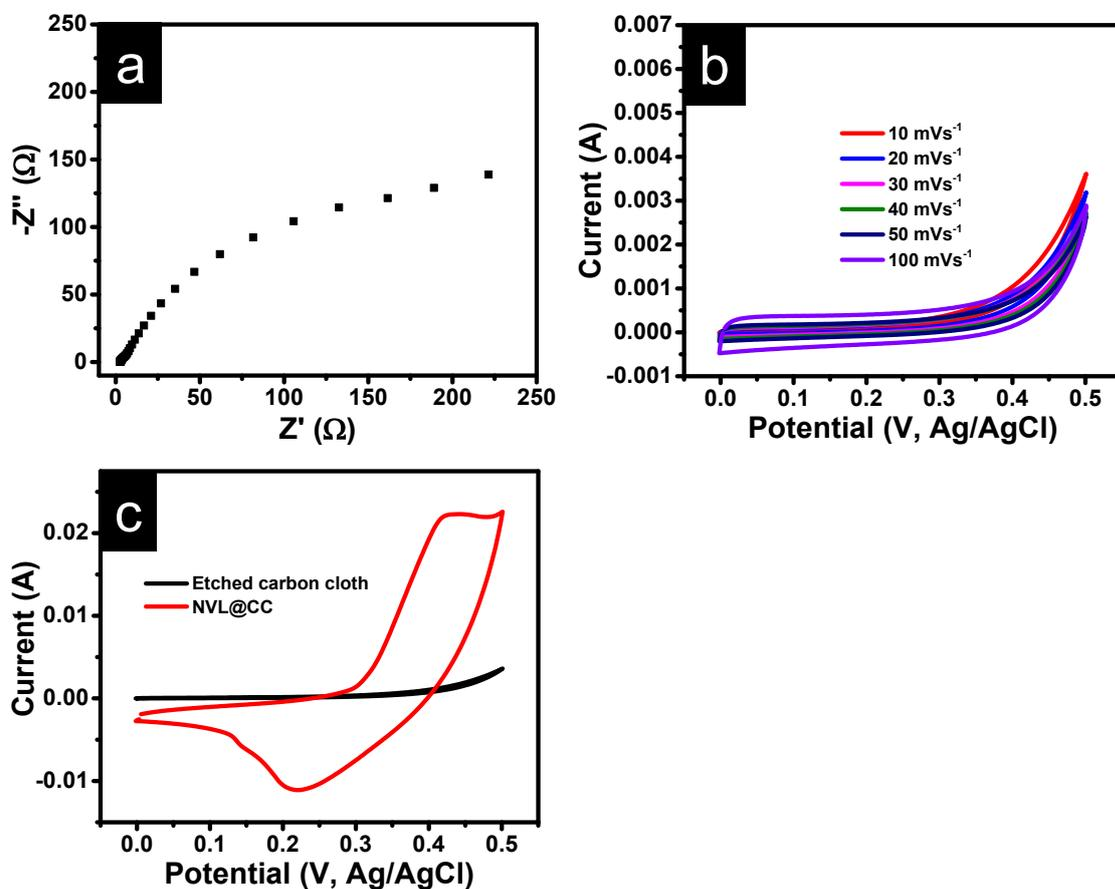
**Fig. S4** (a) EIS spectra for etched carbon cloth; (b) CV curves for etched carbon cloth at various scan rates; (c) Comparison of NVL@CC and etched carbon cloth CV curve at 10  $\text{mV s}^{-1}$  scan rate.
