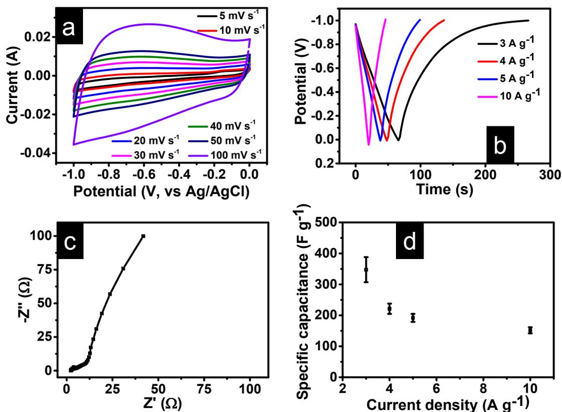
**Fig. S3** (a) CV curves for activated carbon coated carbon cloth at various scan rates; (b) GCD curves for activated carbon coated carbon cloth at various current densities; (c) EIS spectra for
