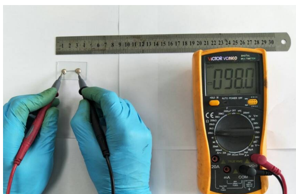
Figure S13. The photograph shows the electrical conductivity of a CNBs/TPU fiber.
