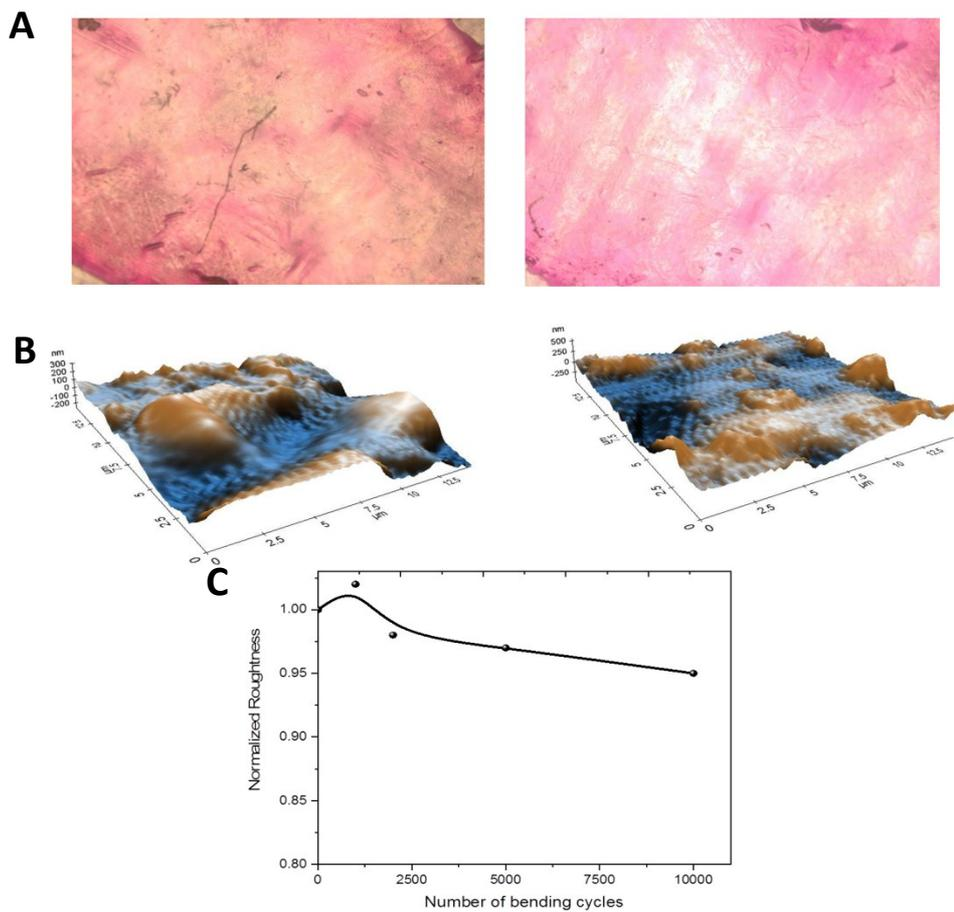
**Figure S7.** (A) Optical image of fresh (left) and after 10,000 bending cycles (right) of CTPR-Rh films. (B) AFM image of fresh (left) and after 10,000 bending cycles (right) of CTPR-Rh films. (C) Roughness changes versus number of bending cycles.
