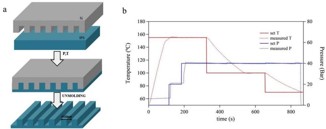
**Figure S9.** (a) Outline of the replication of a polymer grating from Si to IPS. (b) Temperature and pressure profiles during the nanoimprinting process.
