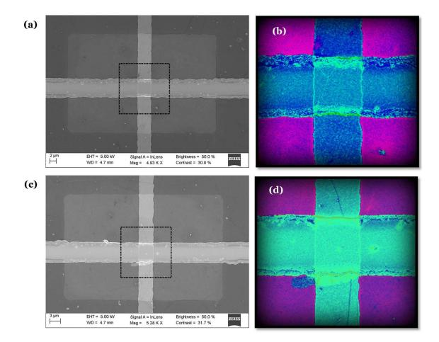
**Figure S2: Comparison of graphene film in D2 devices.** The SEM image of the D2 device (a) without and (c) with grain-boundary. Pseudo-colored SEM image of (b) a good cross-point and (d) a cross-point with prominent grain.
