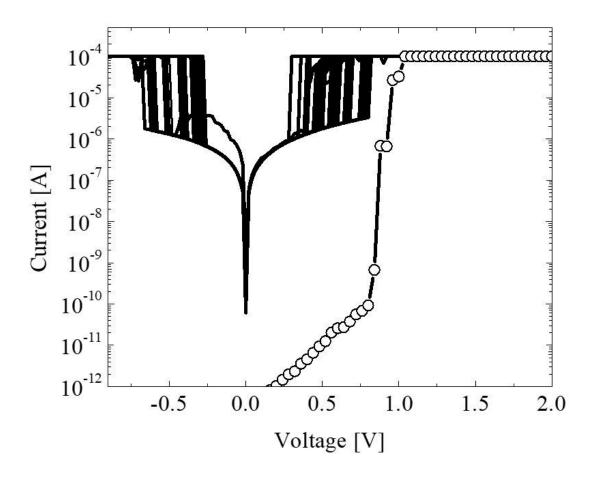
Figure S3: The TS in graphene-based devices. Defective graphene-barrier needed lower forming voltage  $\sim + 1$  V, can introduce bi-direction TS behavior in the graphene-based devices.
