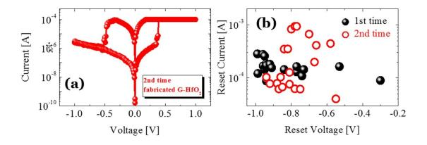
**Figure S1: Performance comparison of MS mode with re-fabricated D2 devices.** (a) The I-V switching characteristics of the 2<sup>nd</sup>-time fabricated graphene-based D2 devices. (b) The device-to-device variation of the reset current with reset voltage is showing symmetrical performances of the 1<sup>st</sup>-time and 2<sup>nd</sup>-time fabricated graphene-based D2 devices.
