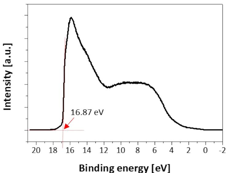
**Fig. S10** UPS spectrum of the CNF using He I excitation.
