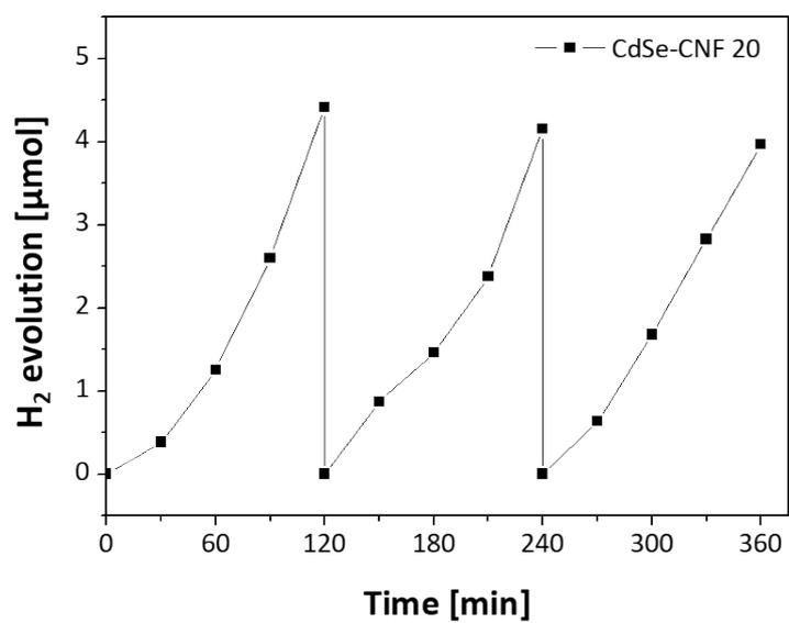
**Fig. S13** Stability test of photocatalytic hydrogen evolution of the CdSe-CNF 20 in 0.25 M Na<sub>2</sub>S/0.35 M Na<sub>2</sub>SO<sub>3</sub> aqueous solution under visible light ( $\lambda \geq 420$  nm)
