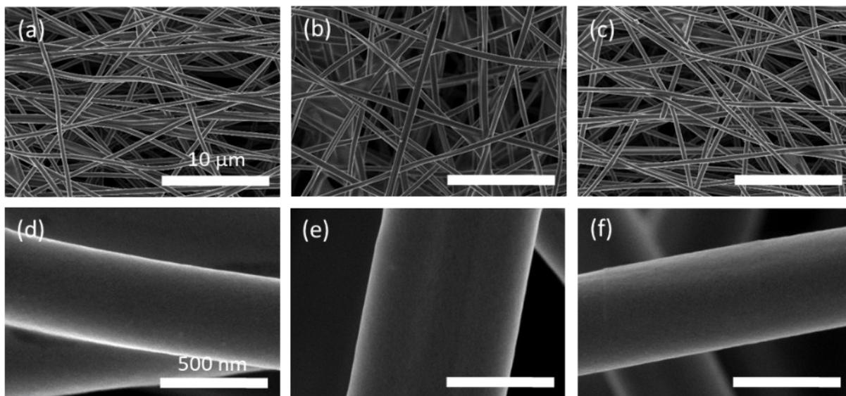
**Fig. S3** Low magnification SEM images of CdSe-CNF with different concentrations of QD: (a) 20 mg ml<sup>-1</sup>, (b) 50 mg ml<sup>-1</sup>, and (c) 100 mg ml<sup>-1</sup>. High magnification SEM images of CdSe-CNF with different concentrations of QDs: (d) 20 mg ml<sup>-1</sup>, (e) 50 mg ml<sup>-1</sup>, and (f) 100 mg ml<sup>-1</sup>.
