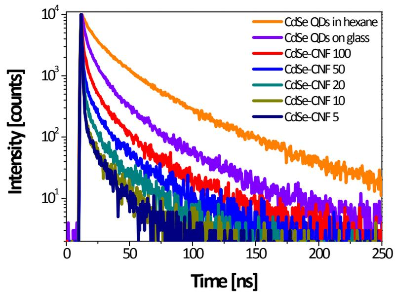
**Fig. S12** Transient PL decay curves of CdSe-CNF with different QDs concentrations from 5 mg ml<sup>-1</sup> to 100 mg ml<sup>-1</sup>.
