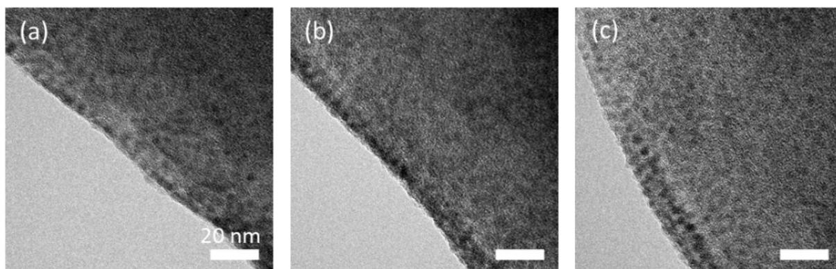
**Fig. S5** TEM images of CdSe-CNF with different concentrations of QD: (a) 20 mg ml<sup>-1</sup>, (b) 50 mg ml<sup>-1</sup>, and (c) 100 mg ml<sup>-1</sup>.
