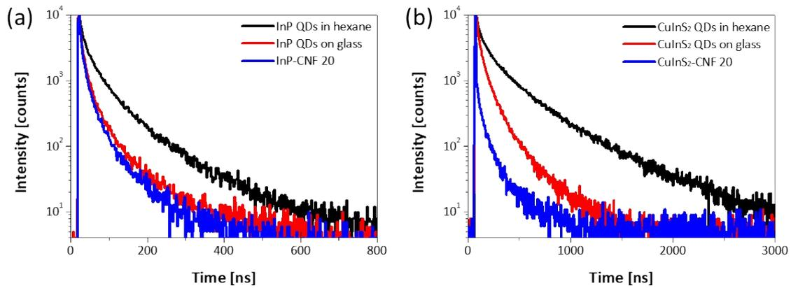
**Fig. S11** Transient PL decay curves of (a) InP-CNF and (b) CuInS<sub>2</sub>-CNF with the QDs concentration of 20 mg ml<sup>-1</sup>.
