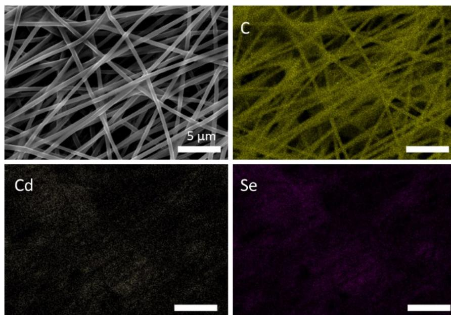
**Fig. S4** SEM-EDS mapping of C, Cd, and Se for CdSe-CNF 20.
