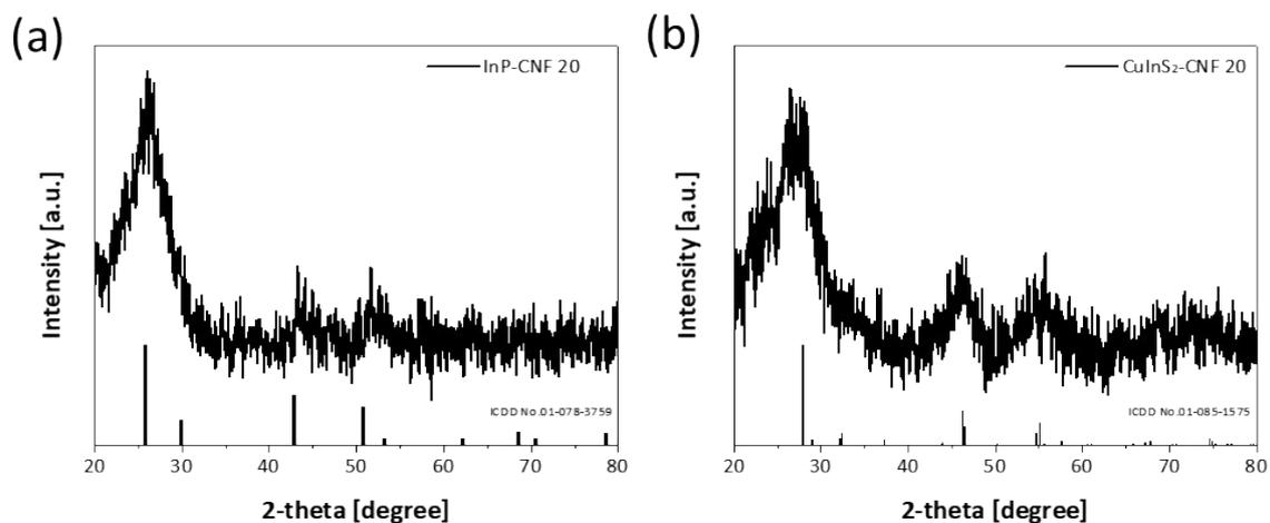
**Fig. S7** XRD patterns of (a) InP-CNF, and (c) CuInS<sub>2</sub>-CNF with the QD concentration of 20 mg ml<sup>-1</sup>.
