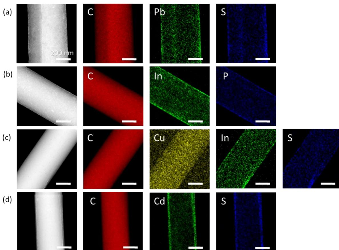
**Fig. S6** TEM-EDS mapping of single component QD-coated CNFs: (a) PbS, (b) InP, (c) CuInS<sub>2</sub>, and (d) CdS.
