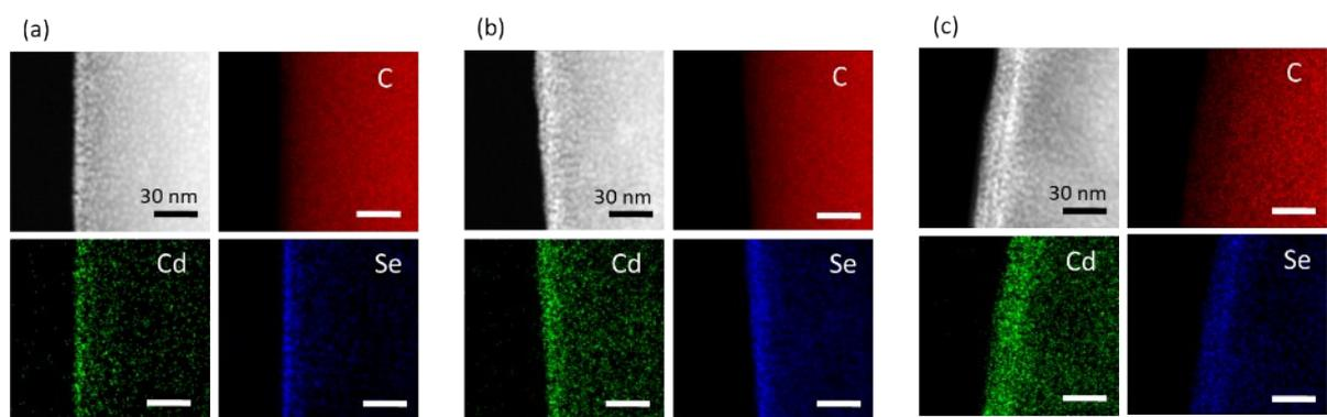
**Fig. S8** TEM-EDS elemental mapping images of (a) CdSe-CNF 20, (b) CdSe-CNF 50, and (c) CdSe-CNF 100.
