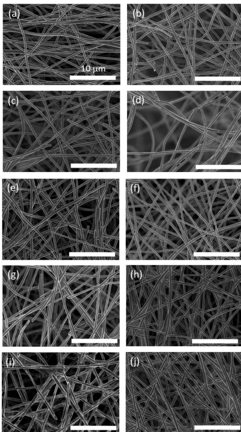
**Fig. S2** Low magnification SEM images of QD-coated CNFs: (a) CdSe, (b) PbS, (c) InP, (d) CuInS<sub>2</sub>, (e) CdS, (f) InP/ZnS, (g) CuInS<sub>2</sub>/ZnS, (h) CdSe/ZnS, (i) CdZnSeS/ZnS, and (j) CdZnS/ZnS.
