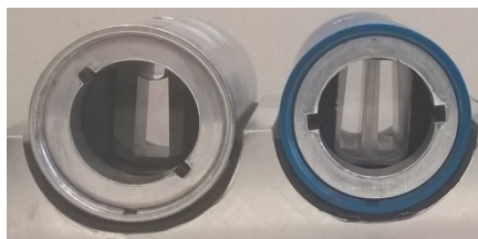
Figure S2 Comparison of mono-sector measurement cell for MWE-AUC and double-sector cell used in MWL-AUC.
