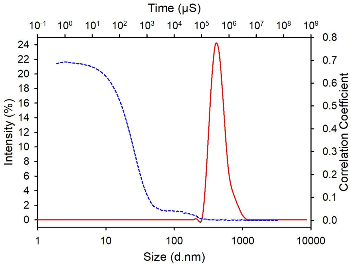
Figure S8. Size distribution and correlation coefficient of TDF precipitated with AOT/Maisine 35-1 and then freeze dried in the presence of sesame oil. Particles in oil samples are diluted into DCM prior to measurement. Measurements are an average of 3 scans using a Malvern Zetasizer Nano S dynamic light scattering instrument.
