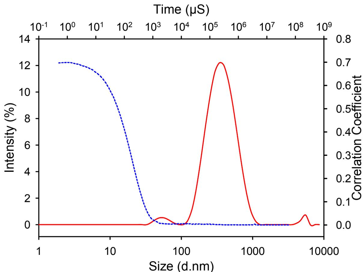
Figure S6. Size distribution and correlation coefficient of TDF precipitated with AOT and then freeze dried in the presence of sesame oil. Particles in oil samples are diluted into DCM prior to measurement. Measurements are an average of 3 scans using a Malvern Zetasizer Nano S dynamic light scattering instrument.
