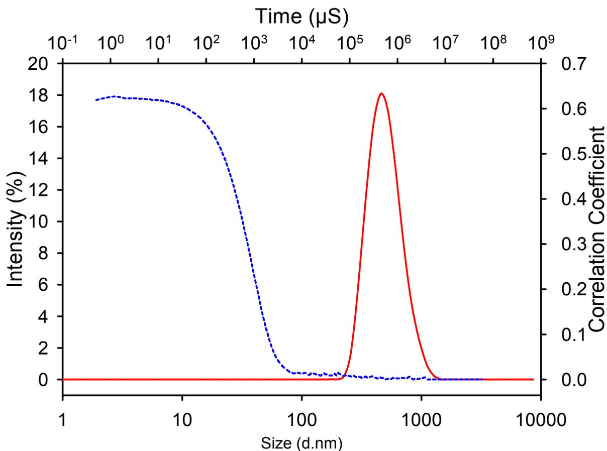
Figure S7. Size distribution and correlation coefficient of TDF precipitated with AOT/Lauroglycol FCC and then freeze dried in the presence of sesame oil. Particles in oil samples are diluted into DCM prior to measurement. Measurements are an average of 3 scans using a Malvern Zetasizer Nano S dynamic light scattering instrument.
