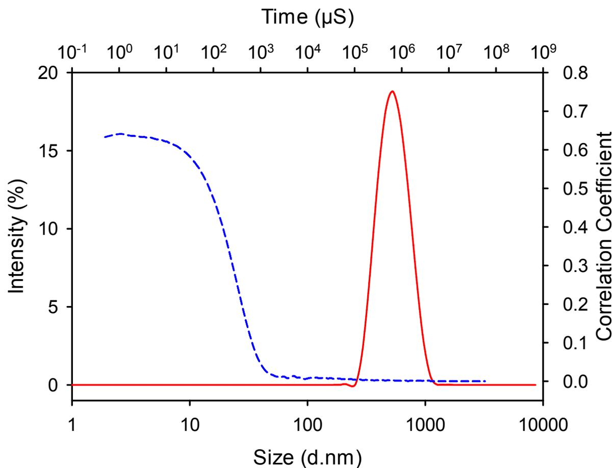
Figure S5. Size distribution and correlation coefficient of TDF precipitated with AOT and Maisine 35-1, measured in DCM continuous phase. Measurements are an average of 3 scans using a Malvern Zetasizer Nano S dynamic light scattering instrument.
