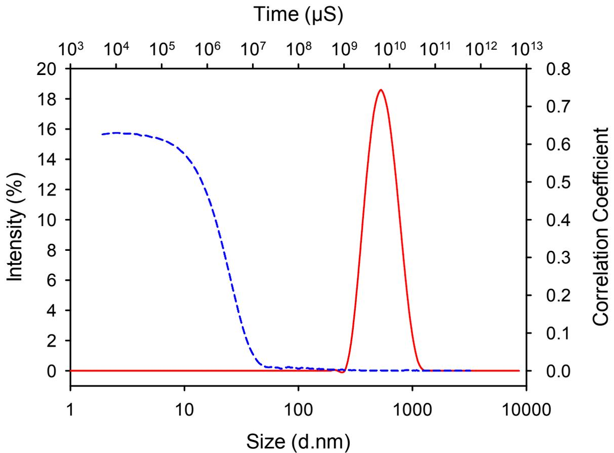
Figure S4. Size distribution and correlation coefficient of TDF precipitated with AOT and Lauroglycol FCC, measured in DCM continuous phase. Measurements are an average of 3 scans using a Malvern Zetasizer Nano S dynamic light scattering instrument.
