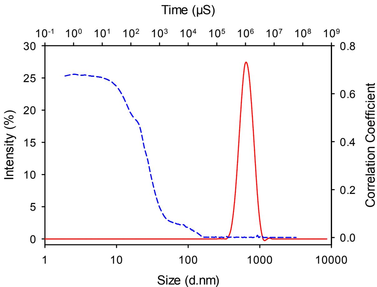
Figure S11. Size distribution and correlation coefficient of TDF precipitated with AOT/Maisine 35-1 and then freeze dried in the presence of peanut oil. Particles in oil samples are diluted into DCM prior to measurement. Measurements are an average of 3 scans using a Malvern Zetasizer Nano S dynamic light scattering instrument.
