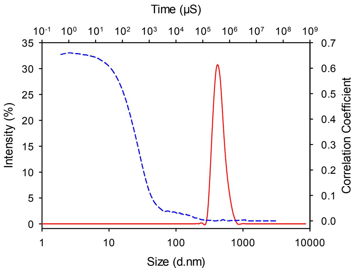
Figure S9. Size distribution and correlation coefficient of TDF precipitated with AOT and then freeze dried in the presence of peanut oil. Particles in oil samples are diluted into DCM prior to measurement. Measurements are an average of 3 scans using a Malvern Zetasizer Nano S dynamic light scattering instrument.
