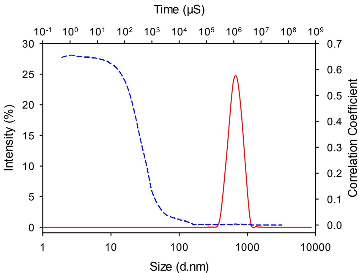
Figure S10. Size distribution and correlation coefficient of TDF precipitated with AOT/Lauroglycol FCC and then freeze dried in the presence of peanut oil. Particles in oil samples are diluted into DCM prior to measurement. Measurements are an average of 3 scans using a Malvern Zetasizer Nano S dynamic light scattering instrument.
