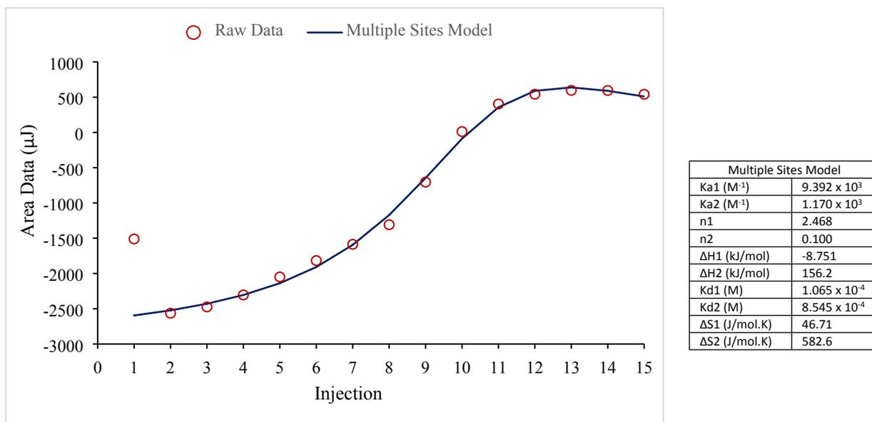
Figure S1. Multiple site model fitting for the isothermal titration calorimetry analysis of TDF/AOT nanoprecipitation in water.
