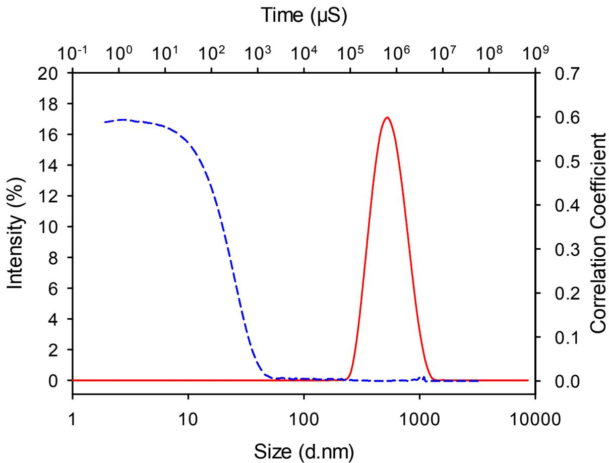
Figure S3. Size distribution and correlation coefficient of TDF precipitated with AOT and measured in DCM continuous phase. Measurements are an average of 3 scans using a Malvern Zetasizer Nano S dynamic light scattering instrument.
