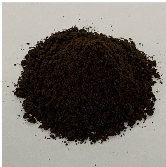
Fig. S1 The typical photograph of the lyophilized N, S-codoped CDs powder.
