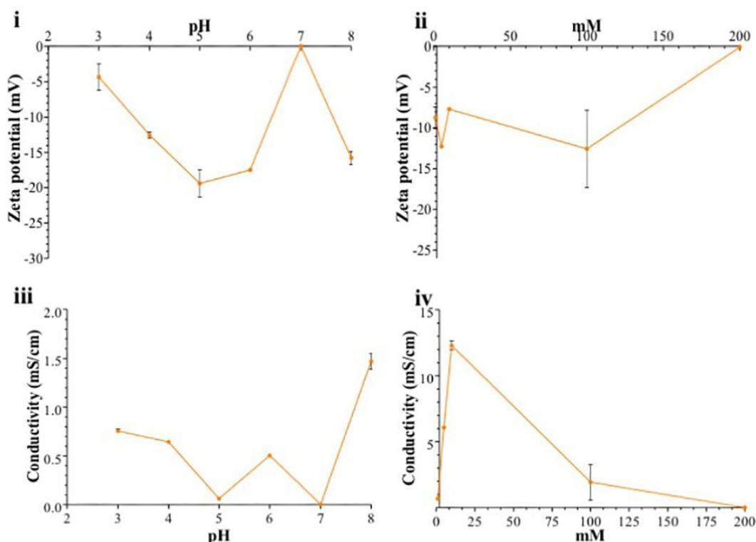
Figure S 3.1: Relationship between  $\zeta$  and C of MNP suspension and differ conditions. i)  $\zeta$  of MNP in PBS pH6.5 at 200, 100, 10, 5 and 1 mM concentrations. ii)  $\zeta$  of the MNP in 10 mM MES at different pH ranging from 3 until 8. iii) C of MNP in PBS pH6.5 at 200, 100, 10, 5 and 1 mM concentrations. iv) C of the MNP in 10 mM MES at different pH ranging from 3 until 8.
