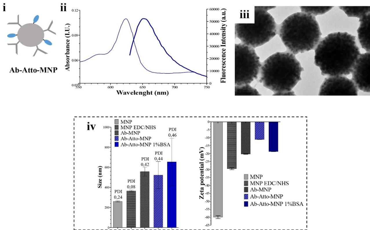
Figure S 2.6: i) Schematic structure of Ab-Atto-MNP. ii) UV-Vis spectrum (grey line) and fluorescent spectrum (blue line) for the 50 µg/mL in Di water. Ab-Atto-MNP absorb at 630 nm and emit at 655 nm. iii) TEM image of Ab-Flu-MNP. iv) Size and zeta potential measured by DLS analysis of the particles at each step of functionalization for 10 µg/mL of particle in filtered DI water.
