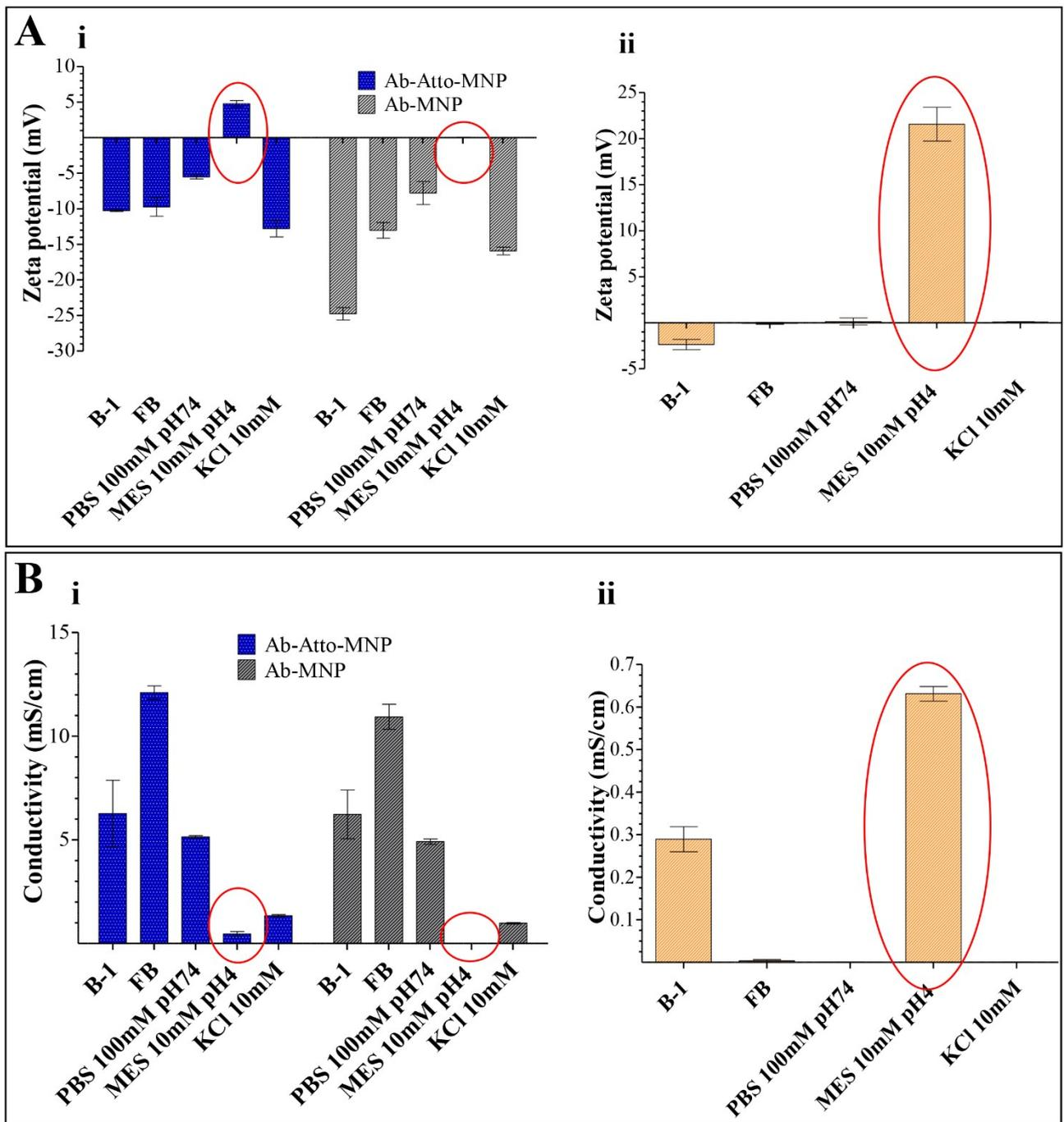
Figure S 3.4: DLS data achieved for Ab-Atto-MNP (blue bars) and Ab-MNP (grey bars) measuring  $\zeta$  (A) and C (C) in different buffers. DLS data achieved for St-G-FITC-SiNP measuring  $\zeta$  (B) and C (D) in different buffers. 10 mM MES pH4 was chosen as the suitable buffer for quantification assays with these particles.
