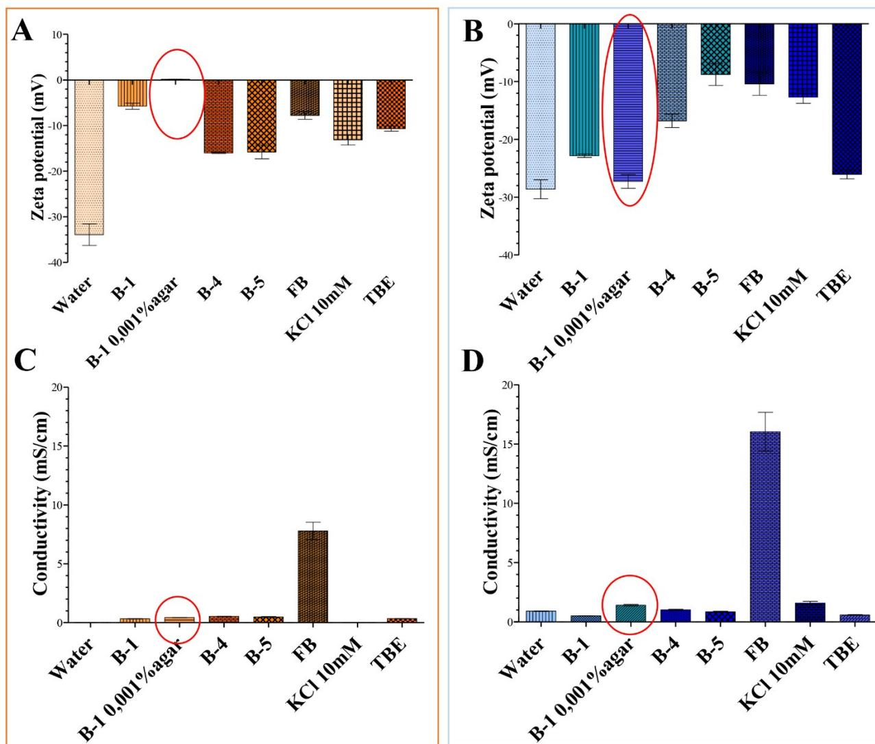
Figure S 3.3: DLS data achieved for Ab-Flu-MNP measuring  $\zeta$  (A) and C (C) in different buffers. DLS data achieved for St-G-MB-SiNP measuring  $\zeta$  (B) and C (D) in different buffers. B-1 0,001% of agarose was chosen as the suitable buffer for tracking analysis with these particles.
