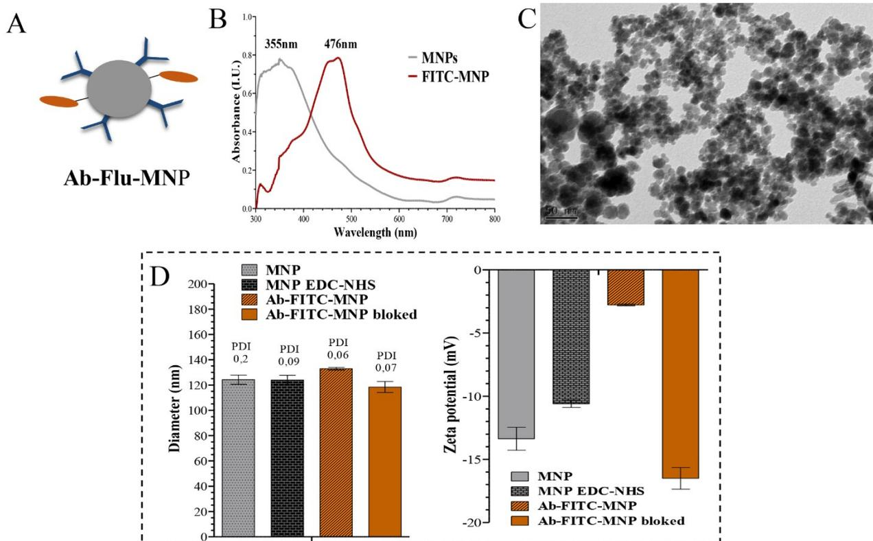
Figure S 2.4: A) Schematic structure of Ab-Flu-MNP. B) UV-Vis spectrum of the particles before functionalization (grey line- MNPs) and after functionalization with Ab and fluorescein amine (orange line- Ab-Flu-MNP). Whereas plane MNP have a broad absorbance peak at c.a. 350 nm, Ab-Flu-MNP absorb at 476 nm. C) TEM image of Ab-Flu-MNP. D) Size and zeta potential measured by DLS analysis of the particles at each step of functionalization for 10 µg/mL of particle in filtered DI water.
