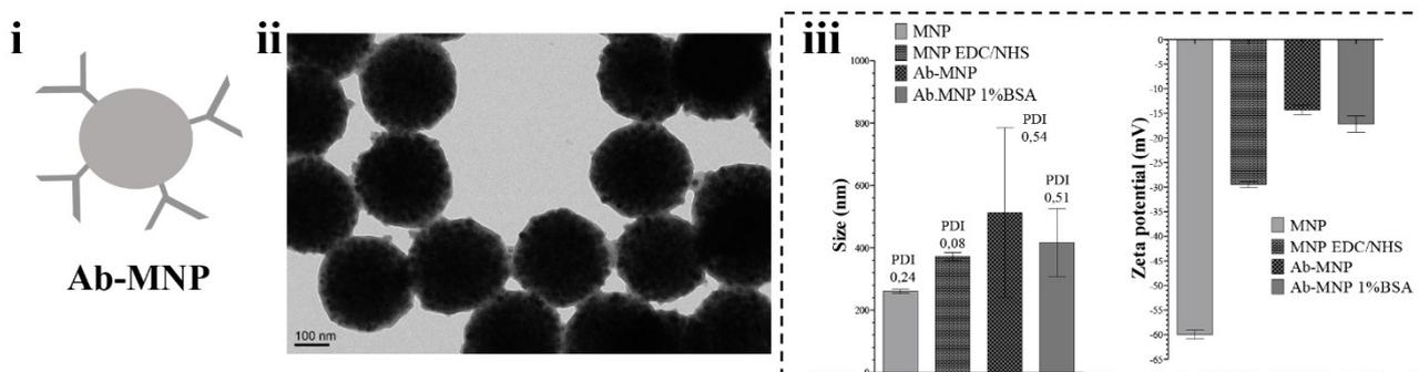
Figure S 2.5: Structure (i) and TEM (ii) of Ab-MNP; iii) DLS data related to size and zeta potential of the particles at each step of functionalization.
