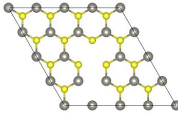
**Fig. S8**  $V_{1W+2S}$  vacancy complex consisting of W, S-D<sub>up</sub> and S-D<sub>down</sub> vacancies with  $M_{tot}=0 \mu B$ .
