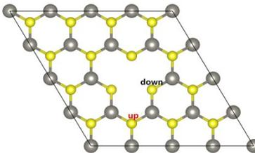
**Fig. S11**  $V_{1W+2S}$  vacancy complex consisting of W, S-A<sub>up</sub> and S-D<sub>down</sub> vacancies with  $M_{tot}=0 \mu B$ .
