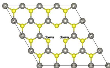
**Fig. S6**  $V_{1W+2S}$  vacancy complex consisting of W, S-A<sub>up</sub> and S-B<sub>up</sub> vacancies with  $M_{tot}=0 \mu_B$ .
