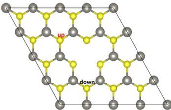
**Fig. S9**  $V_{1W+2S}$  vacancy complex consisting of W, S-D<sub>up</sub> and S-E<sub>down</sub> vacancies with  $M_{tot}=0 \mu B$ .
