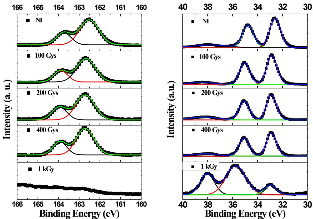
**Fig. S2** XPS spectrum of the Non-irradiated (NI) and irradiated samples, all showing two and three peaks for the S2p and W4f core levels, respectively, as reported previously for 2D-WS<sub>2</sub>. The solid lines represent their respective peak deconvolution.
