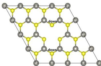
**Fig. S12**  $V_{1W+2S}$  vacancy complex consisting of W, S-C<sub>up</sub> and S-D<sub>up</sub> vacancies with  $M_{\text{tot}}=0 \mu\text{B}$ .
