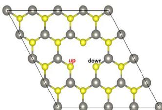
**Fig. S7**  $V_{1W+2S}$  vacancy complex consisting of W, S-A<sub>up</sub> and S-B<sub>down</sub> vacancies with  $M_{tot}=0 \mu_B$ .
