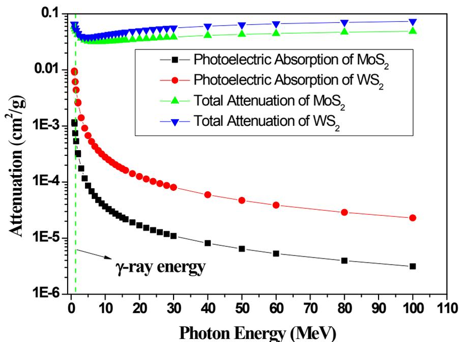
**Fig. S3** XCOM plots showing the  $\gamma$ -ray scattering mechanisms in MoS<sub>2</sub> and WS<sub>2</sub> as a function of radiation energies. The average energy for the Co<sup>60</sup>  $\gamma$ -rays, which is around 1.33 MeV is also shown as a reference.
