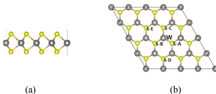
**Fig. S4** Side (a) and top (b) views of perfect  $WS_2$  monolayer. The gray and yellow spheres represent W and S atoms, respectively. The letters W, S-A, S-B,..., and S-E label W atom and its five neighbor S atoms.
