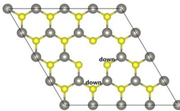
**Fig. S10**  $V_{1W+2S}$  vacancy complex consisting of W, S-A<sub>up</sub> and S-D<sub>up</sub> vacancies with  $M_{tot}=0 \mu B$ .
