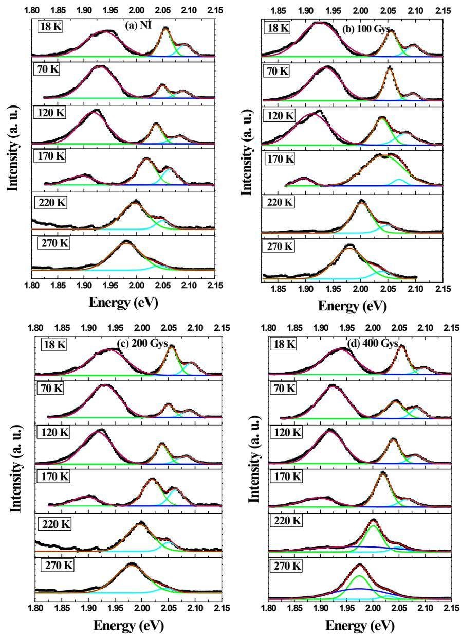
**Fig. S1** PL spectra at different temperatures as a function of irradiation dose and their respective peak deconvolution. (a) Non-irradiated (NI) sample, and irradiated samples (b) 100 Gys, (c) 200 Gys, (d) 400 Gys.
