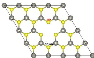
**Fig. S13**  $V_{1W+2S}$  vacancy complex consisting of W, S-C<sub>down</sub> and S-D<sub>up</sub> vacancies with  $M_{\text{tot}}=0 \mu\text{B}$ .
