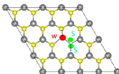
**Fig. S5**  $WS_2$  monolayer with  $V_{1W+2S}$  vacancy complex, consisting of one W vacancy (red sphere) and nearby one sulfur vacancy pair (green spheres) in upper and lower layers at A site. The gray and yellow spheres represent W and S atoms, respectively. Total magnetic moment is equal to  $2.0 \mu_B$ .
