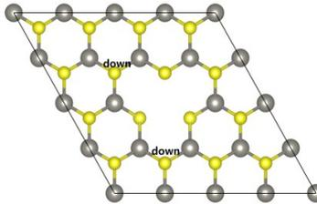
**Fig. S9**  $V_{1W+2S}$  vacancy complex consisting of W, S-D<sub>up</sub> and S-E<sub>up</sub> vacancies with  $M_{tot}=0 \mu B$ .
