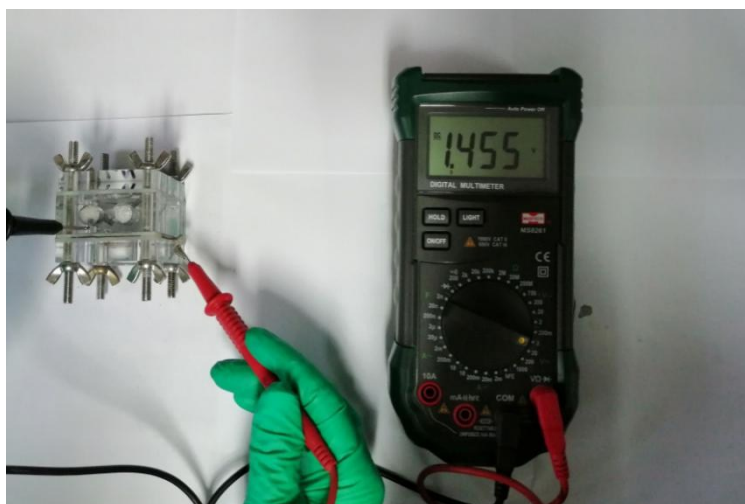
Fig. S33 Photograph of Zn-air battery using Fe-Fe@NC as cathode with an open circuit voltage of 1.45 V.
