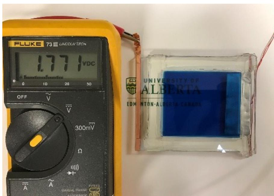
**Fig. S11.** The OCV of the prototype device increased to 1.77 V after colored/charged by a 1.8 V external voltage.
