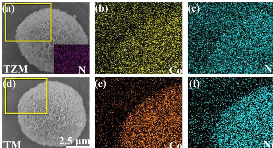
**Figure S2** EDS area mapping of the TZM (a) and TM (d), and corresponding Co (b and e), and Ni (c and f) elements, respectively (Inset is the area mapping of N).
