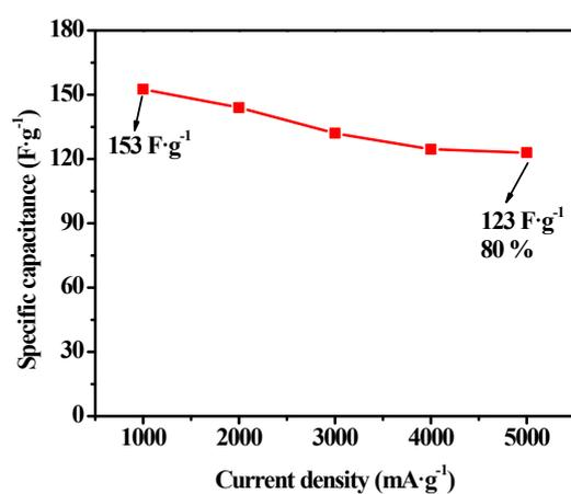
**Figure S3** Comparison of the specific capacitances of TZM//ACS aqueous asymmetric supercapacitor at various current densities
