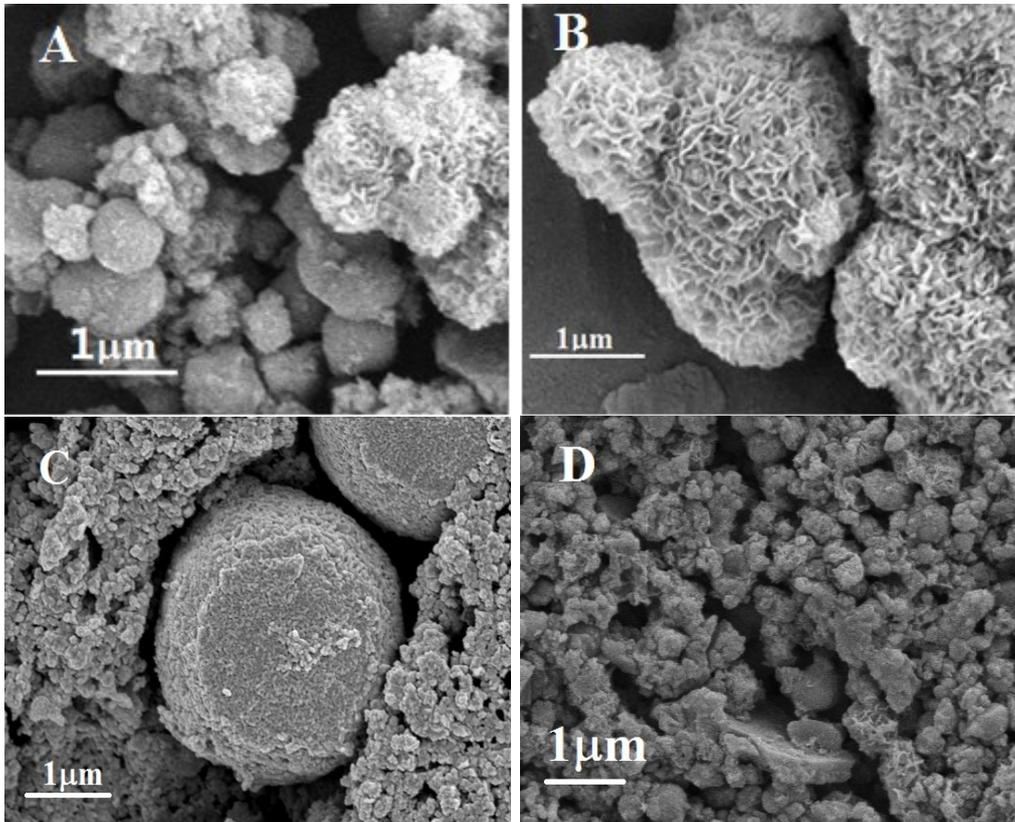
**Figure S1** SEM images of the products (TZM) prepared in 20h(A) and 48h(B); SEM images of TZM(C) and TM(D) after 2000 charging and discharging cycles
