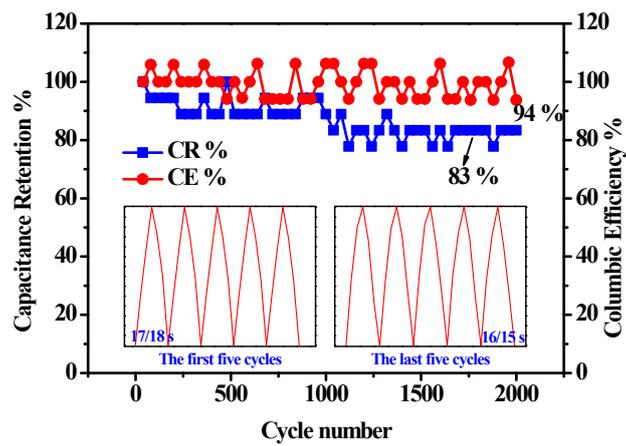
**Figure S4** Cycle stability performance for TZM//ACS aqueous asymmetric supercapacitor at the current density of  $10 \text{ A}\cdot\text{g}^{-1}$
