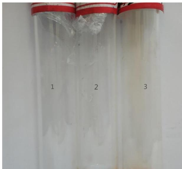
**Figure S2** Observation of tail gas colour in three sets of experiments using  $\text{KNO}_3/\text{TiPO}$  catalyst ( $\text{KNO}_3 : \text{TiPO} = 4:1$ )
