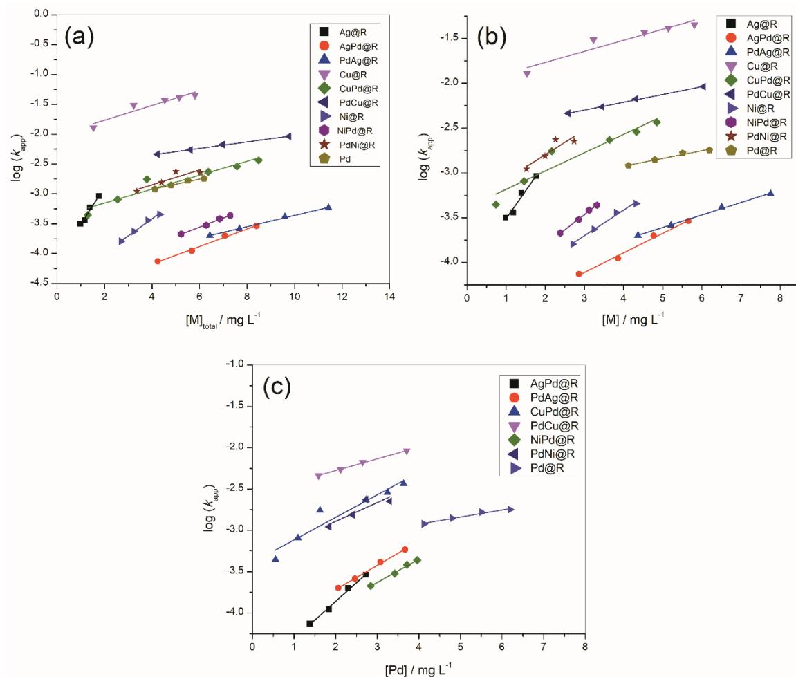
**Figure S6.**  $k_{\text{app}}$  for the Nip catalytic reduction reaction as a function of: (a) the total concentration of metals; (b) selected metals (Ag, Cu, Ni) and (c) the concentration of Pd. ([Nip] = 0.1 mmol L<sup>-1</sup>, [NaBH<sub>4</sub>] = 100 mmol L<sup>-1</sup>, at 15 °C).
