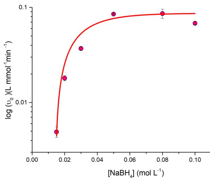
**Figure S5.**  $k_{app}$  for the reduction of Nip as a function of  $[NaBH_4]$  ( $[Nip] = 0.1 \text{ mmol L}^{-1}$ ,  $[Cu@R] = 1.53 \text{ mg L}^{-1}$ , at  $15^\circ\text{C}$ , in water).
