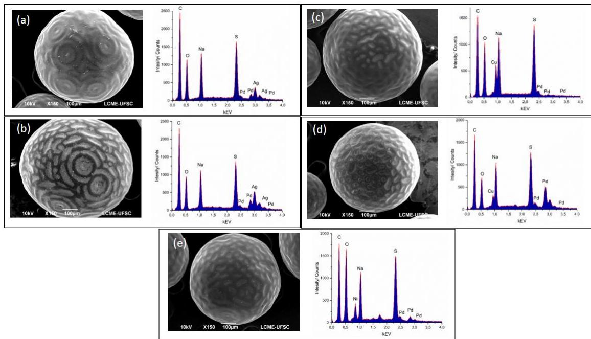
**Figure S1.** SEM micrographs and their respective EDS spectra of synthesized bimetallic nanocatalysts: (a) AgPd@R, (b) PdAg@R, (c) CuPd@R, (d) PdCu@R and (e) NiPd@R.
