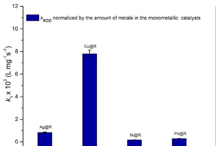
**Figure S7.** Catalytic activity ( $k_1$ ) of resin-supported nanoparticles considering the total amount of metals for the monometallic nanoparticles for the Nip reduction reaction.
