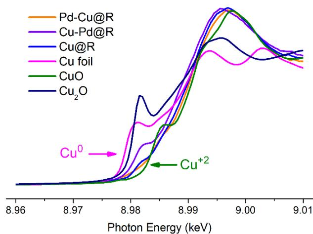
**Figure S3.** XANES spectra at Cu-edge for the Cu-based catalysts, Cu foil and CuO and Cu<sub>2</sub>O standards.
