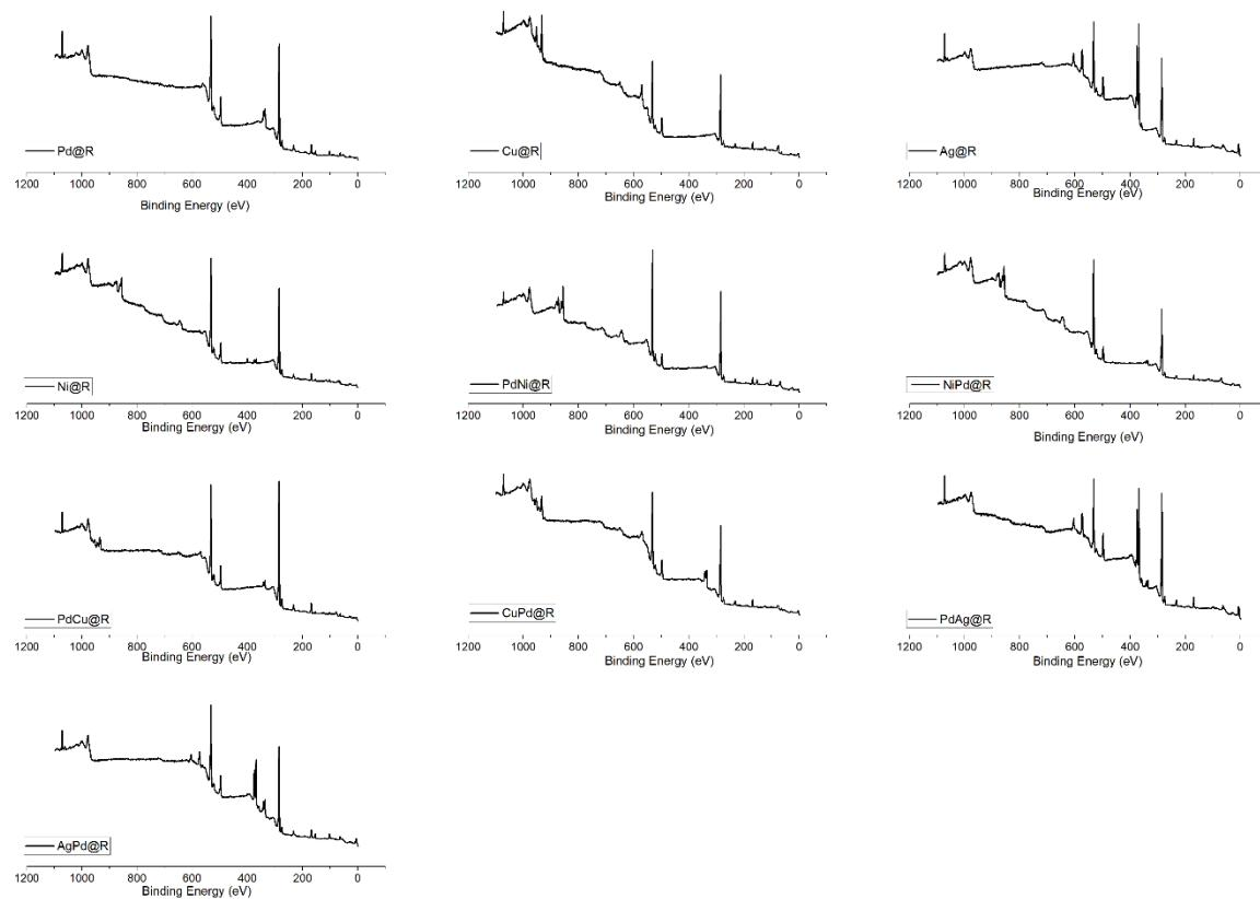
**Figure S2.** XPS survey spectra for all catalysts.
