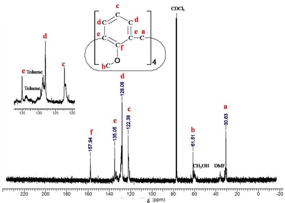
**Figure S8**  $^{13}\text{C}$ -NMR spectra of  $[4]\text{CH}_3$  (**4**)
