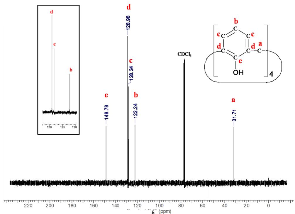
**Figure S5**  $^{13}\text{C}$ -NMR spectra of [4]H (3)
