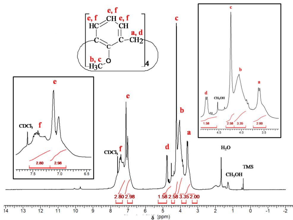
**Figure S7**  $^1\text{H}$ -NMR spectra of [4]CH<sub>3</sub> (4)
