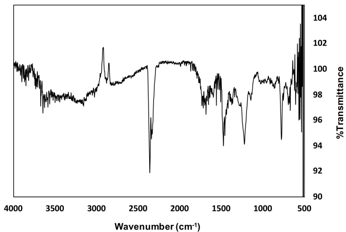
**Figure S9** FT-IR Spectra of MC-[4]H (direct synthesis from **3** with *s*-trioxane)
