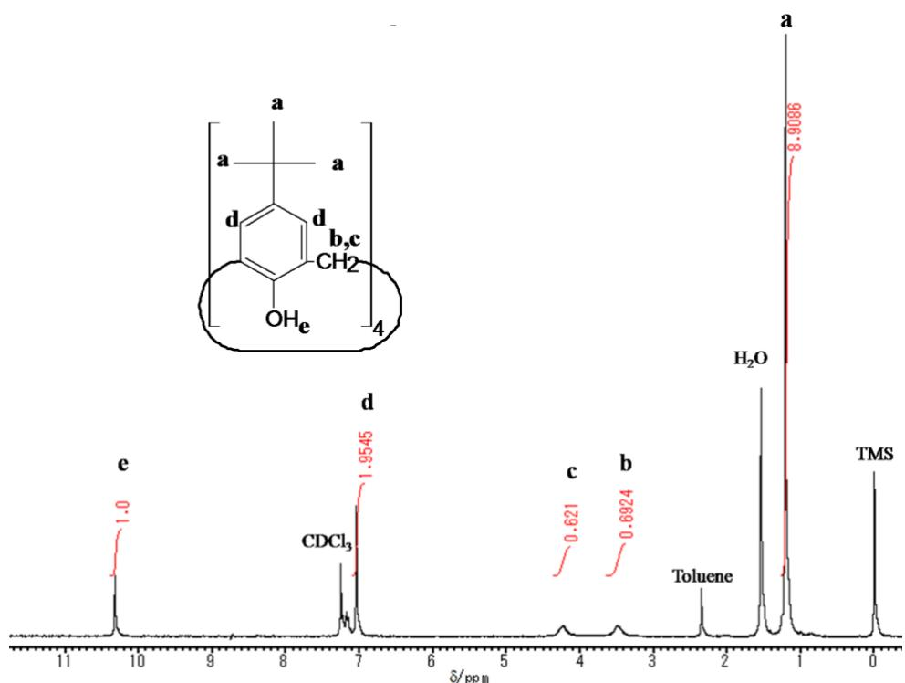
**Figure S2** <sup>1</sup>H-NMR spectra of <sup>t</sup>Bu[4]H (2)
