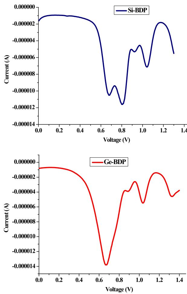
**Figure S1** DPV oxidation potential curves of Si-BDP and Ge-BDP dyes in  $\text{CH}_2\text{Cl}_2$  solution
