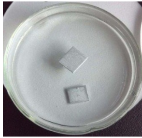
Fig.S6 Picture of the pre-treated Al sheet and SHS fabricated on Al substrate, superhydrophobic test floating on water.
