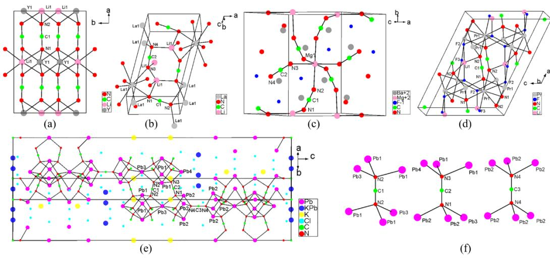
Figure S5. Crystal structures of (a)  $\text{LiY}(\text{CN}_2)_2$ , (b)  $\text{LiLa}(\text{CN}_2)_2$ , (c)  $\text{Ba}_4\text{Mg}(\text{CN}_2)_4\text{F}_2$ , (d)  $\text{LiPr}_2(\text{CN}_2)_2\text{F}_3$  and (e) **1**. (f) The coordination environment of  $\text{CN}_2$  in **1**.
