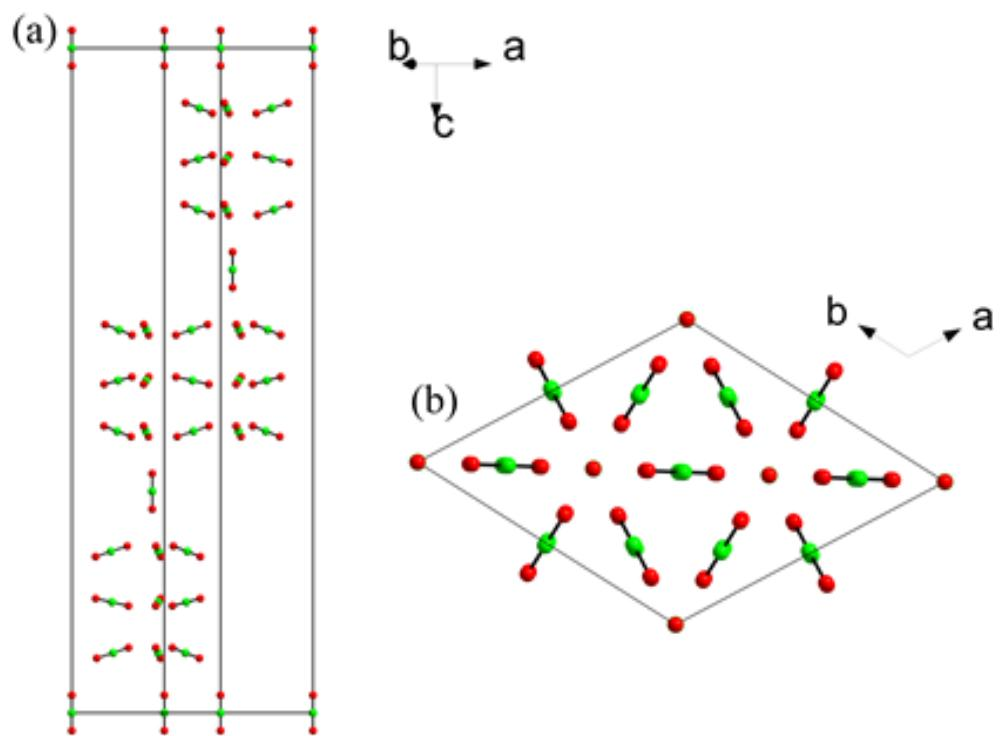
Figure S9. (a) Arrangement of  $\text{CN}_2$  groups along  $c$  axis and (b) projection of the  $\text{CN}_2$  units at  $ab$  plane.
