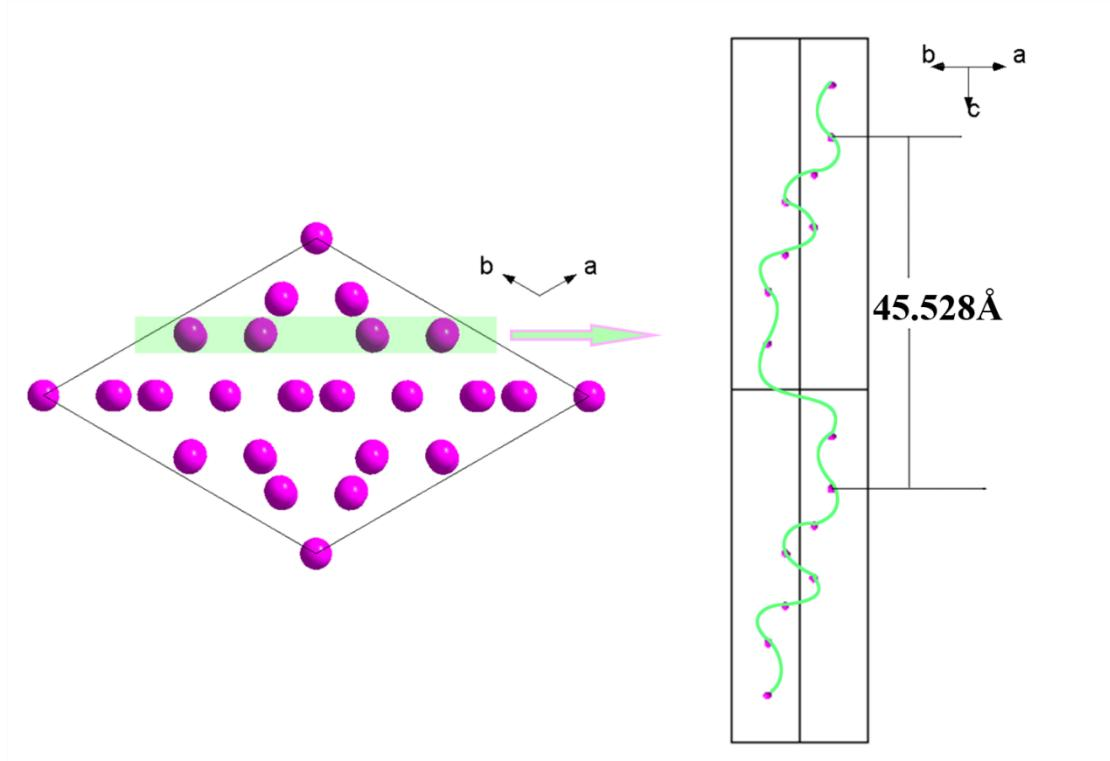
Figure S3. The rotation of  $\text{Pb}^{2+}$  cations along  $c$  axis.
