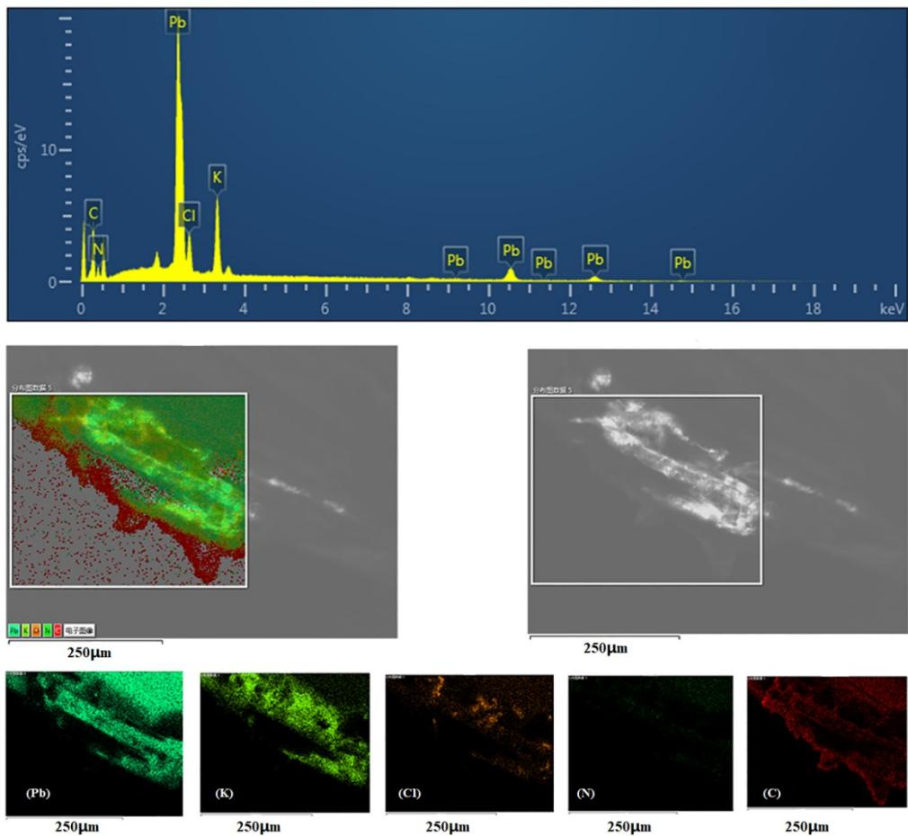
Figure S6. Elemental analysis spectrum of **1**.
