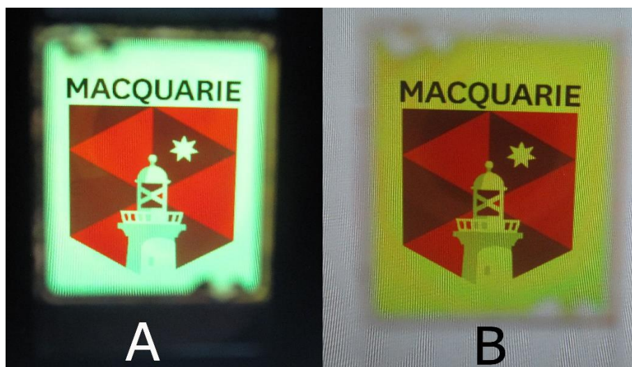
The planar cell placed between a pair of crossed (A) and parallel (B) linear polarizers
