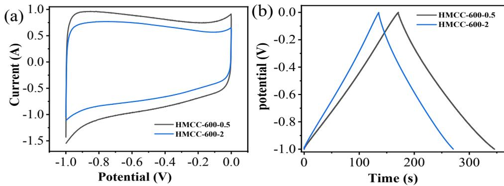
**Figure S1** Electrochemical performance of HMCC-600-0.5 and HMCC-600-2 in three-electrode system. (a) Cyclic voltammograms curves at  $5 \text{ mV s}^{-1}$ , (b) Galvanostatic charge/discharge curves at  $1 \text{ A g}^{-1}$ .
