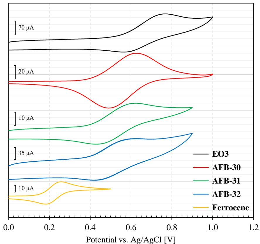
**Fig. S4** Cyclic voltammograms of all dyes on TiO<sub>2</sub> measured in acetonitrile with 0.1 M LiTFSI, with a carbon counter electrode and Ag/AgCl reference electrode. For the measurement of ferrocene, the working electrode was a glassy carbon electrode.
