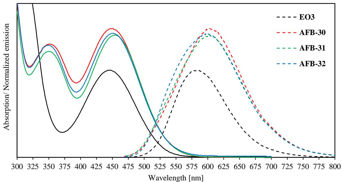
**Fig. S3** Absorption spectra in solution plotted with corresponding normalized emission spectra (dashed lines). The intersects dictates the optical bandgaps. Intersecting wavelengths: **EO3** 521 nm, **AFB-30** 520 nm, **AFB-31** 518 nm and **AFB-32** 518 nm.
