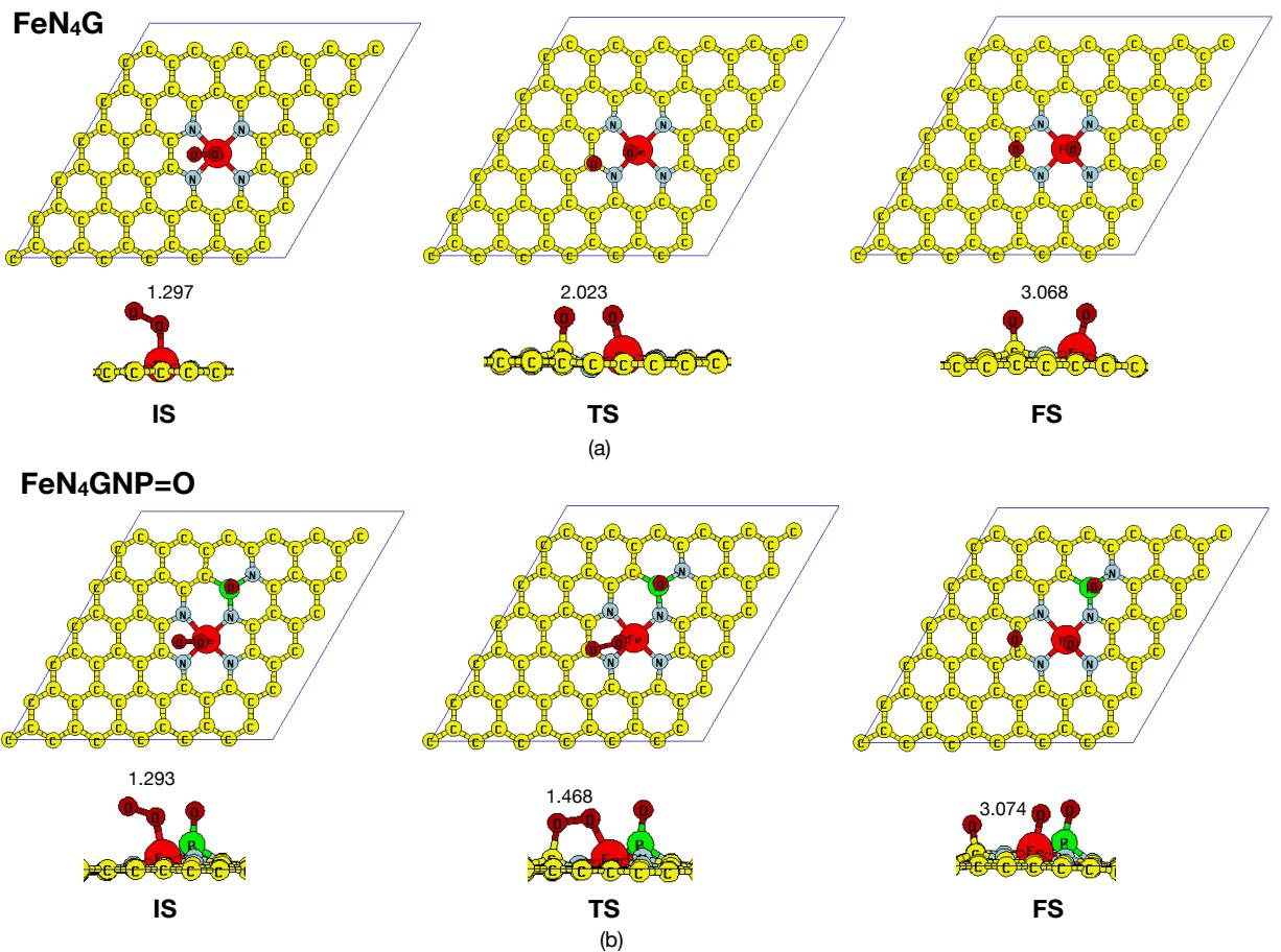
Figure S11: Initial state (IS), transition state (TS) and final state (FS) configurations of O<sub>2</sub> dissociation on the FeN<sub>4</sub> site of FeN<sub>4</sub>G-NP=O (a) and undoped FeN<sub>4</sub>G systems (b).
