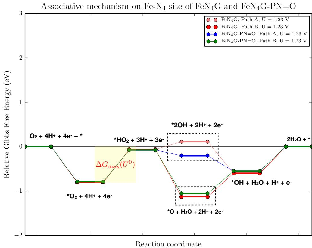
Figure S8: ORR energy profiles at  $U = 1.23$  V for associative mechanism on the FeN<sub>4</sub> site of FeN<sub>4</sub>G-NP=O system compared to that of undoped FeN<sub>4</sub>G system.
