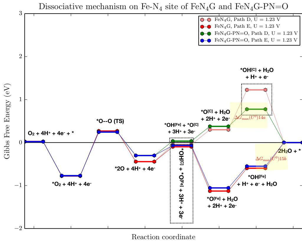
Figure S9: ORR energy profiles at  $U = 1.23$  V for dissociative mechanism on the FeN<sub>4</sub> site of FeN<sub>4</sub>G-NP=O system compared to that of undoped FeN<sub>4</sub>G system.
