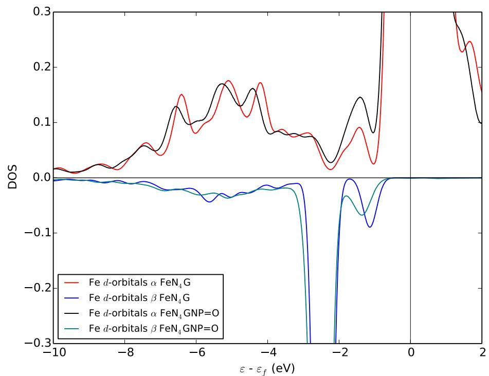
Figure S7: Local density of states (LDOS) of the d-states of FeN<sub>4</sub>G-NP=O and undoped FeN<sub>4</sub>G.
