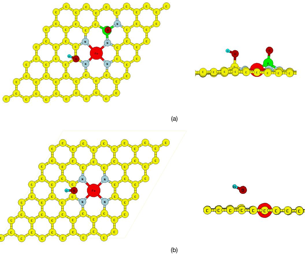
Figure S12: OH adsorption configurations on the C site of FeN<sub>4</sub>G-NP=O system (a) and undoped FeN<sub>4</sub>G system (b).
