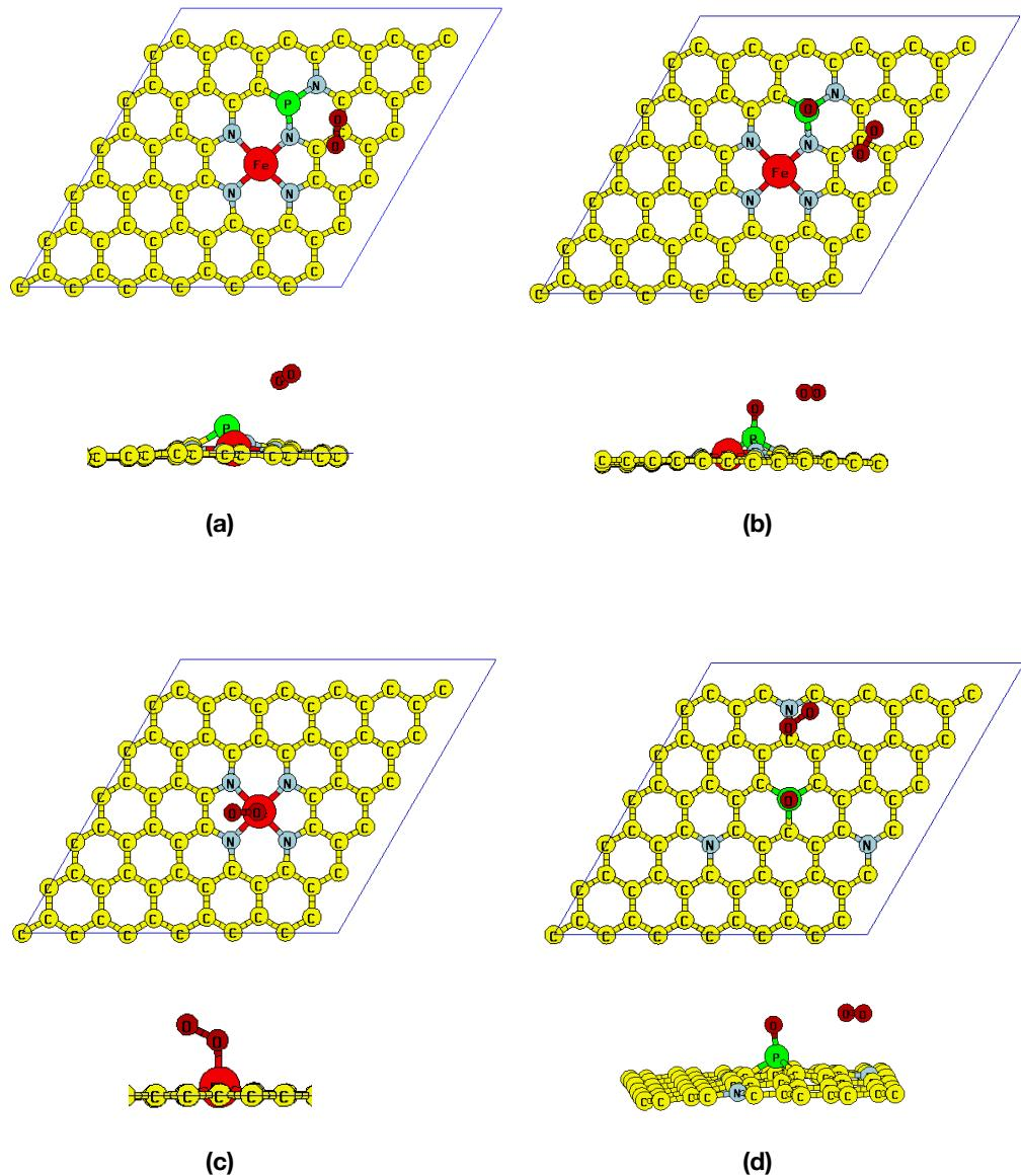
Figure S2: O<sub>2</sub> adsorption configurations on C-N site of FeN<sub>4</sub>G-NP (a), C-N site of FeN<sub>4</sub>G-NP=O (b), FeN<sub>4</sub> site of undoped FeN<sub>4</sub>G (c) and C-N site of GN<sub>3</sub>PO (d).
