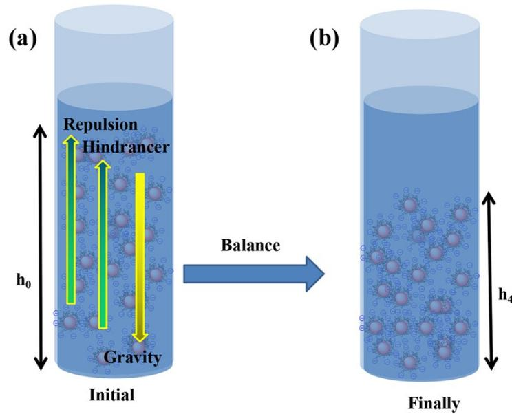
**Fig.S13** Subside model of PVP and TMAH modified SiC powder in water medium.
