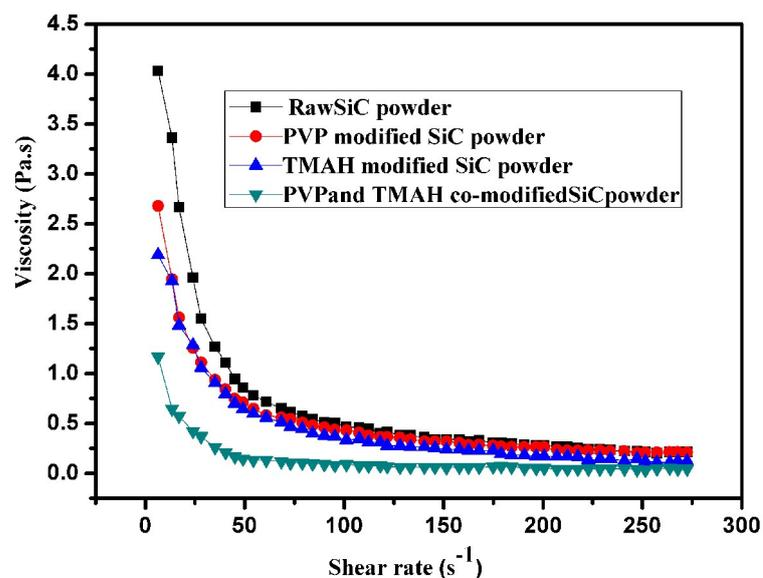
**Fig.S8** Effect of shear rate on viscosity (45 Vol% of solid content).
