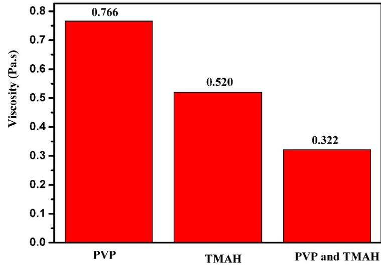
**Fig.S5** Minimum viscosity contrast of slurry prepared with SiC powder modified with different modifier.
