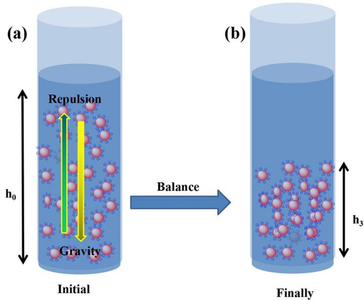
**Fig.S12** Subside model of TMAH modified SiC powder in water medium.
