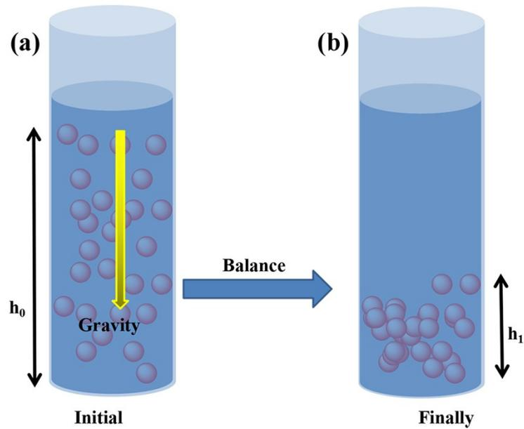
**Fig.S10** Subside model of original SiC powder in water medium.
