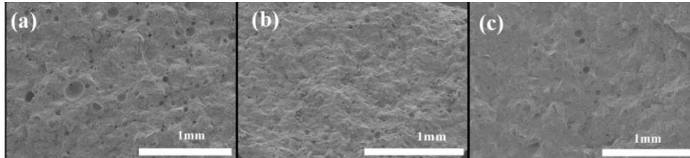
**Fig.S7** Fracture surface SEM image of SiC ceramic green body fabricated by different modified SiC powder, (a) PVP modified SiC powder, (b) TMAH modified SiC powder, (c) PVP and TMAH co-modified SiC powder.
