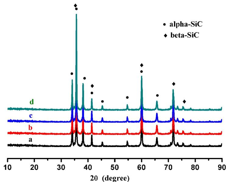
**Fig.S9** XRD patterns of the original SiC powder (a), PVP modified SiC Powder (b), TMAH modified SiC Powder (c) and (d) TMAH and PVP co-modified SiC powder.
