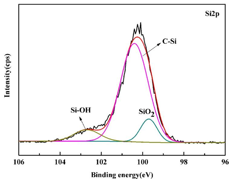
**Fig.S3** Si<sub>2p</sub> XPS spectra of the original SiC powder.
