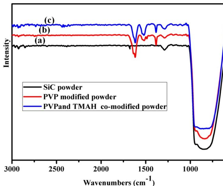
**Fig.S4** FT-IR spectra of different powder, (a) SiC powder, (b) PVP modified SiC powder and (c) PVP and TMAH co-modified SiC powder.
