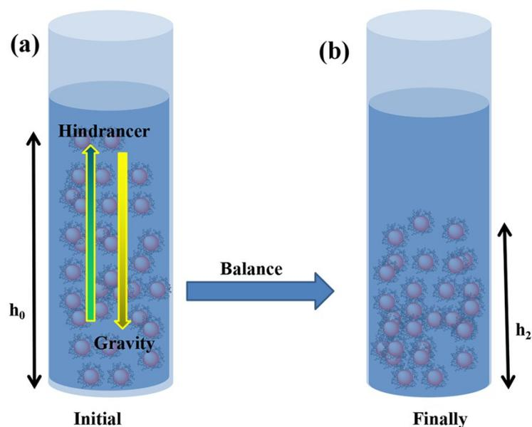
**Fig.S11** Subsidence model of PVP modified SiC powder in water medium.
