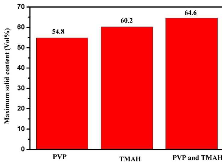
**Fig.S6** Maximum solid content contrast of slurry prepared with SiC powder modified with different modifier.
