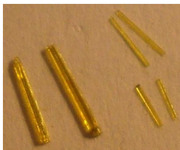
Fig. S1 Single crystals of [VOL(OPr)(H 2 O)] ( 2 ) isolated by solvent evaporation at low temperature.
