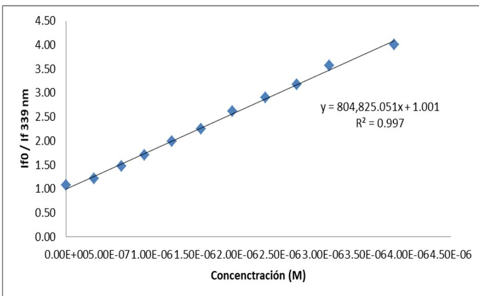
**Figure S18.** Stern-Volmer plot for  $[V^{IV}O(L2-H)_2]$
