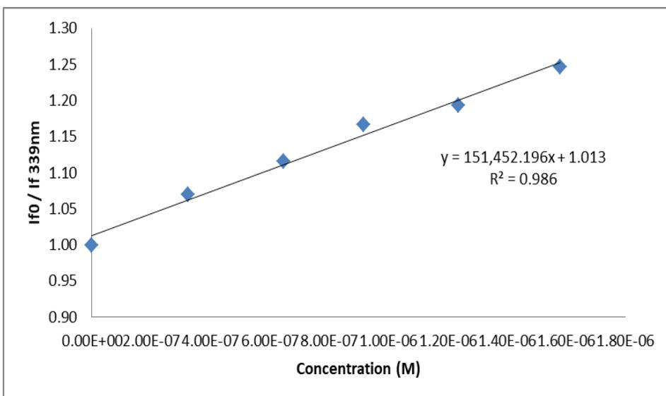
**Figure S20.** Stern-Volmer plot for  $[V^{IV}O(L3-H)_2]$
