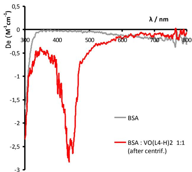
**Figure S14.** Circular dichroism spectra in the range of 300-800 nm of solutions containing BSA ( $\sim 300 \mu M$ ) and  $[V^{IV}O(L4-H)_2]$  complexes. The molar ratio is indicated. Quartz cells with optical path of 0.5 and 1.0 cm was used. In this experiment there were some problems with precipitation of a solid inside the cell.
