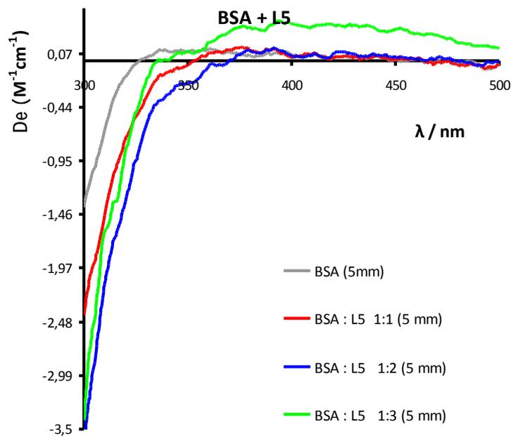
**Figure S11.** Circular dichroism spectra in the range of 300-500 of solutions containing BSA (~300 mM) and L5. The molar ratio is indicated. Quartz cell with optical path of 0.5 cm was used.
