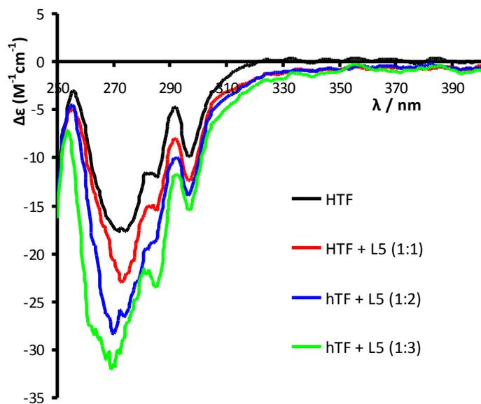
**Figure S8.** Circular dichroism spectra in the range 250-500 of solutions containing apo-HTF ( $\sim 150$  mM) and free ligand precursor L5 with different apo-HTF:ligand molar ratios.
