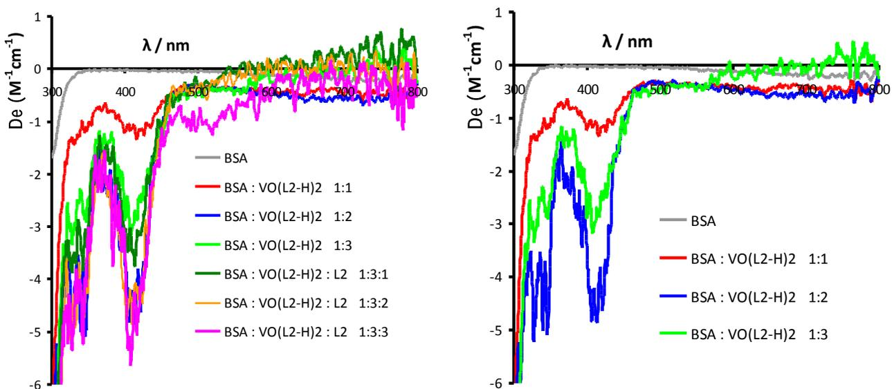
**Figure S12.** Circular dichroism spectra in the range of 300-800 nm of solutions containing BSA ( $\sim 300 \mu\text{M}$ ) and  $[\text{V}^{\text{IV}}\text{O}(\text{L2-H})_2]$  complexes, followed by additions of L2. The molar ratios are indicated. Quartz cells with optical path of 0.5 and 1.0 cm was used.
