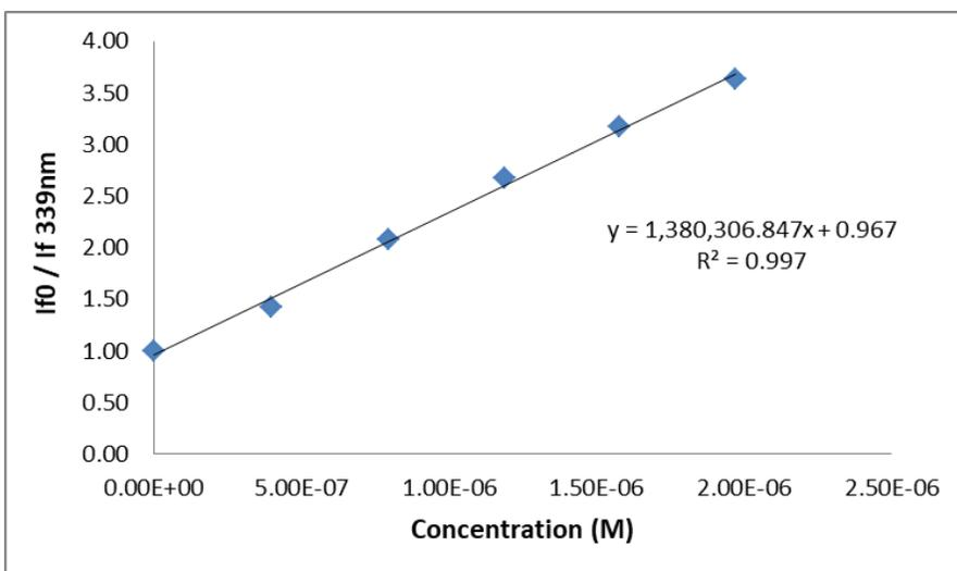
**Figure S16.** Stern-Volmer plot for L1
