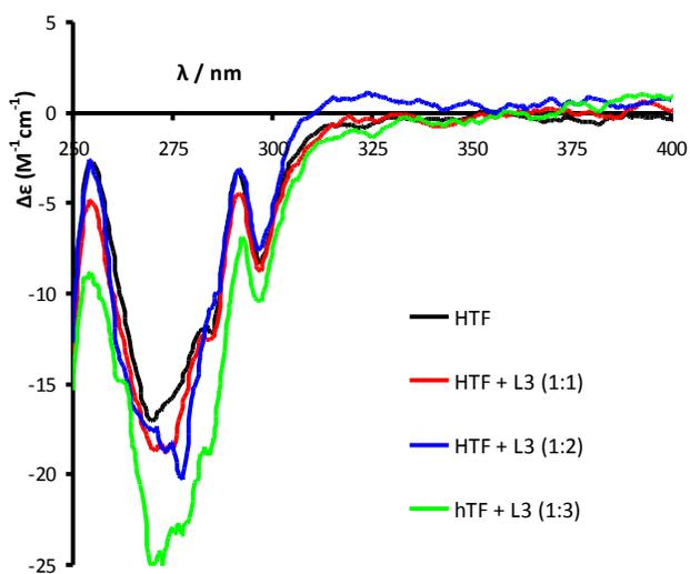
**Figure S7.** Circular dichroism spectra in the range 250-400 of solutions containing apo-HTF (~150 mM) and free ligand precursor L3 with different apo-HTF:ligand molar ratios.
