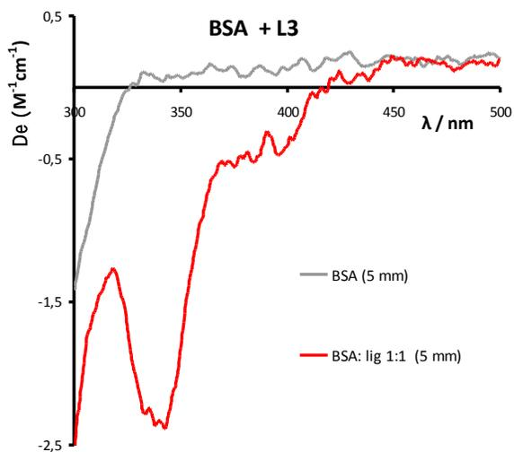
**Figure S10.** Circular dichroism spectra in the range of 300-500 of solutions containing BSA (~300 mM) and L3. The molar ratio is indicated. Quartz cell with optical path of 0.5 cm was used.
