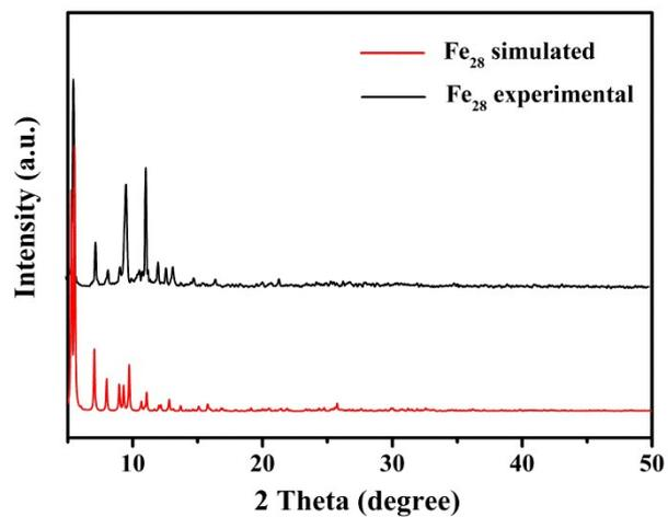
Fig. S1 XRD patterns of  $\text{Fe}_{28}$  powder samples.
