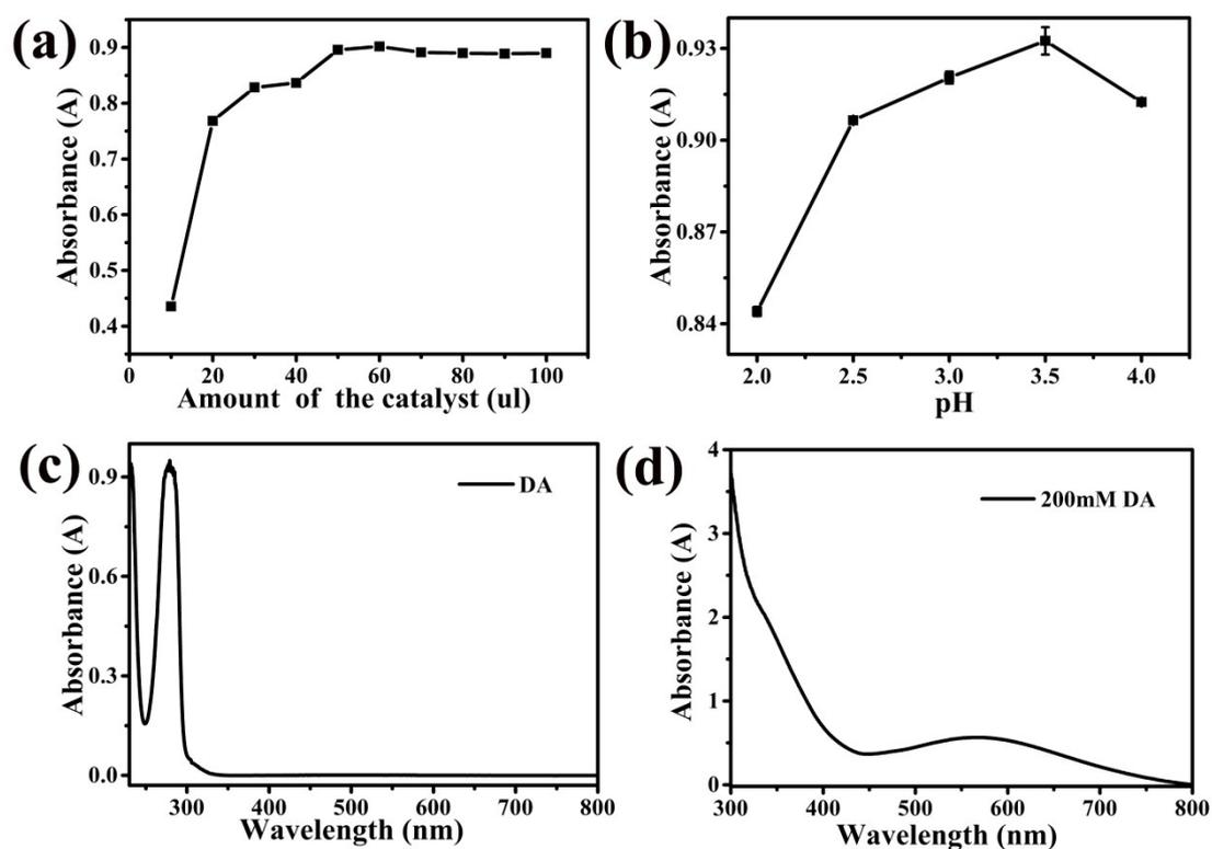
Fig. S4 (a) different amount of the catalyst facilitate the oxidation of DA at ultrapure water; (b) A pH dependent response curve for DA detection using  $\text{Fe}_{28}$  kept at 25 °C. The error bars represent the standard deviation of three measurements; (c) UV-vis absorption spectrum of the reaction solution of DA after 1 min; (d) UV-vis absorption spectrum of the reaction solution of DA with  $\text{Fe}_{28}$  after 1 min.
