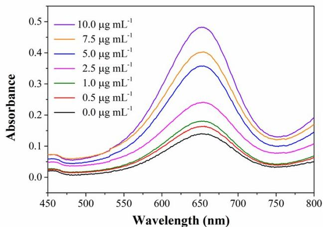
**Figure S3.** UV-vis absorption spectra of TMB and  $\text{H}_2\text{O}_2$  with different concentrations of MIL-53(Fe).  $[\text{TMB}] = 0.2 \text{ mM}$ ,  $[\text{H}_2\text{O}_2] = 2.5 \text{ mM}$ .
