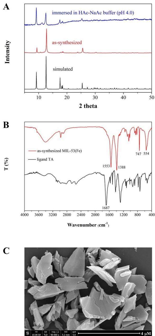
**Figure S2.** (A) PXRD patterns of MIL-53(Fe) under different conditions: simulated, as-synthesized, and immersed in 50 mM HAc-NaAc buffer (pH 4.0) under 3 h. (B) FTIR spectrum of as-synthesized MIL-53(Fe) and terephthalic acid (TA) ligand. (C) Typical SEM image of MIL-53(Fe).
