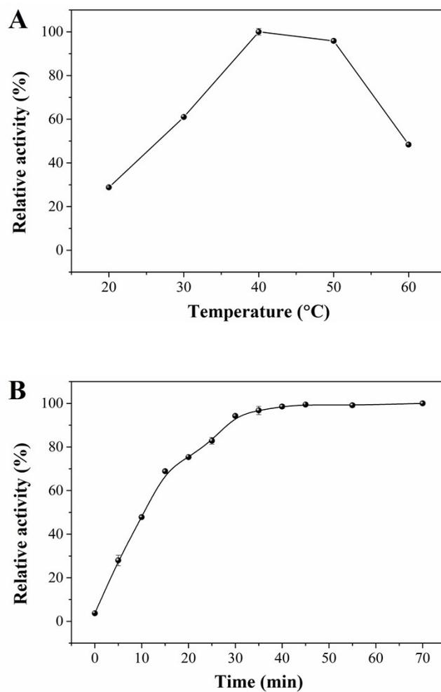
**Figure S8.** Effect of TMB oxidation temperature (A) and time (B) on the peroxidase-like activity of DNA-modified MIL-53(Fe). The absorbance was read at the maximum absorbance of 652 nm and the maximum point in each curve was set as 100 %. [M24] = 200 nM, [MIL-53(Fe)] = 5  $\mu\text{g mL}^{-1}$ .
