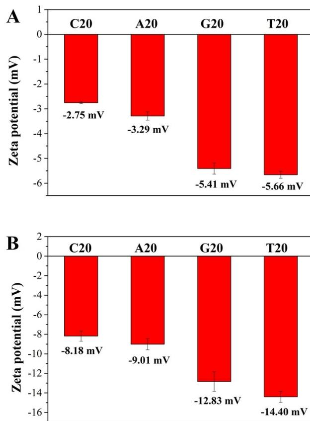
**Figure S5.** Zeta potential of 20-mer DNA homopolymer-modified MIL-53(Fe) (A) and the four types of homopolymers (B) at pH 4.0. [ssDNAs] = 200 nM.
