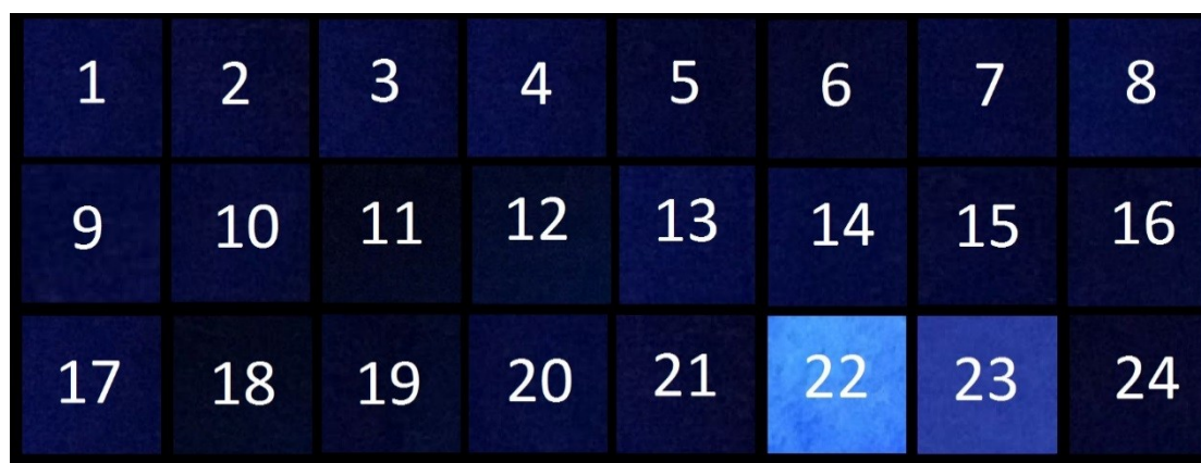
Figure S13. Fluorescence changes in test paper (under a 365 nm UV lamp) with probe BT-AC upon addition of some representative analytes (1. BT-AC ; 2. buffer; 3. Pro; 4. Asp; 5. Try; 6. Arg; 7. Tyr; 8. His; 9. Glu; 10. Lys; 11. Thr, 12. glucose; 13. K + ; 14. Ca 2+ ; 15. Na + ; 16. Mg 2+ ; 17. Zn 2+ ; 18. Fe 3+ ; 19. Cu 2+ ; 20. H 2 O 2 ; 21. NaHS; 22. Cys; 23. Hcy; 24. GSH).
