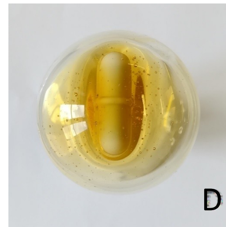
Fig S24: Picture of dissolved MCC in BMIMLev : 25 °C, 2 wt% (A); 40 °C, 7 wt% (B); 60 °C, 16 wt% (C); 80°C, 22 wt%(D); 100 °C, 24 wt%(E)
