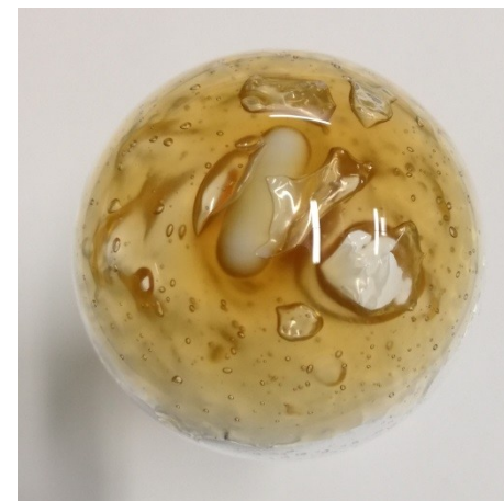
Fig S26: Picture of under vacuum undissolved MCC in BMIMLev (100 °C, 34.5 wt%)
