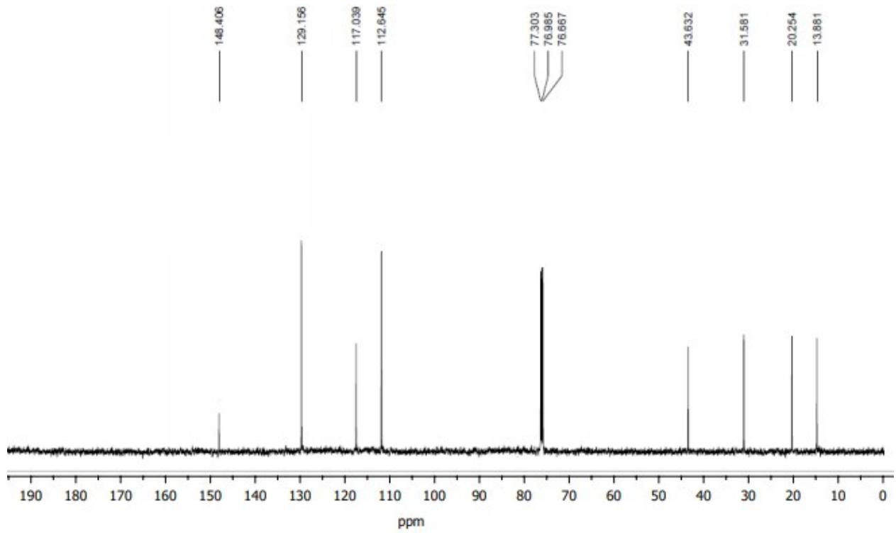
**Figure 24:**  $^{13}\text{C}$  NMR (100 MHz,  $\text{CDCl}_3$ ) of *N*-butylaniline (**16a**)
