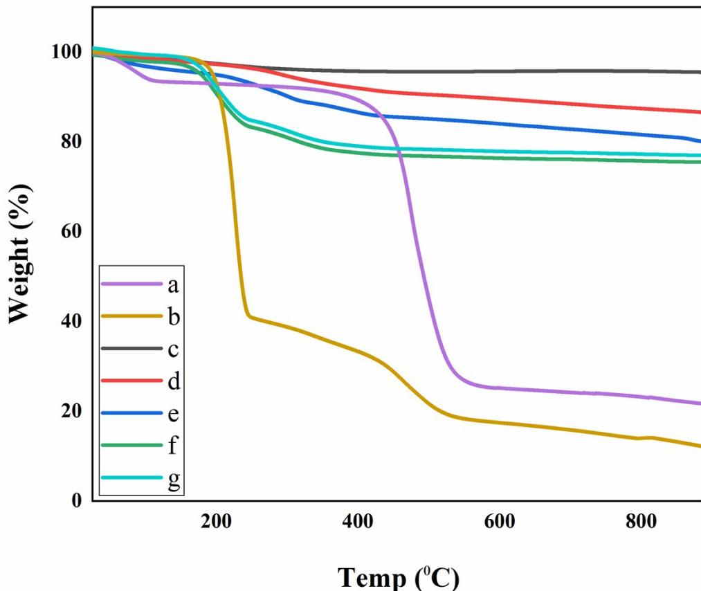
**Fig. S8.** TGA thermograms of NH<sub>2</sub>-MIL53(Al)(I) (a), AMCA-MIL53(Al)(II) (b), Fe<sub>3</sub>O<sub>4</sub> NPs (c), Fe<sub>3</sub>O<sub>4</sub>@AMCA-MIL53(Al)(III) NPs (d), Fe<sub>3</sub>O<sub>4</sub>@AMCA-MIL53(Al)-Ethephon(IV) (e) and Fe<sub>3</sub>O<sub>4</sub>@ AMCA-MIL53(Al)-NH<sub>2</sub>-Co<sup>II</sup> NPs(VI) (f) and the 7<sup>th</sup> reused Fe<sub>3</sub>O<sub>4</sub>@ AMCA-MIL53(Al)-NH<sub>2</sub>-Co<sup>II</sup> NPs(VI) (g) from the C-N cross coupling reaction (g).
