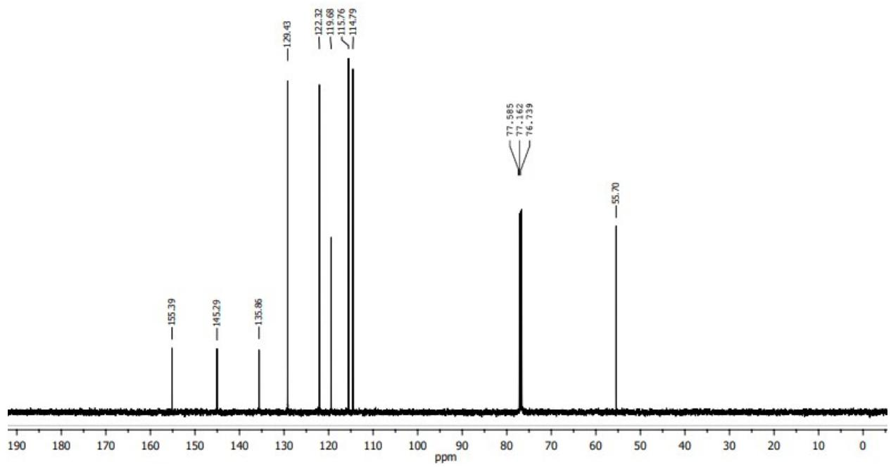
**Figure 16:**  $^{13}\text{C}$  NMR (100 MHz,  $\text{CDCl}_3$ ) of 4-Methoxy-*N*-phenylaniline (**10a**)
