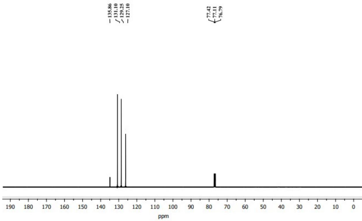
**Figure 38:** <sup>13</sup>C NMR (100 MHz, CDCl<sub>3</sub>) of Diphenyl sulfide (**1b**)
