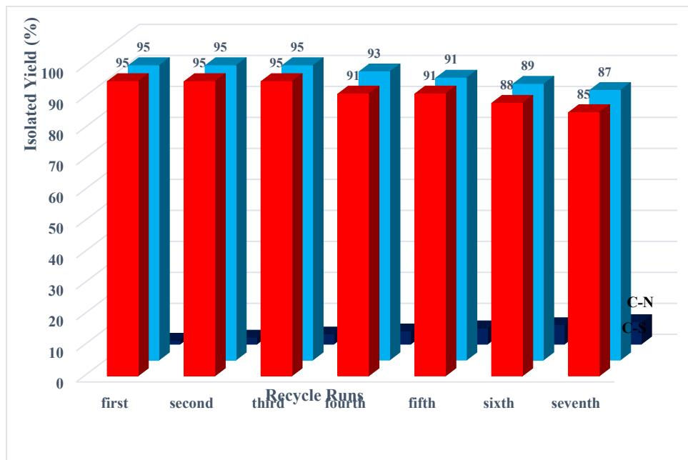
**Fig. S12.** C-N and C-S cross coupling reactions in the presence of the reused  $\text{Fe}_3\text{O}_4@\text{AMCA}$ -MIL53(Al)-NH<sub>2</sub>-Co<sup>II</sup> NPs(**VI**).
