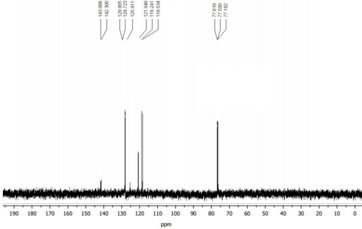
**Figure 12:** <sup>13</sup>C NMR (100 MHz, CDCl<sub>3</sub>) of 4-Chloro-N-phenylaniline (**7a**)
