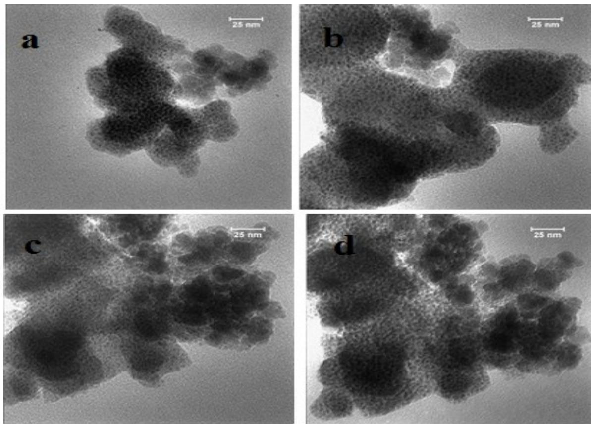
**Fig. S3.** TEM images of the fresh  $\text{Fe}_3\text{O}_4@\text{AMCA-MIL53}(\text{Al})-\text{NH}_2\text{-Co}^{\text{II}}$  NPs (**VI**) (a and b) and the 7<sup>th</sup> reused  $\text{Fe}_3\text{O}_4@\text{AMCA-MIL53}(\text{Al})-\text{NH}_2\text{-Co}^{\text{II}}$  NPs (**VI**) from the C-N cross coupling reaction (c) and the 7<sup>th</sup> reused  $\text{Fe}_3\text{O}_4@\text{AMCA-MIL53}(\text{Al})-\text{NH}_2\text{-Co}^{\text{II}}$  NPs (**VI**) from the C-S cross coupling reaction (d).
