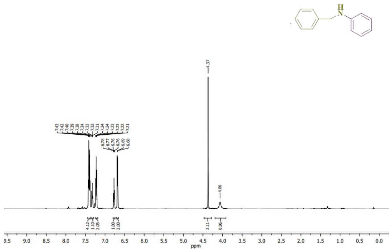
**Figure 21:**  $^1\text{H}$  NMR (300 MHz,  $\text{CDCl}_3$ ) of *N*-benzylniline (13a)
