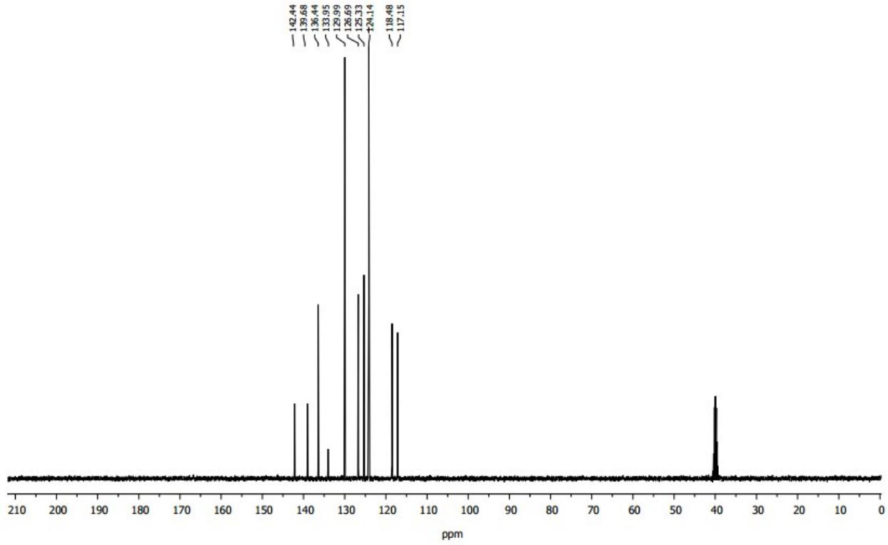
**Figure 26:**  $^{13}\text{C}$  NMR (100 MHz, DMSO- $d_6$ ) of 2-Nitro-N-phenylaniline (**19a**)
