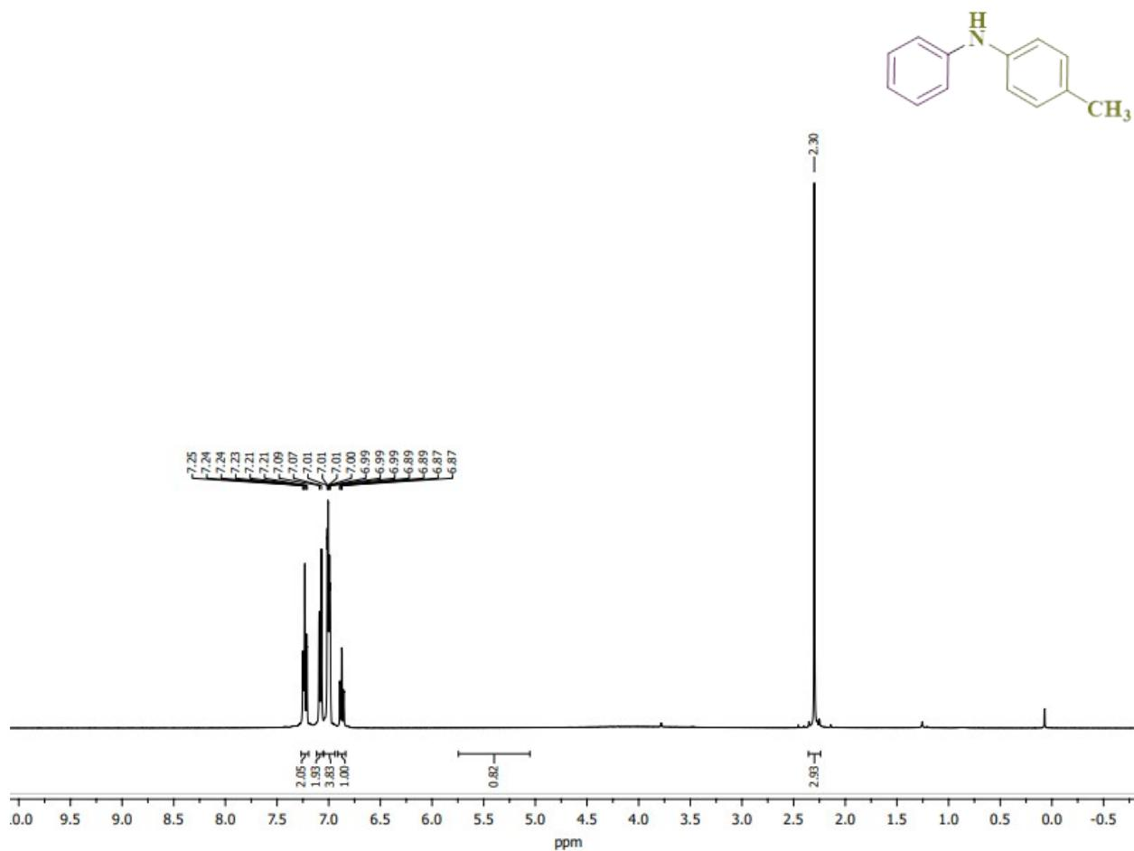
**Figure 17:** <sup>1</sup>H NMR (300 MHz, CDCl<sub>3</sub>) of 4-Methyl-N-phenylaniline (**11a**)
