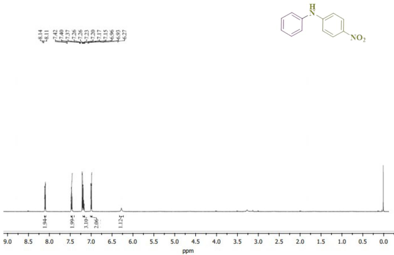
**Figure 13:** <sup>1</sup>H NMR (300 MHz, CDCl<sub>3</sub>) of 4-Nitro-*N*-phenylaniline (**8a**)
