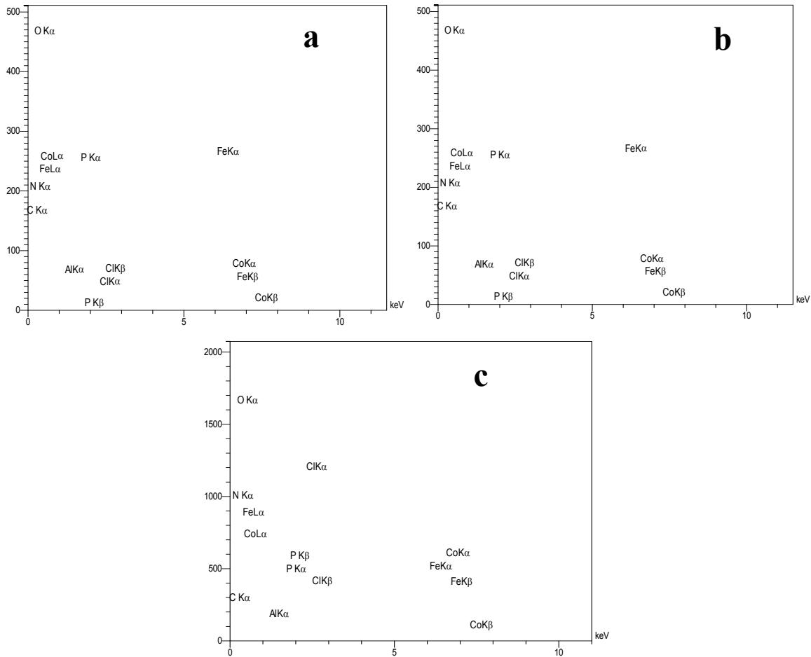
**Fig. S6.** EDX spectrum of  $\text{Fe}_3\text{O}_4@\text{AMCA-MIL53}(\text{Al})-\text{NH}_2\text{-Co}^{\text{II}}$  NPs (**VI**) (a), the 7<sup>th</sup> reused  $\text{Fe}_3\text{O}_4@\text{AMCA-MIL53}(\text{Al})-\text{NH}_2\text{-Co}^{\text{II}}$  NPs (**VI**) from the C-N cross coupling reaction (b) and the 7<sup>th</sup> reused  $\text{Fe}_3\text{O}_4@\text{AMCA-MIL53}(\text{Al})-\text{NH}_2\text{-Co}^{\text{II}}$  NPs (**VI**) from the C-S cross coupling reaction (c).
