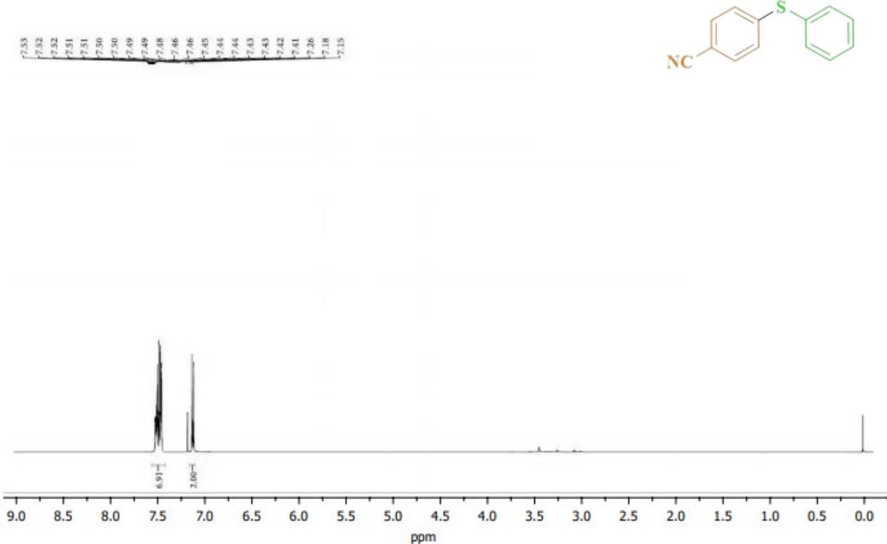
**Figure 48:** <sup>1</sup>H NMR (400 MHz, CDCl<sub>3</sub>) of Phenyl (*p*-cyanophenyl) sulfide (**14b**)
