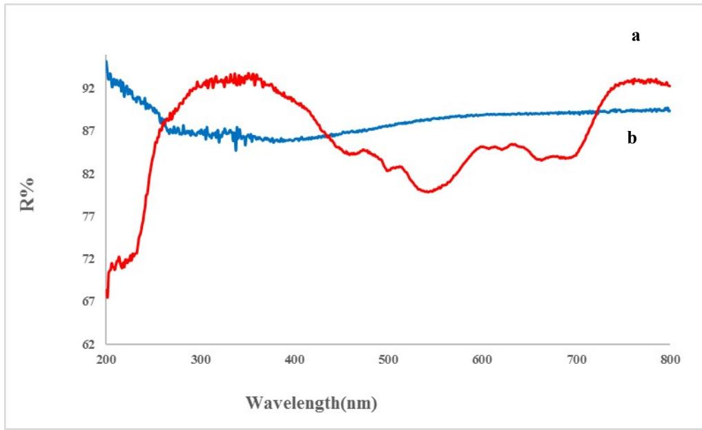
**Fig. S11.** UV-vis. DRS spectra of cobalt(II) chloride (a) and  $\text{Fe}_3\text{O}_4@\text{AMCA}-\text{MIL53}(\text{Al})-\text{NH}_2$ - $\text{Co}^{\text{II}}$  NPs(**VI**) (b).
