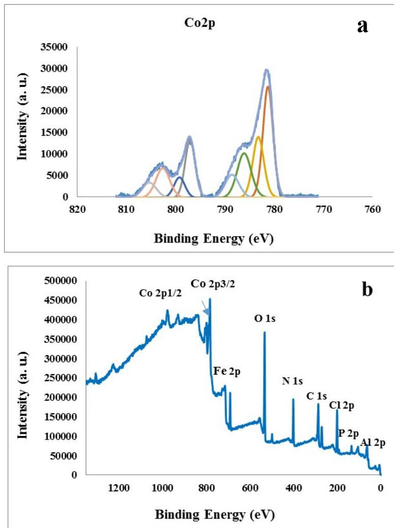
**Fig. S9.** XPS spectra (a) and XPS elemental survey (b) of  $\text{Fe}_3\text{O}_4@\text{AMCA-MIL53(Al)-NH}_2\text{-Co}^{\text{II}}$  NPs (**VI**).
