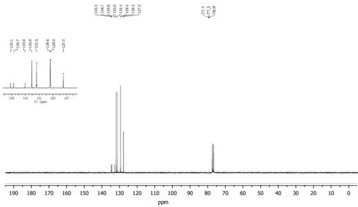
**Figure 41:** <sup>13</sup>C NMR (75 MHz, CDCl<sub>3</sub>) of Phenyl (*p*-chlorophenyl) sulfide (**2b**)
