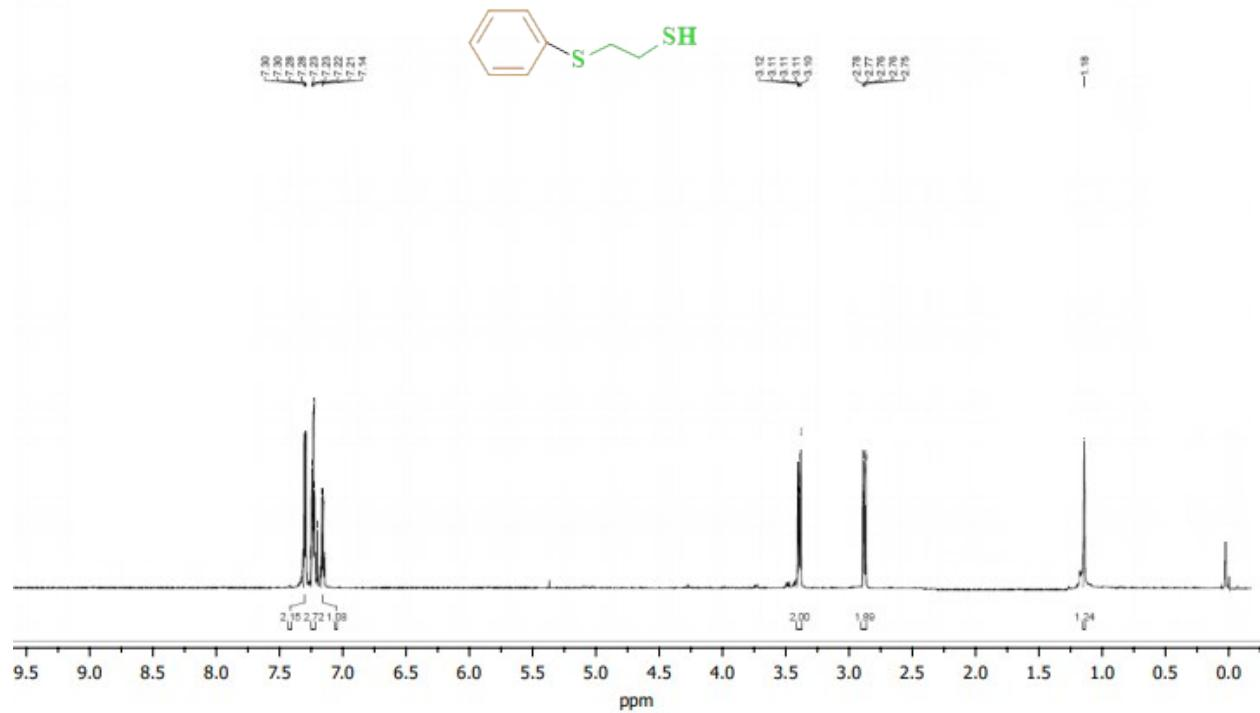
**Figure 44:**  $^1\text{H}$  NMR (400 MHz,  $\text{CDCl}_3$ ) of 2-(Phenylthio) ethane-1-thiol (**6b**)
