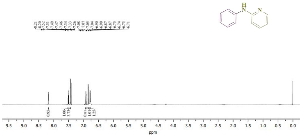
**Figure 19:** <sup>1</sup>H NMR (300 MHz, CDCl<sub>3</sub>) of *N*-phenylpyridin-2-amine (12a)
