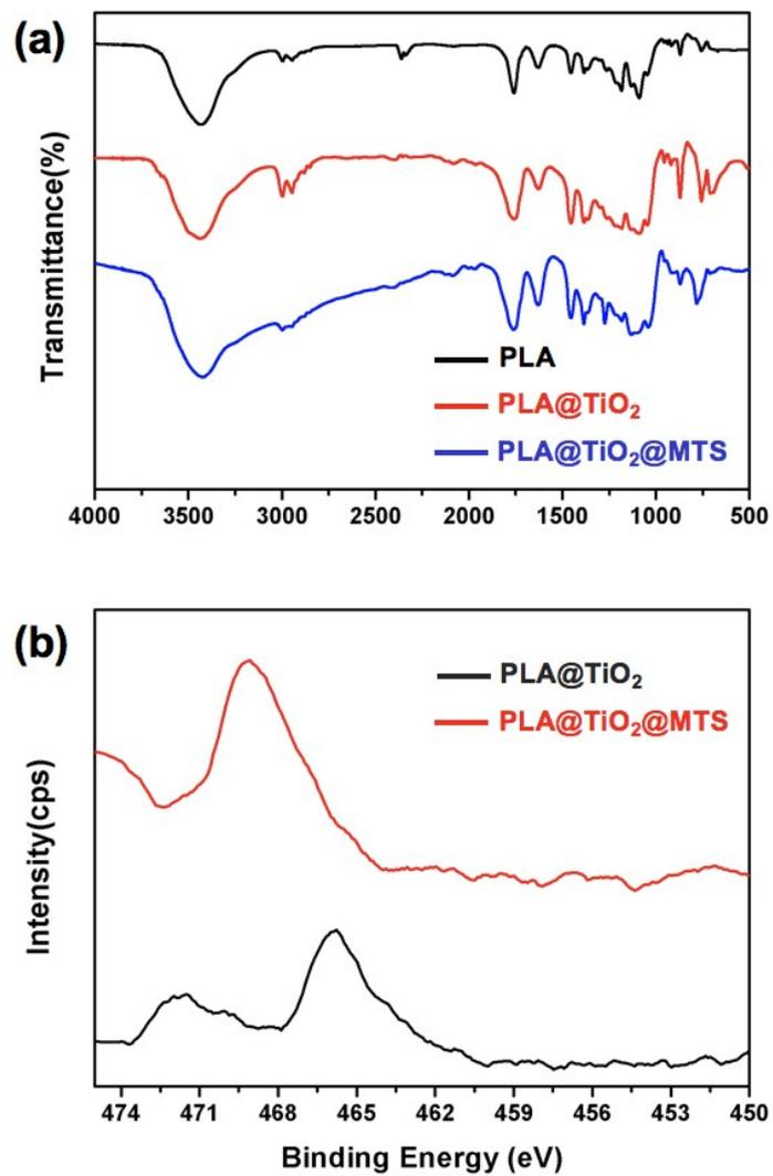
**Fig. S1** (a) FT-IR spectra of PLA, PLA@TiO<sub>2</sub>, PLA@TiO<sub>2</sub>@MTS, and (b) X-ray photoelectron spectroscopy (XPS) of titanium.
