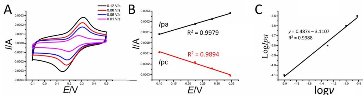
**Fig. S1** (A) CV curves of SP-DNA/cMWCNTs/GCE at different scan rates in the range of 0.01 ~ 0.12 V/s. (B) linear calibration plots for the peak current versus square root of scan rate. (C) linear calibration plots for the logarithm of peak current versus logarithm of scan rate.
