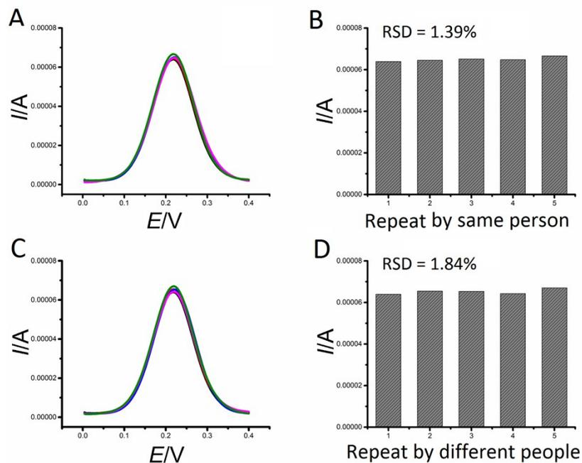
**Fig. S4** (A) The DPV curves of developed WtDNA LCR-based electrochemical biosensor obtained by the same person, (B) histogram of DPV peak current in (A). (C) The DPV curves of developed WtDNA LCR-based electrochemical biosensor obtained by five persons, (D) histogram of DPV peak current in (C).
